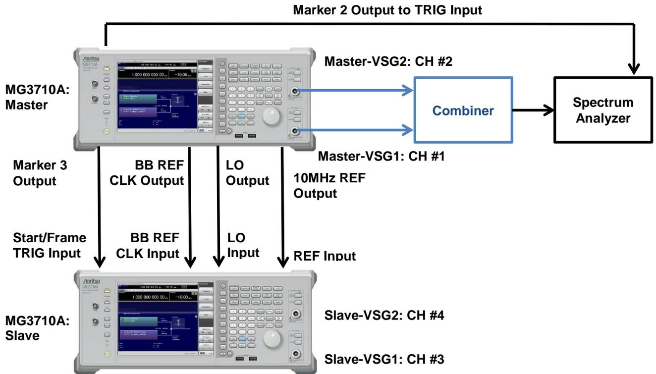
Figure 12. 4x4 MIMO configuration
