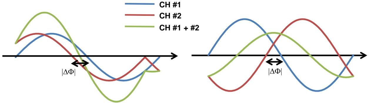
Figure 5. Waveforms of two signals to be synchronized; phase error  $|\Delta\Phi|$  (left) and phase error  $180^\circ + |\Delta\Phi|$  (right)
