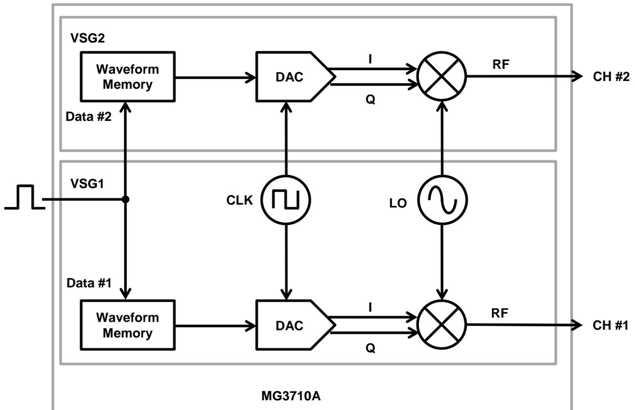
Figure 4. Channel synchronization using MG3710A SG
