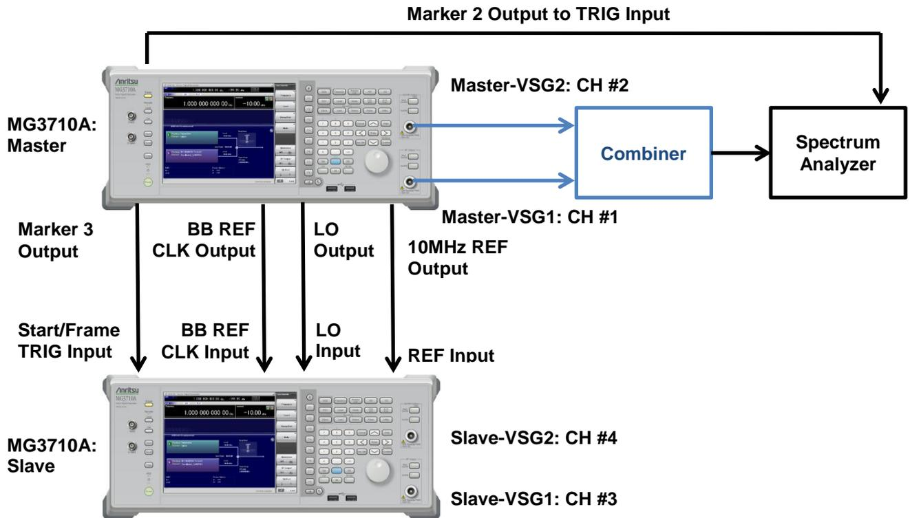
Figure 12. 4x4 MIMO configuration
