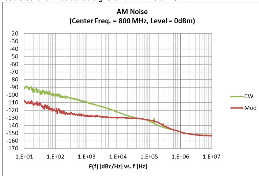
Figure 22. MG3710A AM Noise Characteristics (Measurement Value)
