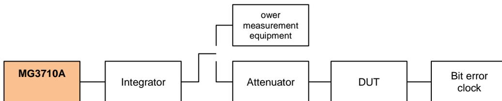
Figure 26. Adjacent Channel Selectivity Measurement System (using MG3710A)
