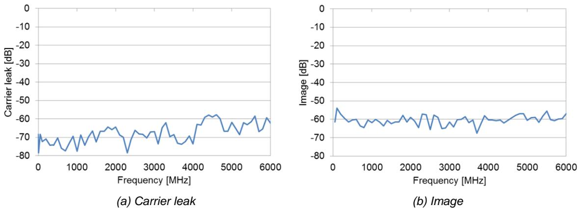
Figure 11. MG3710A Carrier Leak and Image Frequency Characteristics (after I/Q Calibration) (Measured Values)
