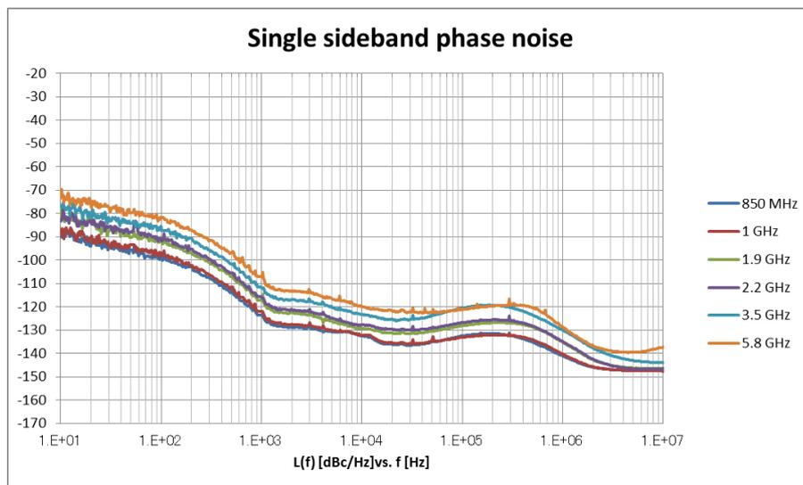
Figure 19. MG3710A Phase Noise Characteristics (Phase Noise Opt.: <200 kHz) (Measurement Value)
