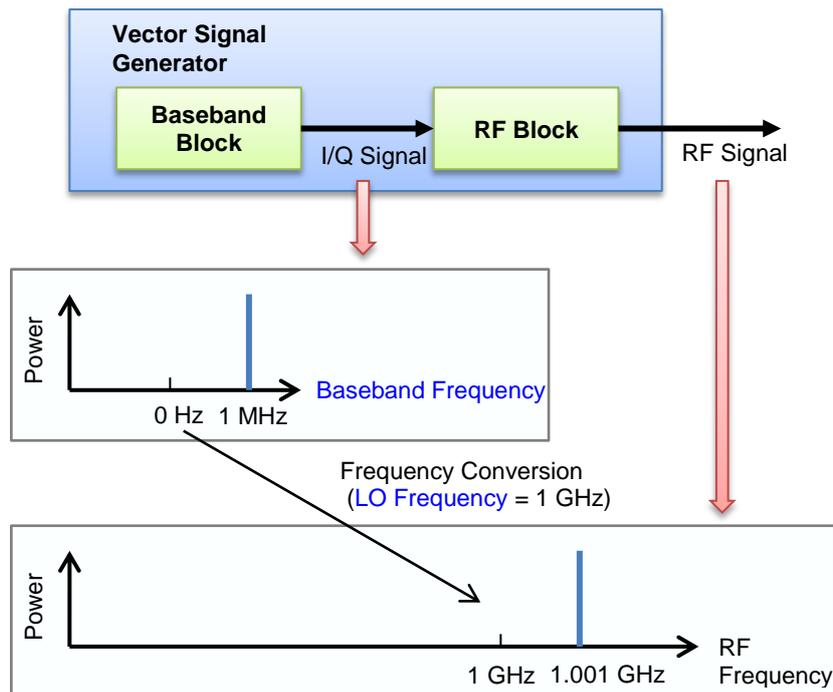
Figure 1. Baseband Frequency and LO Frequency
