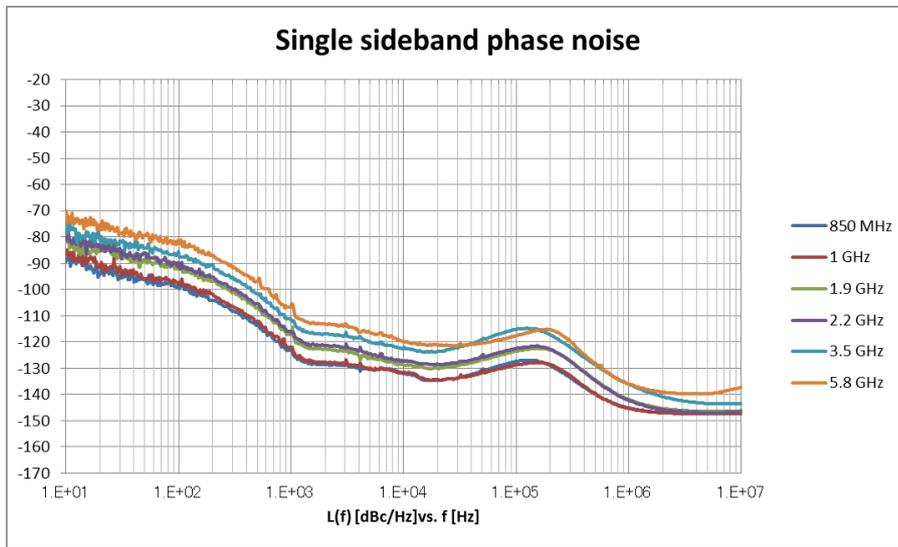
Figure 20. MG3710A Phase Noise Characteristics (Phase Noise Opt.: >300 kHz) (Measurement Value)
