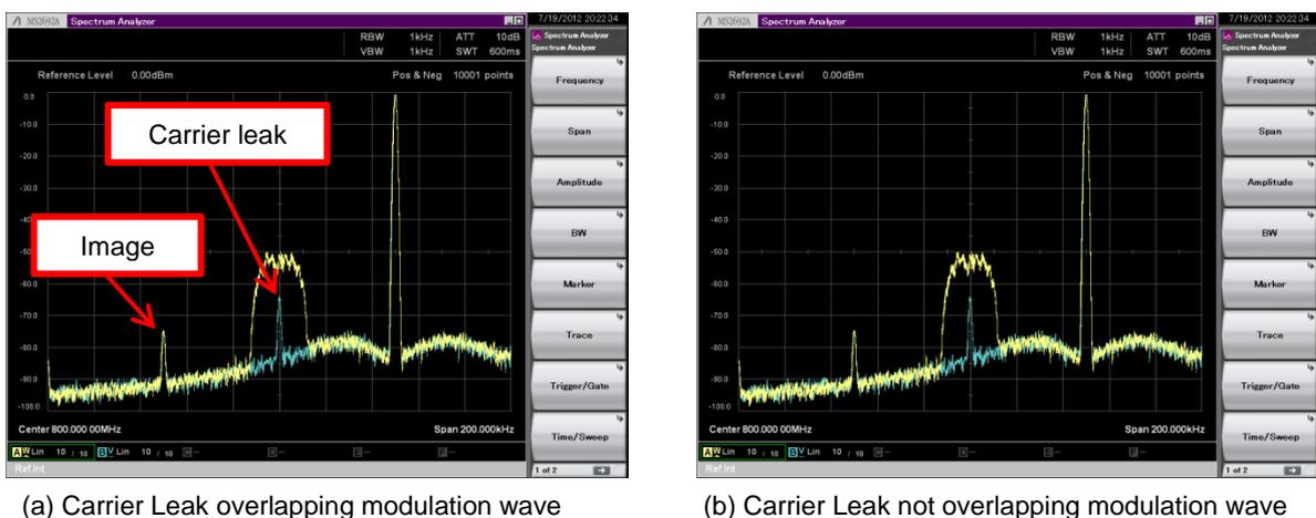
Figure 12. Preventing Carrier Leak and Image
