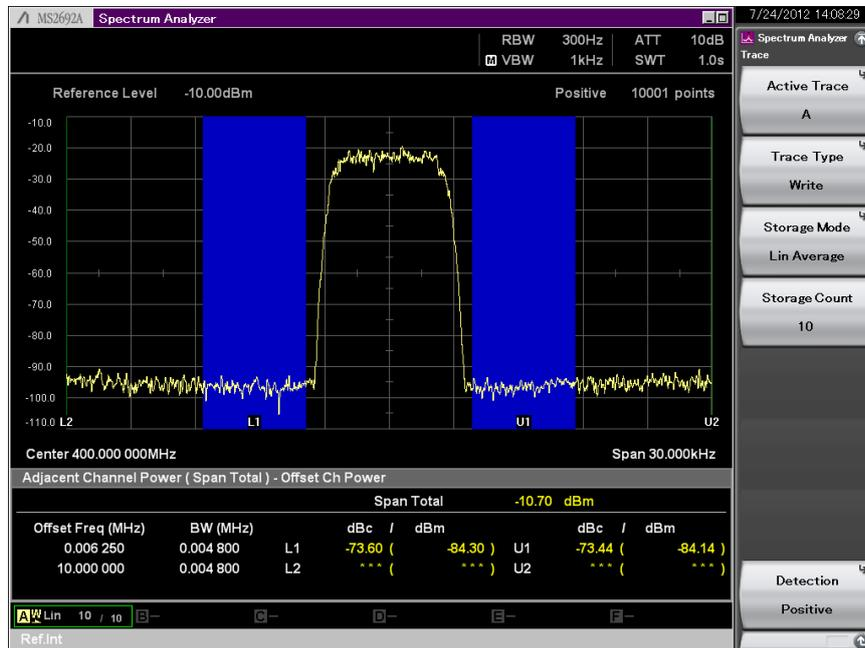
Figure 27. ARIB-STD T61 ACLR (Measurement Value)
