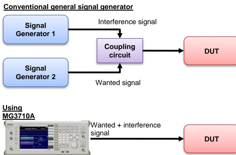
Figure 4. Example of Rx Characteristics Test Setup
