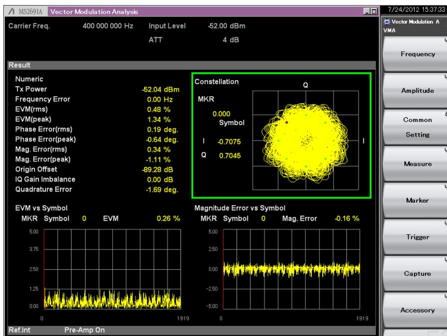
Figure 28. ARIB-STD T61 Modulation Accuracy (Measurement Value)
