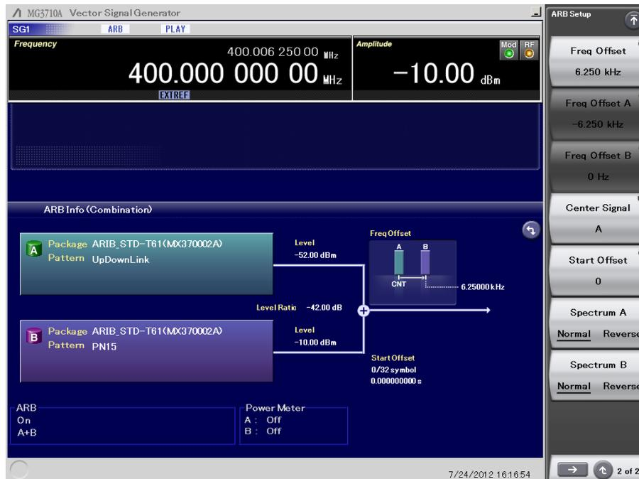
Figure 31. Example of MG3710A Setting Screen
