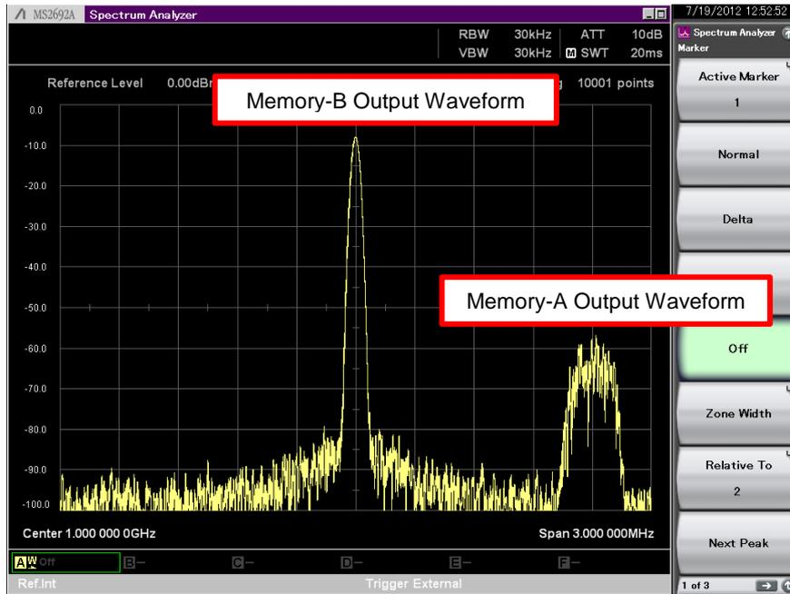
Figure 3. Example of Two-signal Combine Function Spectrum
