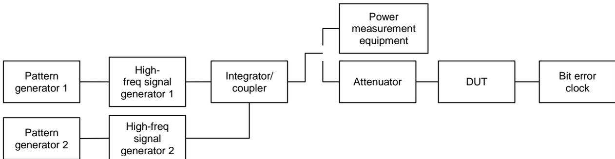
Figure 25. Adjacent Channel Selectivity Measurement System
