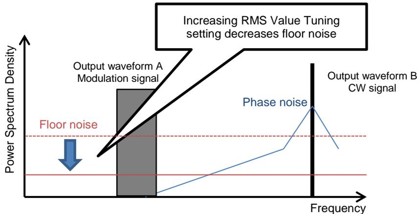
Figure 24. Floor Noise Optimization by RMS Value Tuning
