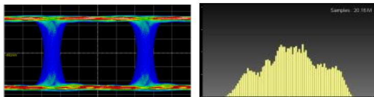
Figure 4-7. Typical Waveform including BUJ, and Jitter Histogram
