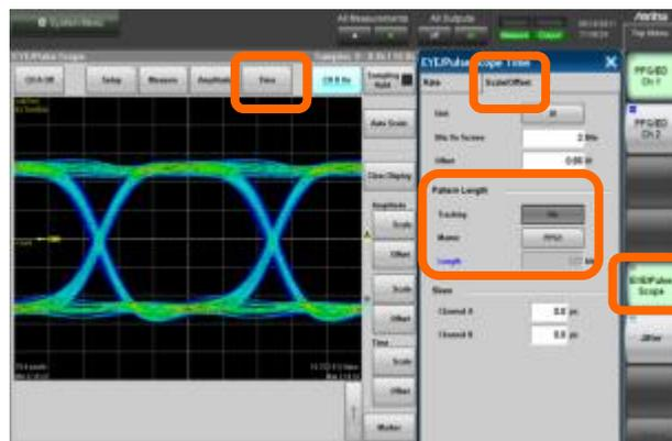
Figure 5-6. Pattern Length Tracking
