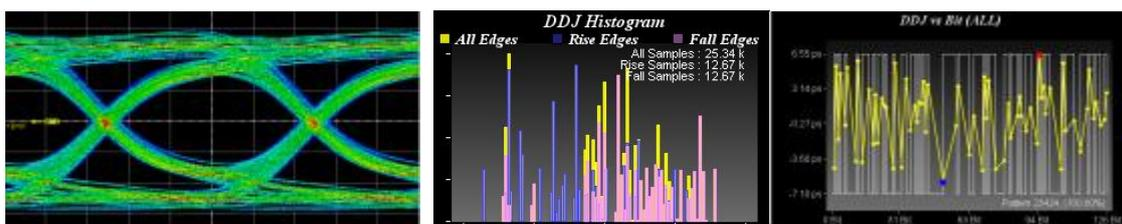
Figure 4-9. Typical Waveform including DDJ, ISI, and DDPW, and Jitter Histogram
