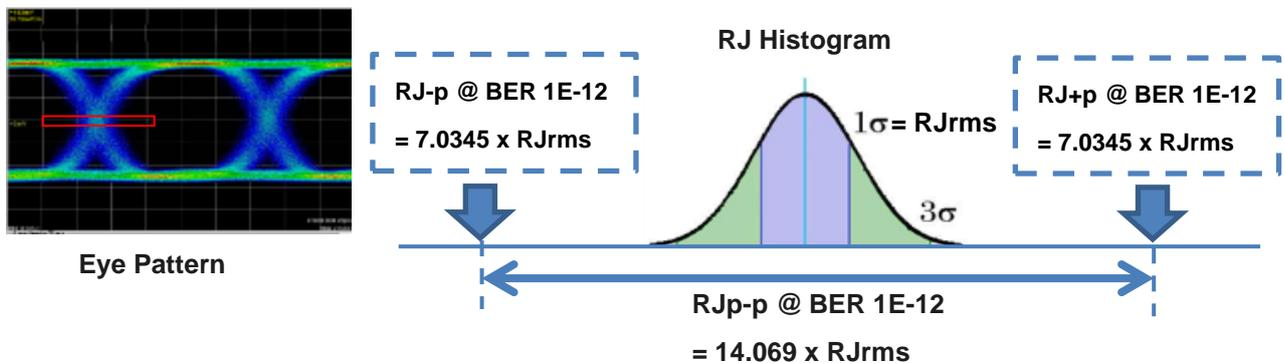
Figure 4-3. Typical Waveform including RJ, and RJ Histogram
