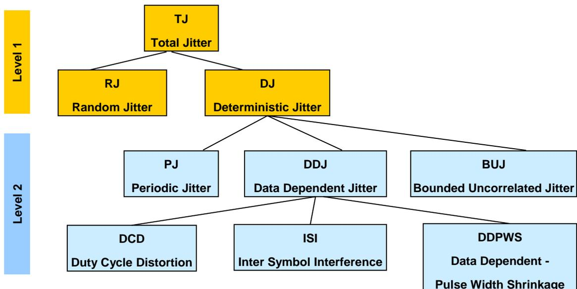
Figure 4-1. Jitter Components and Analysis Level
