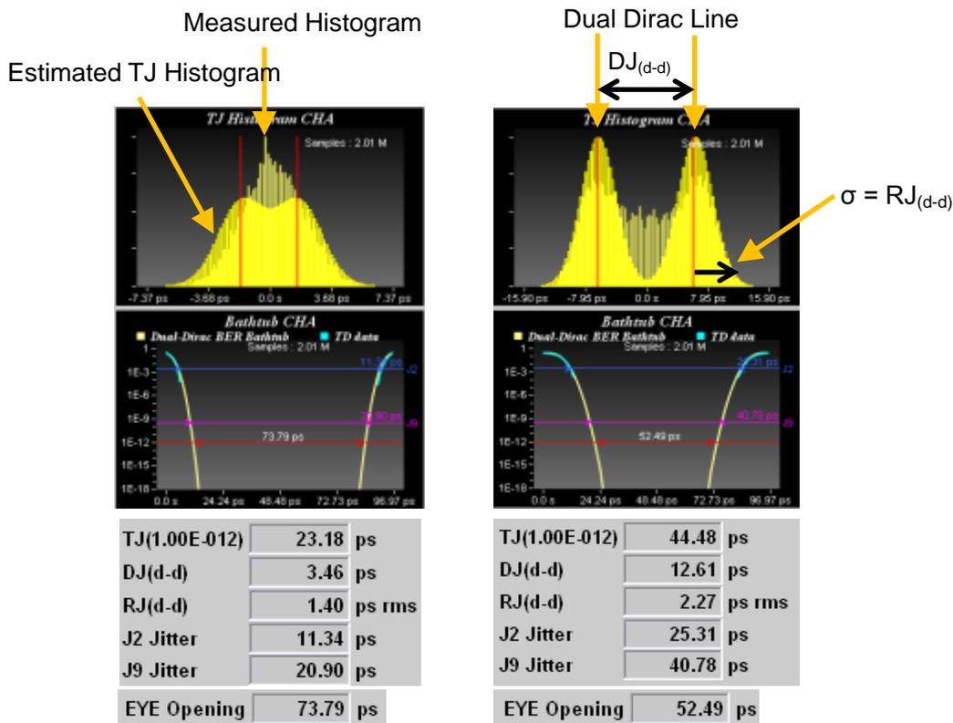
Figure 5-5. Example of Analysis Result using Histogram Method (left: DUT\_A, right: DUT\_B)
