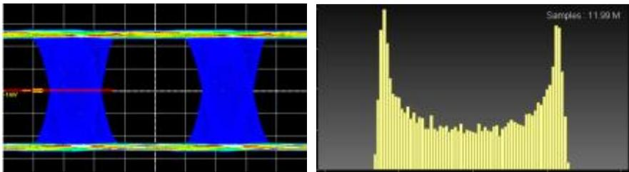
Figure 4-5. Typical Waveform with SJ, and Jitter Histogram
