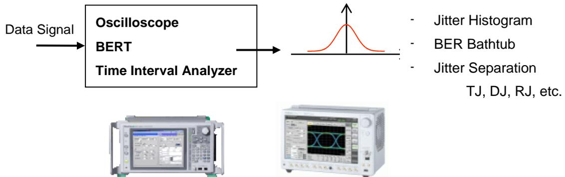
Figure 3-3. Jitter Measurement Instruments for Datacoms/Computing Fields
