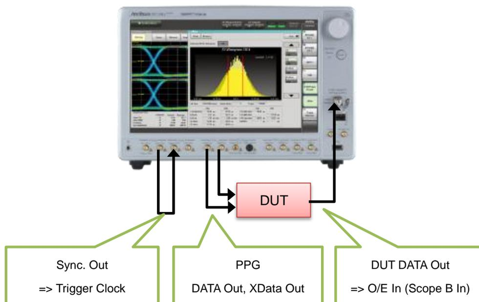
Figure 5-1. Measurement System using MP2100A
