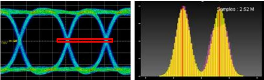
Figure 4-6. Typical Waveform with HPJ, and Jitter Histogram
