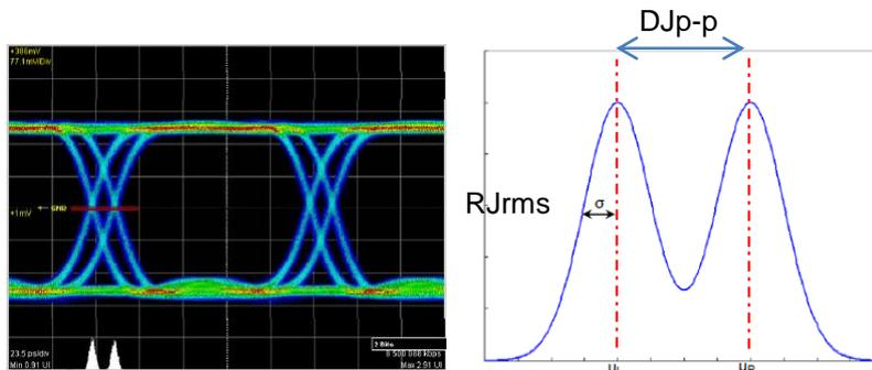
Figure 4-4. Typical DJ Waveform, and Histogram
