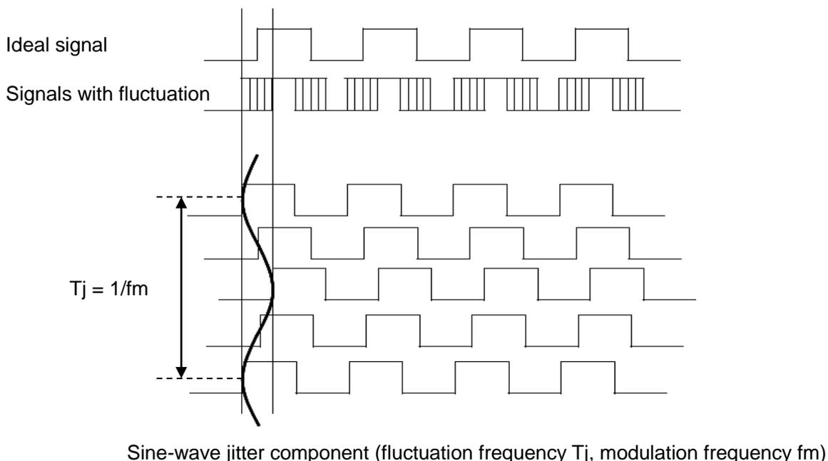
Figure 2-1. Jitter Modulation Frequency
