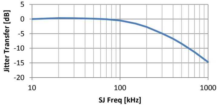
Figure 3-4. Example of Jitter Transfer Measurement Result
