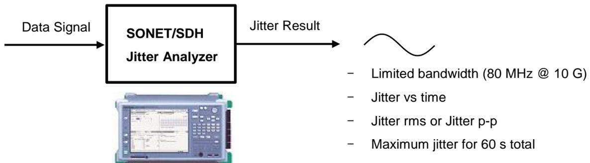
Figure 3-2. SONET/SDH Jitter Measurement Instrument (MP1590B)
