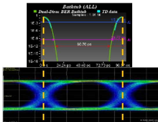
Figure 4-2. Relationship between BER Bathtub Curve and Eye Pattern
