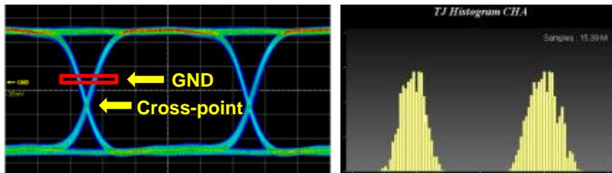
Figure 4-10. Typical Waveform including DCD and Jitter Histogram
