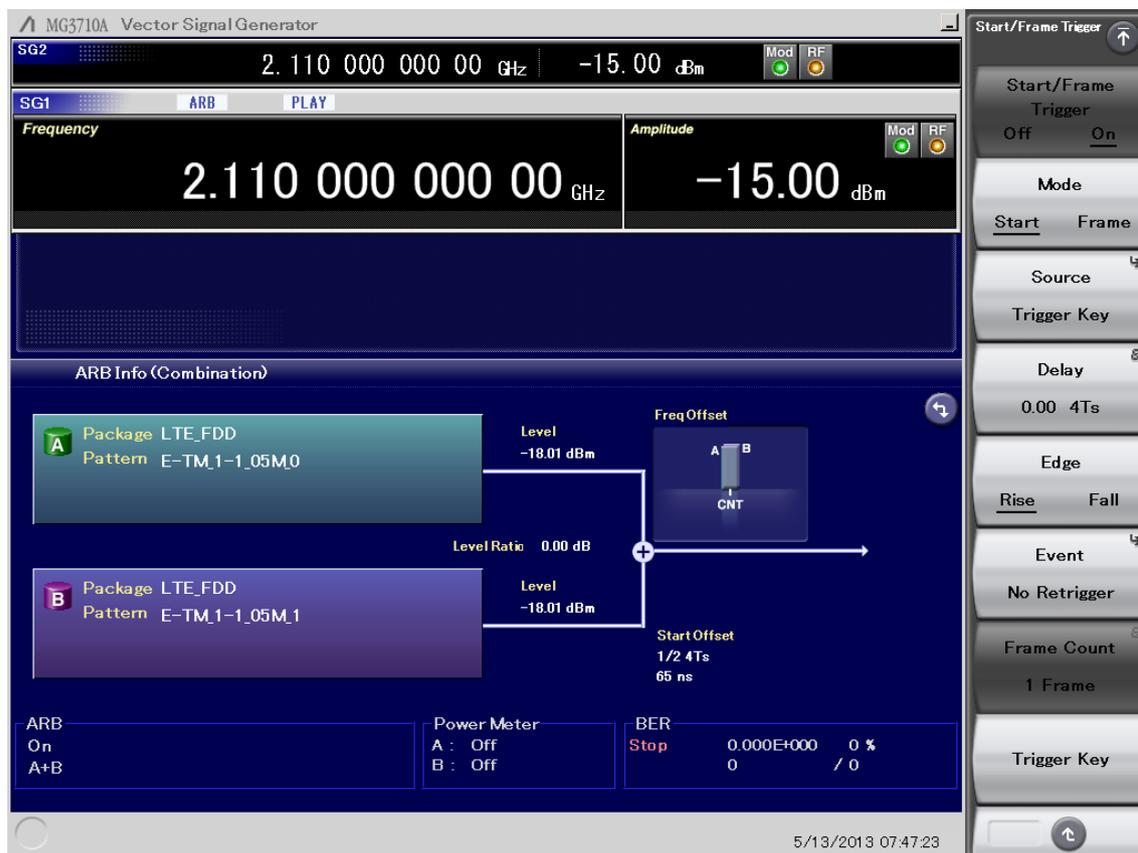
Fig. 5. Example of Four Antenna Signal Outputs (SG1 Setting Display)
