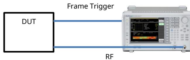
Fig. A-1 Transmit On/Off Power Measurement Setup
