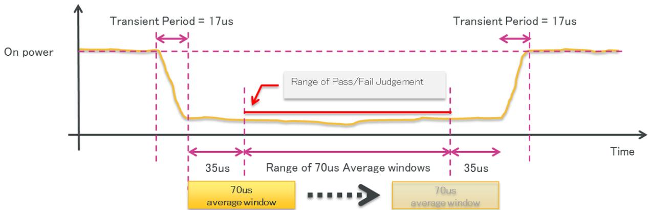
**Fig. 2 Average Power During Transmit On Period (Horizontal Red Line)**
