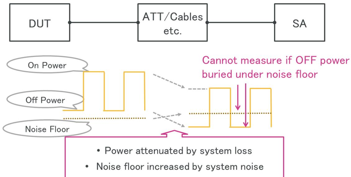
Fig. 4 General Model of Transmit On/Off Power Measurement
