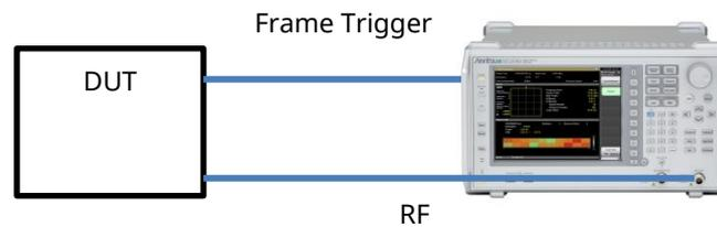
Fig. A-1 Transmit On/Off Power Measurement Setup
