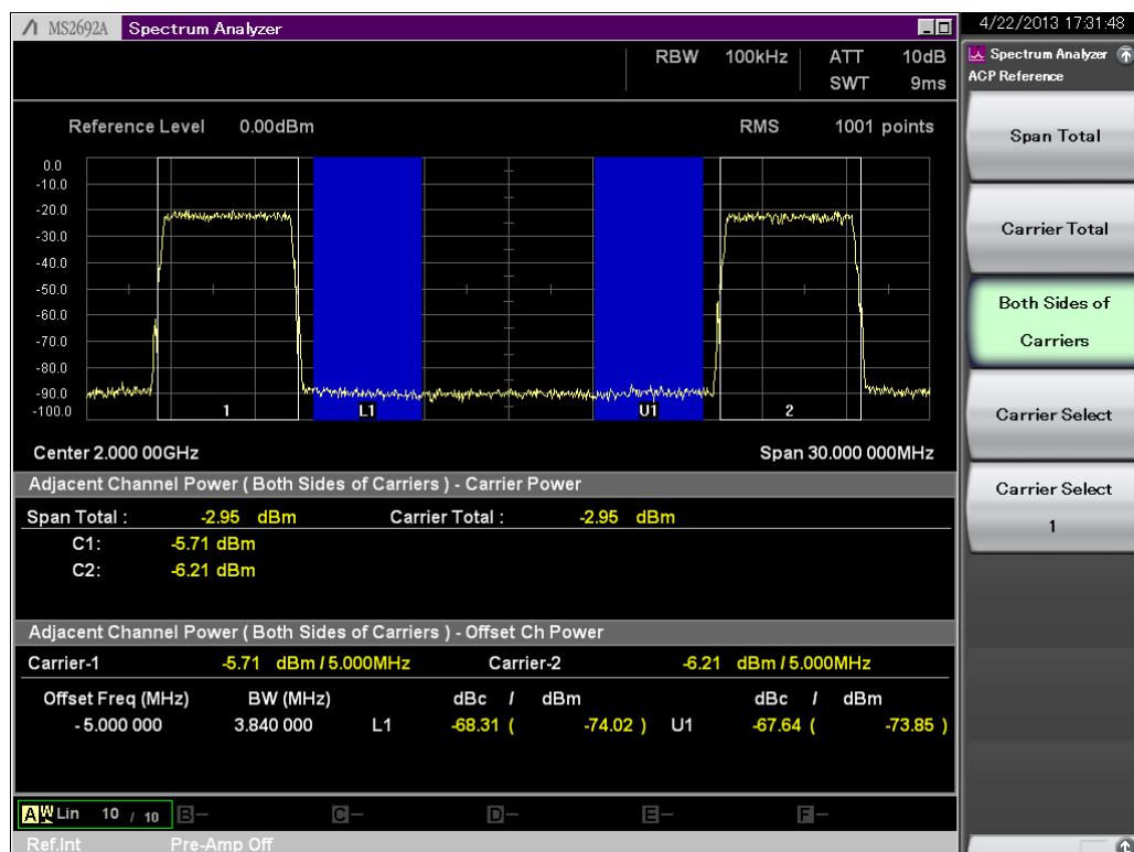
Fig. 15. Non-contiguous spectrum ACLR (sub-block gap) measurement example
