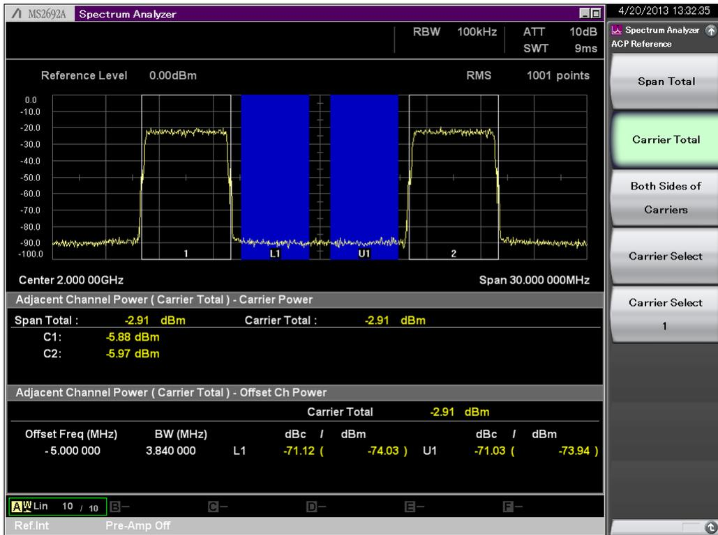
Fig. 13. Non-contiguous spectrum CACLR (sub-block gap) measurement example
