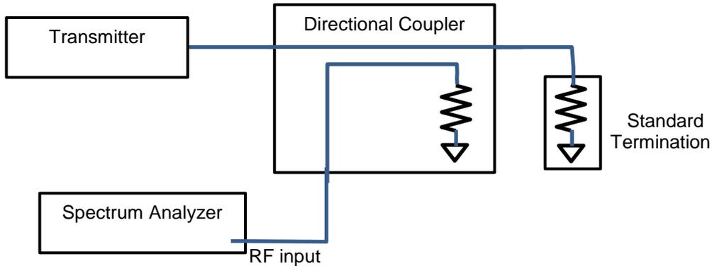
Fig.3. Reference Level Setting Connections
