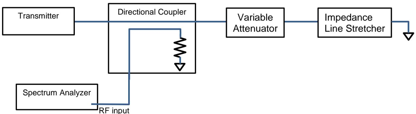
Fig.4. Spurious Generation Frequency Check Setup
