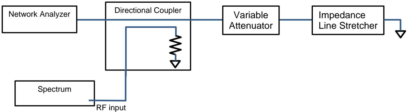
Fig.1. Variable Attenuator Adjustment Setup
