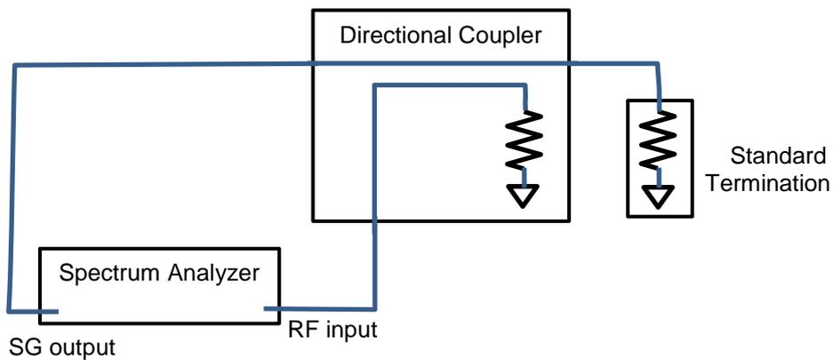
Fig.6. Spurious Level Measurement Setup
