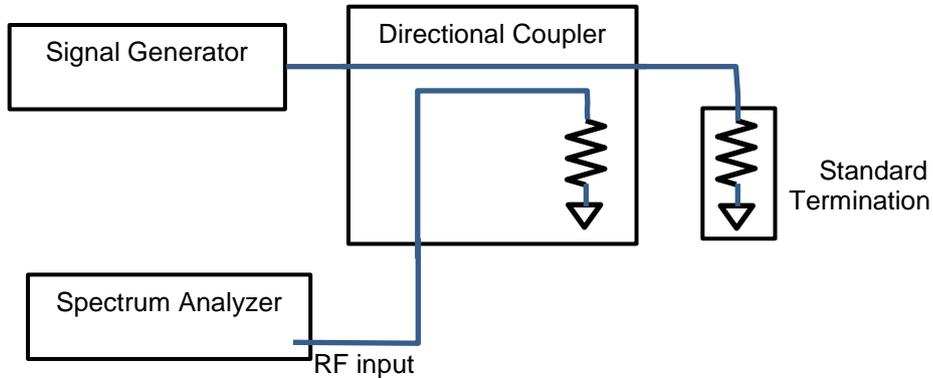
Fig.5. Spurious Level Measurement Setup
