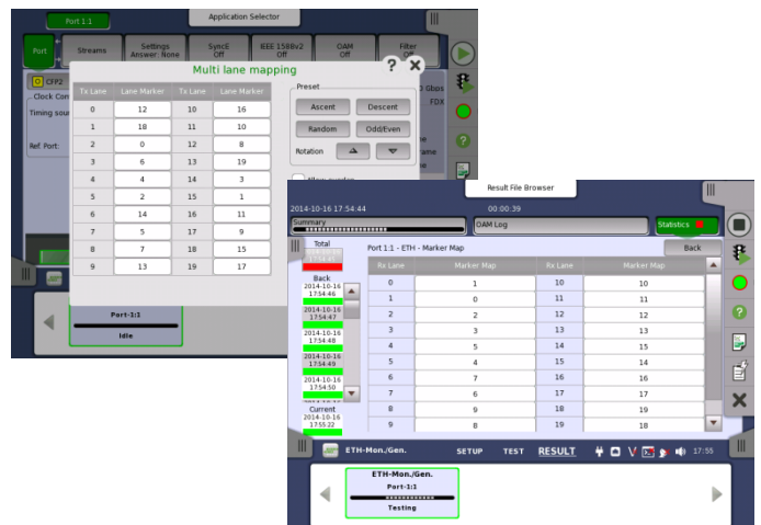
Fig. 3. Lane Mapping Switching and Monitoring
