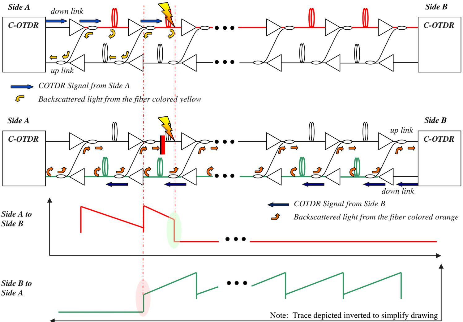
Fig 5; C-OTDR showing the repeater and break location
