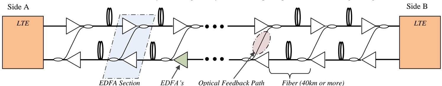
Fig 1; Major components of a Submarine System
