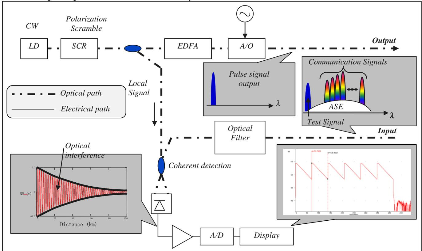
Fig 4; Basic internal working of a C-OTDR
