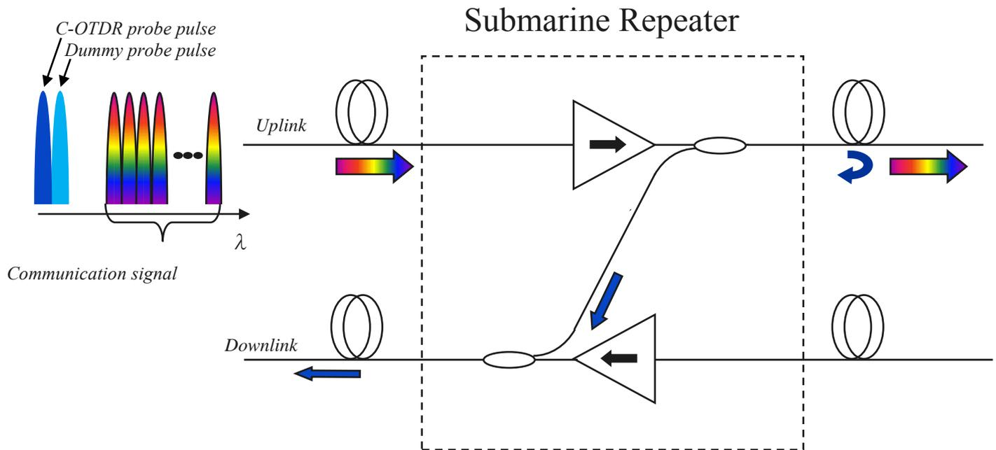
Fig 2; Submarine Repeater system showing C-OTDR return path.
