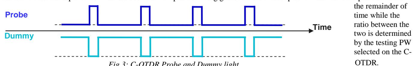
Fig 3; C-OTDR Probe and Dummy light
