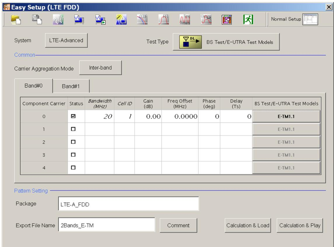
Fig. 3. IQproducer Settings (Inter-band Discontinuous 2 Carrier Aggregation)
