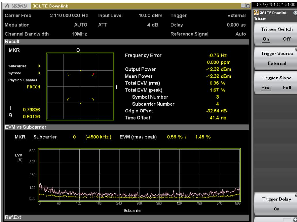
Fig. 7. CC#1 Measurement Results (SA#1)
