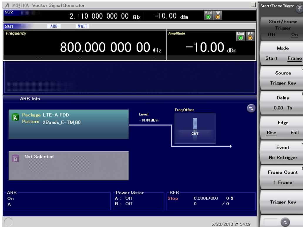
Fig. 4. MG3710A Vector Signal Generator Setting Example
