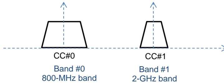
Fig. 1. Discontinuous 2 Carrier Aggregation between Bands
