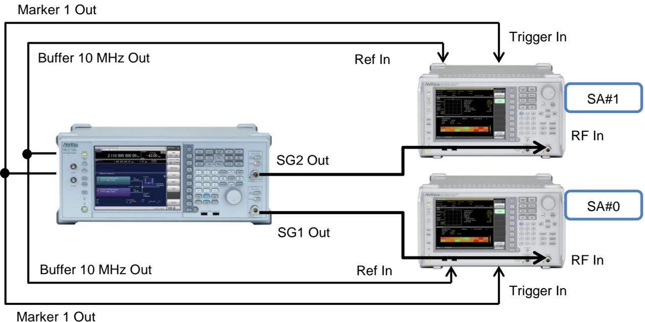
Fig. 2. Connection Setup (Inter-band Discontinuous 2 Carrier Aggregation)
