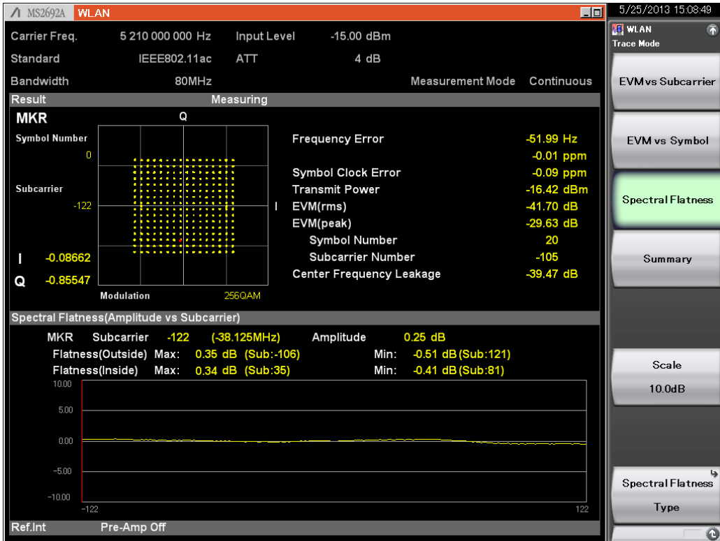
Fig. 3. Modulation Accuracy Measurement (80-MHz bandwidth)
