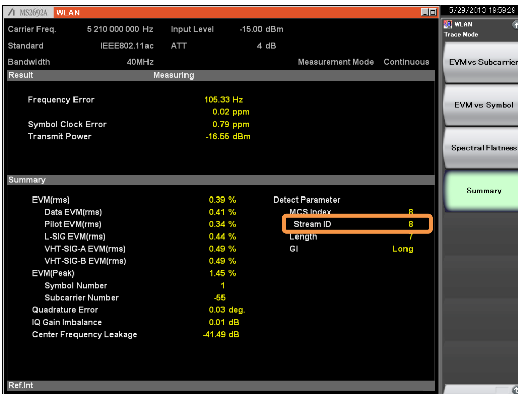
Fig. 15. Measurement Results for 8 Antenna Setup (Tx7)
