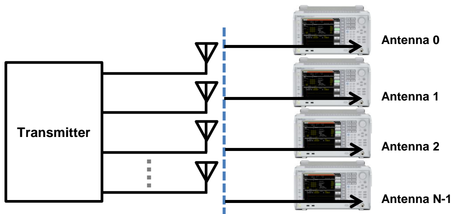
Fig. 14. MIMO Transmitter Test Setup
