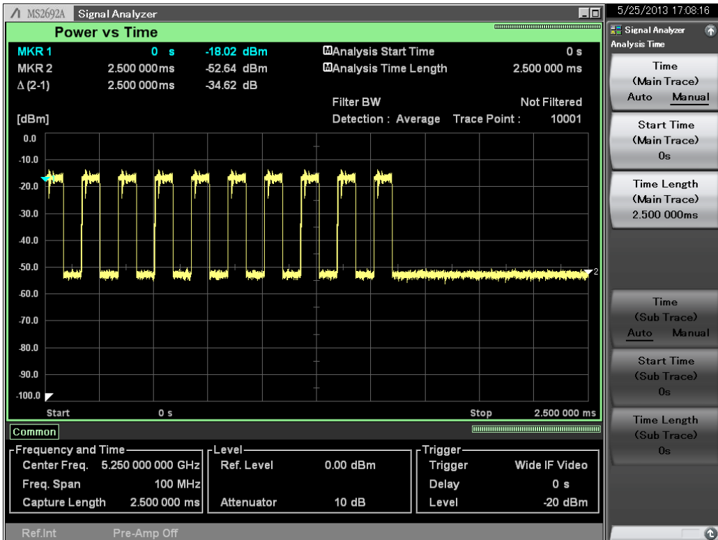
Fig. 18. Results when Sending Burst of 10 W-LAN Packets
