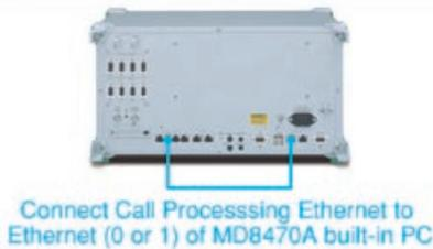
Connect Call Processing Ethernet to Ethernet (0 or 1) of MD8470A built-in PC
