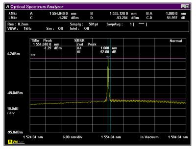
Measures optical transceivers with 0 dBm output, and 50 dB SMSR in <1 s\*2.
