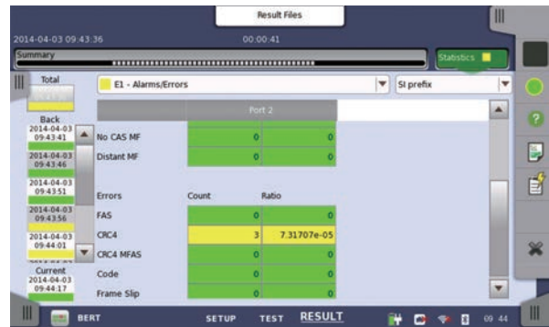
Color indications give an easy overview of GO/NO-GO results
