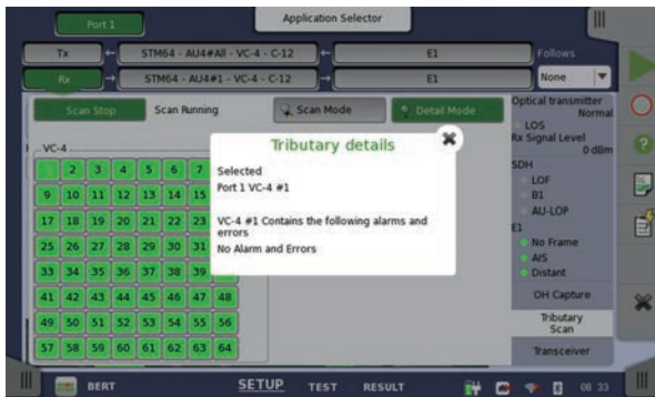
The SDH/SONET tributary scan gives a quick overview of the status of the monitored line
