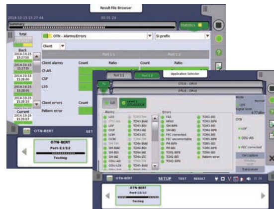
Comprehensive OTN Alarm/Error monitoring and BER testing
