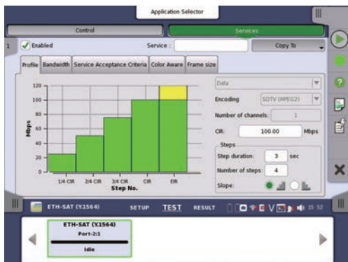
Simple and intuitive configuration of Y.1564 test
