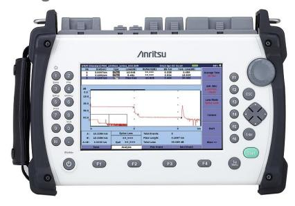
According to increasing the data traffic, the PON network is developing continuously and it has been progressing toward 10G-PON/10GE-PON network. Therefore, the loss and the ORL measurement of OTDRs will be more important not only 1310/1550 nm testing but also 1490 nm testing, as used for the downstream. In addition, The CWDM is deployed for secure networks and the OTDR measurement is also required for this network.
