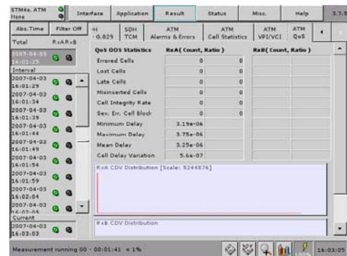
Fig. 8 QoS parameters measured by the CMA 3000.
