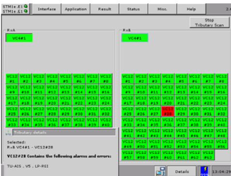
Fig.4: The trouble scan feature gives you a quick overview of the tributaries of the monitored line.
