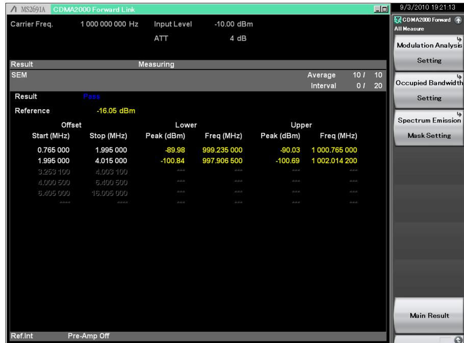
Figure 3.10.2-1 SEM Result Detail Screen
