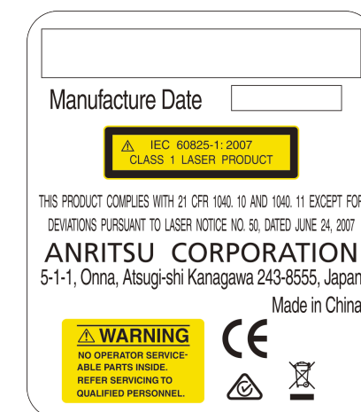
Figure 2 CMA5 Series Light Source Laser Safety Labels
