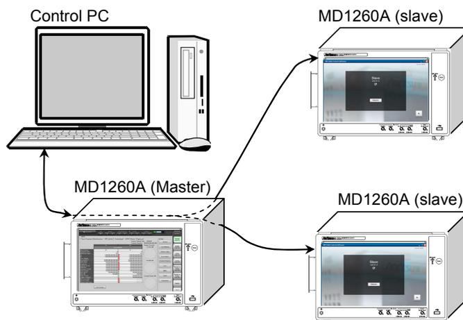
Figure 7.1-2 Remote Control of MD1260A Units by Multiport Function
