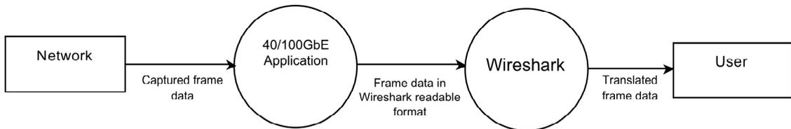
**Figure F.2-1 Data Flow at Tandem Operation**
