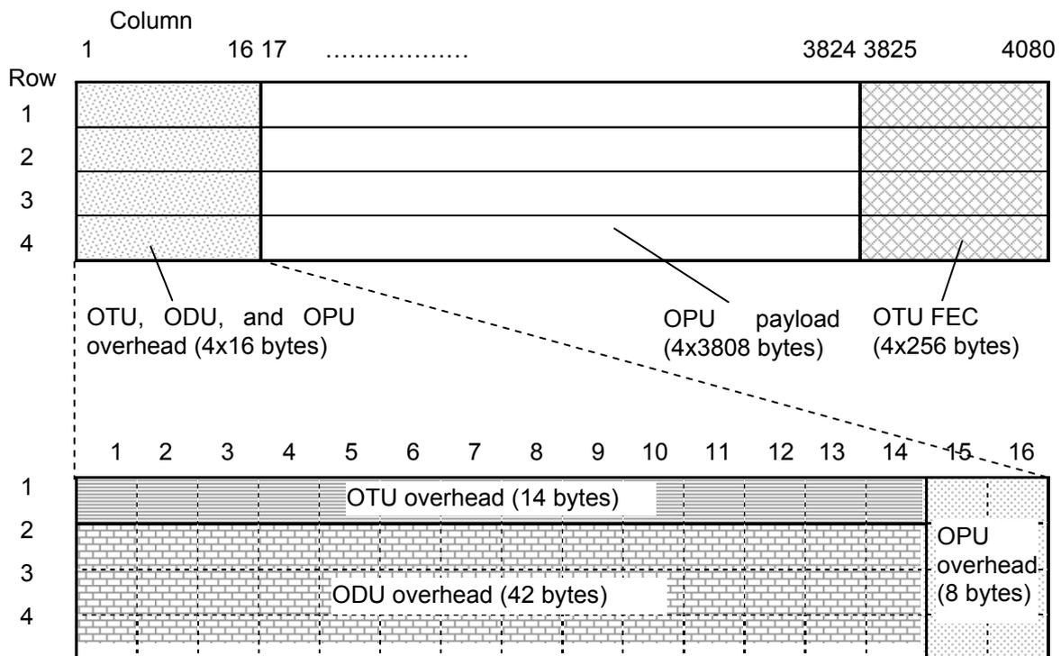
Figure 5.1-2 OTU Frame Format
