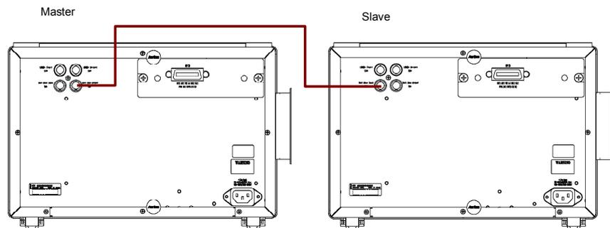
Figure 7.2.3-2 Coaxial Cable Connection
