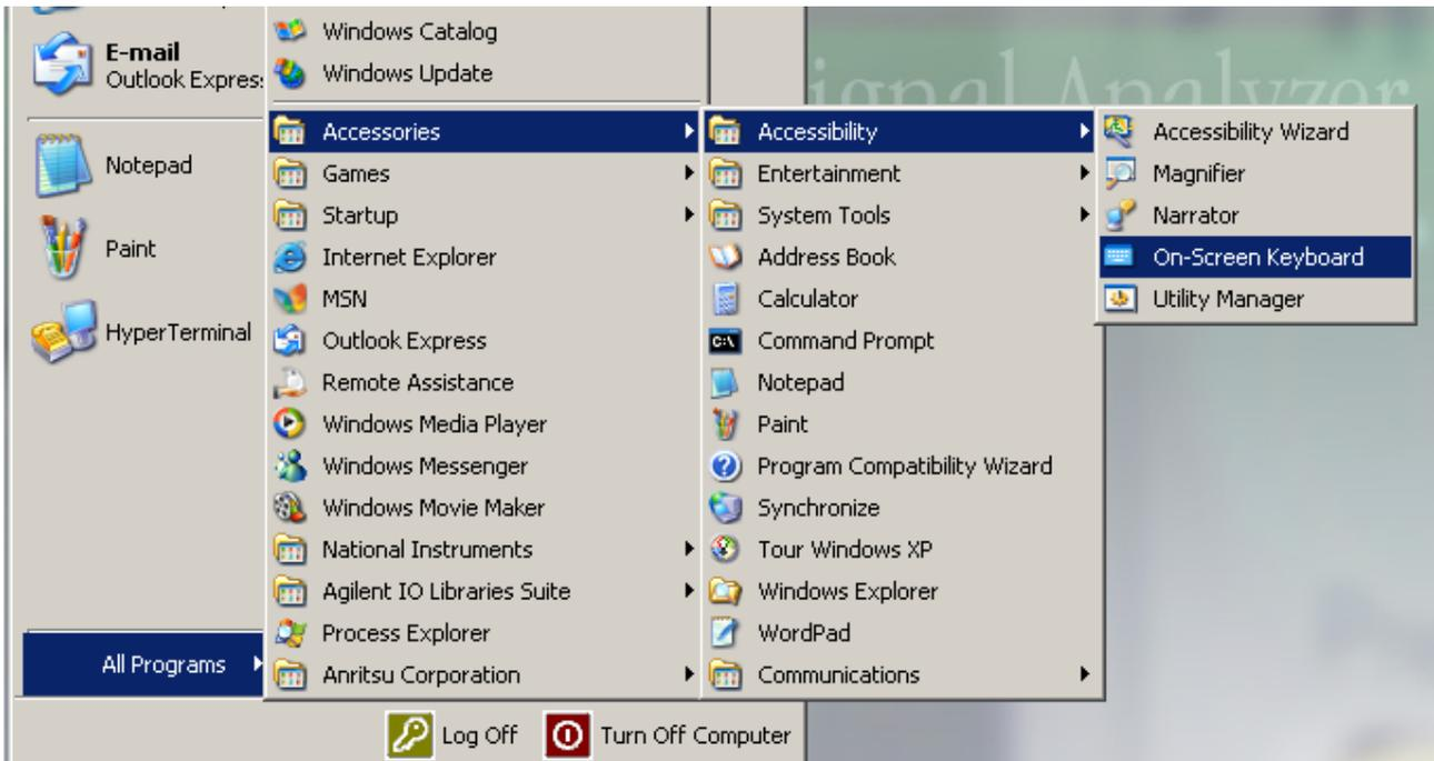
Figure 5.4.3-4 Starting Window Software Keyboard
