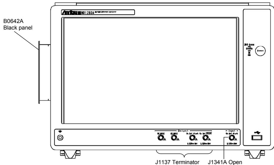
Figure 8.6-1 Installation Position of Accessories
