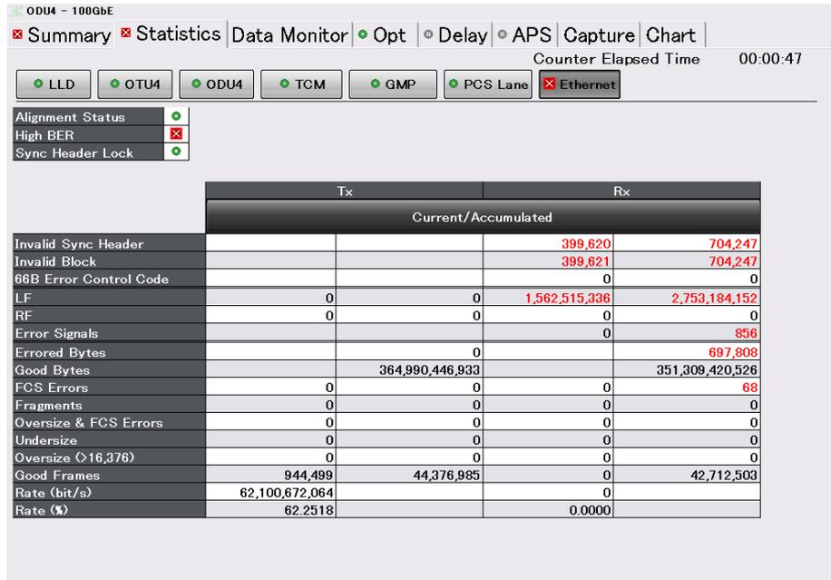
Figure 5.5.8-2 Statistics Tab for 100GbE (Ethernet)
