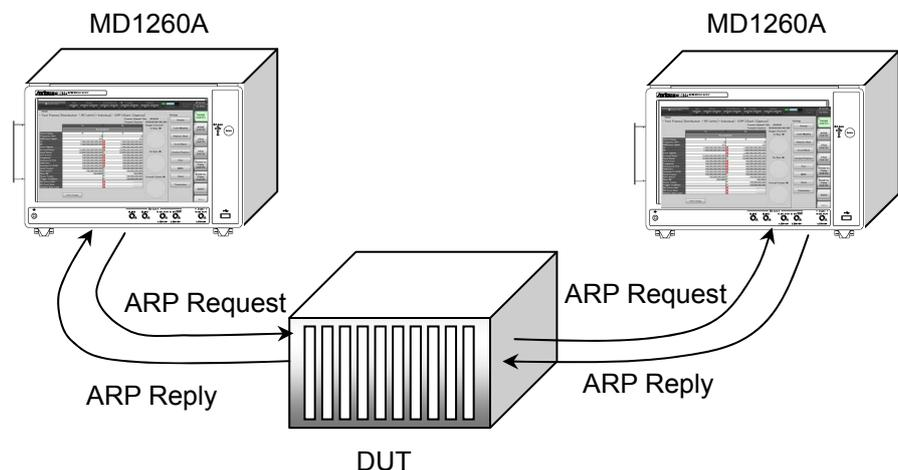
Figure 4.5.1-2 ARP Packet Communication Test Using Two MD1260As
