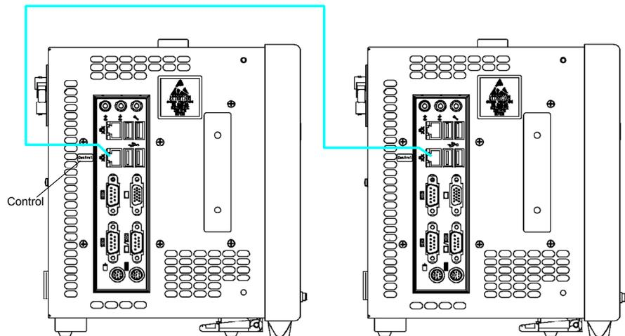
Figure 7.2.3-1 Ethernet Cable Connection
