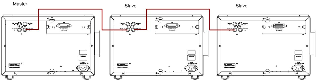
Figure 7.2.3-4 Coaxial Cable Connection between Multiple MD1260A Units
