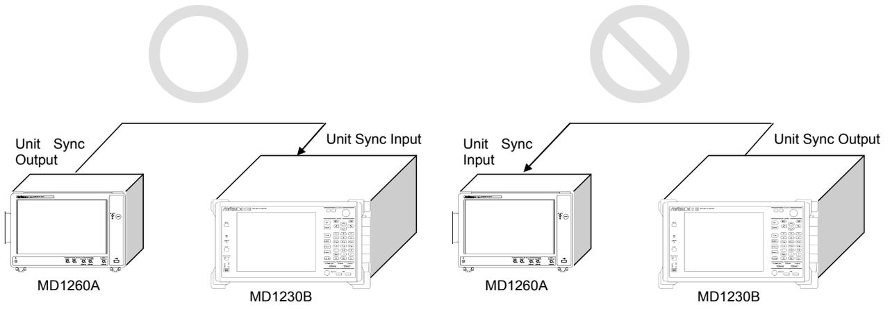
**Figure E.1-2 Direction of Synchronous Clock**
