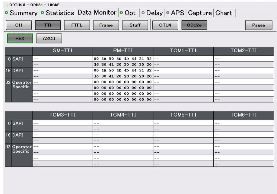
Figure 5.5.10-2 Data Monitor Tab (TTI)-HEX Display
