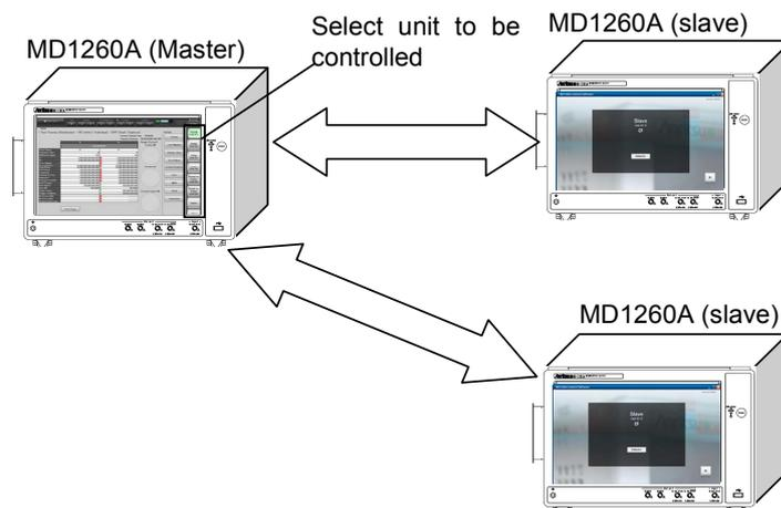
Figure 7.1-1 Example of Multiport Function Control
