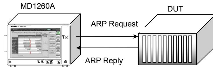
Figure 4.5.1-1 Checking Overlapping IP Addresses by Gratuitous ARP
