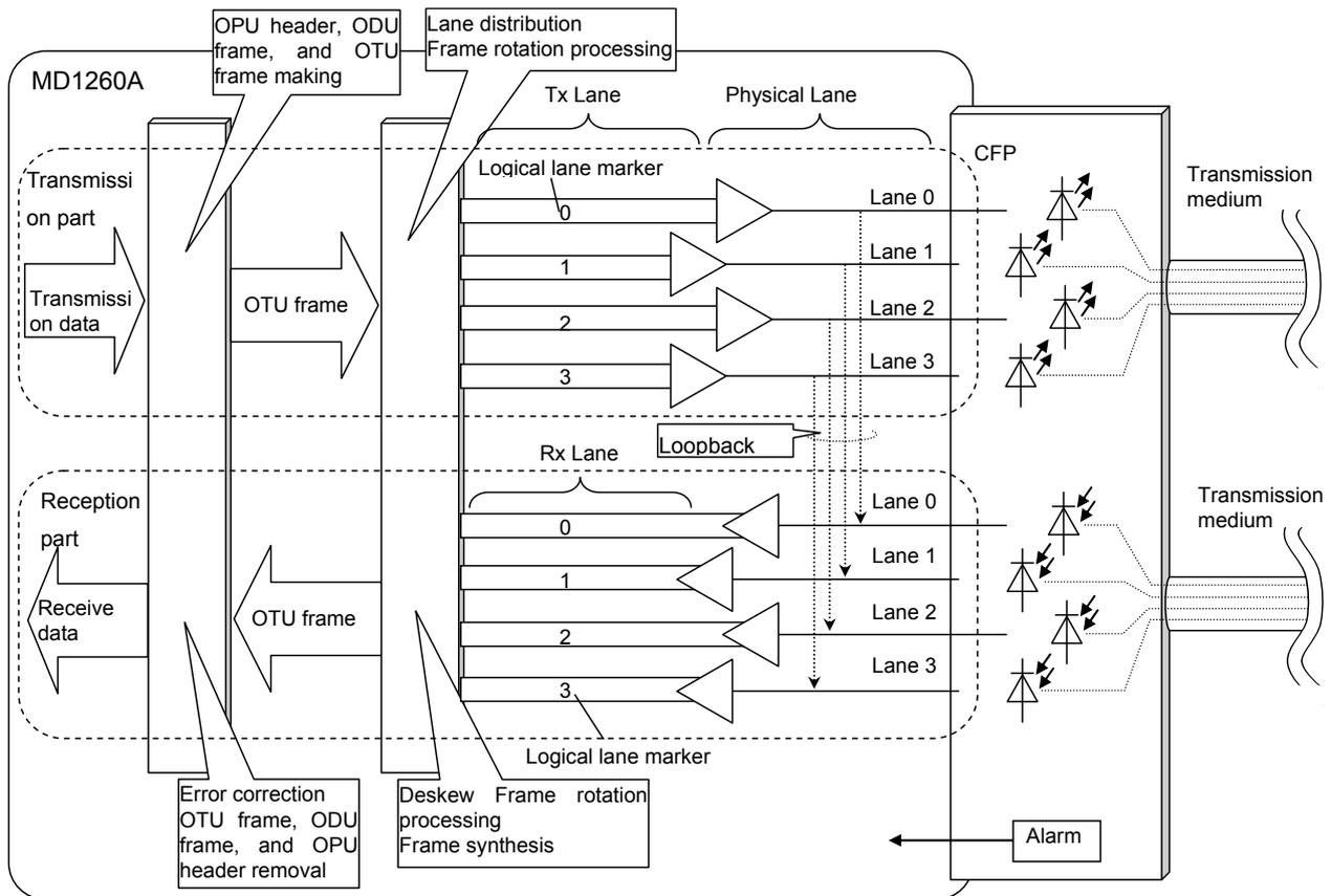
Figure 5.1-1 Flow of OTU3 Signal
