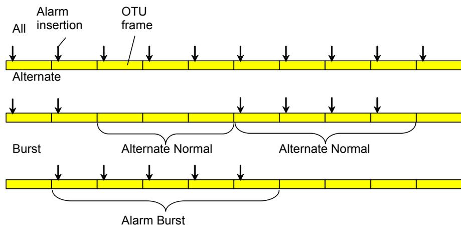
Figure 5.4.9-1 Error/Alarm Insertion Timing
