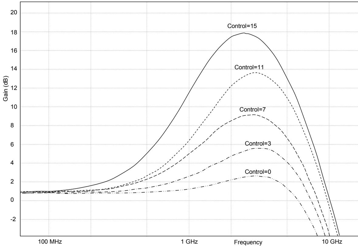
**Figure 3.3.4-4 Frequency Response of Equalizer**
