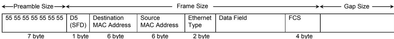
Figure 4.1-2 Format of Ethernet Frame
