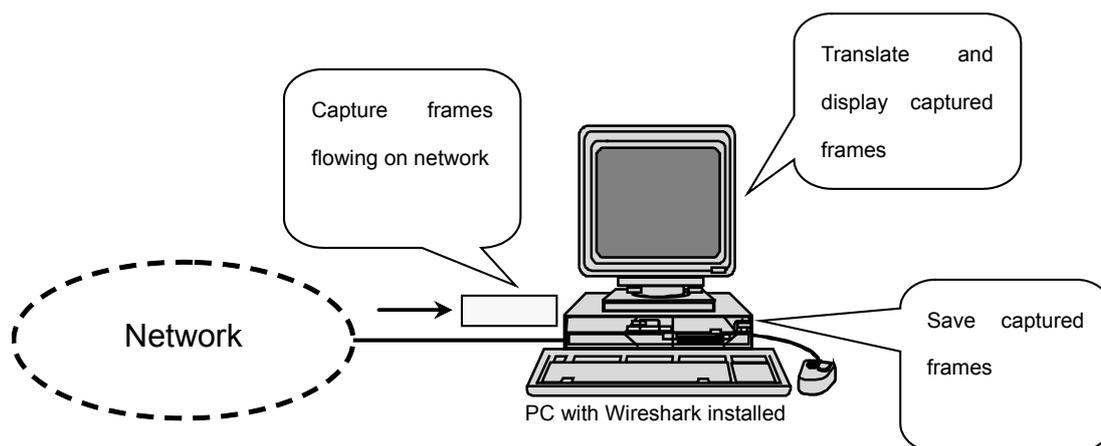
Figure F.1-1 Wireshark Operation
