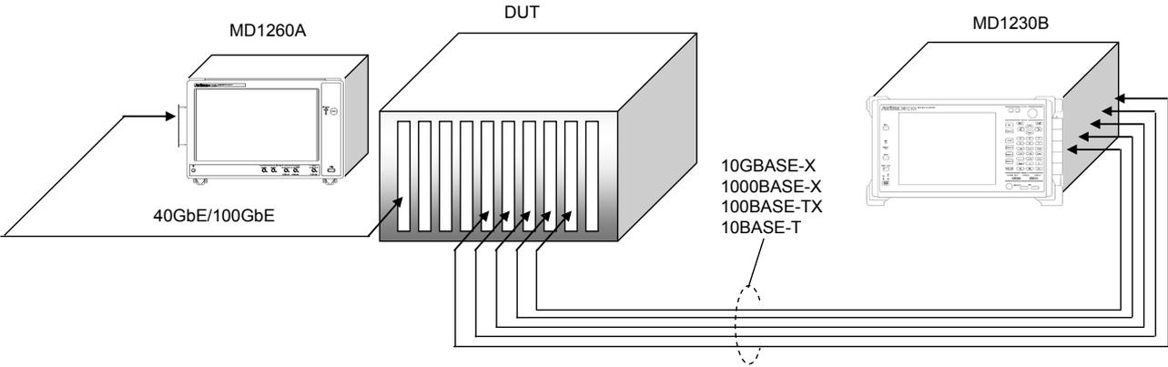
Figure E.1-4 Connecting MD1260A/MD1230A to DUT
