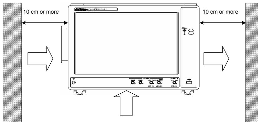
Figure 2.2-2 Vent Airflow System
