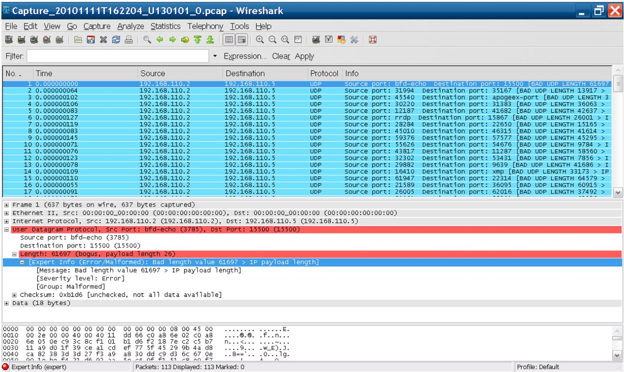
Figure F.1-2 Example of Wireshark Display
