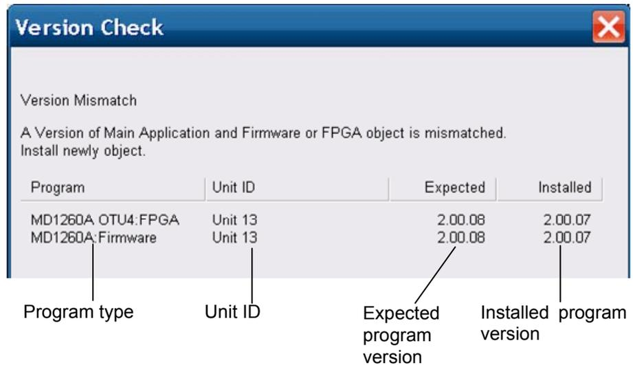
Figure 3.1.1-2 Dialog Indicating Setup Not Completed
