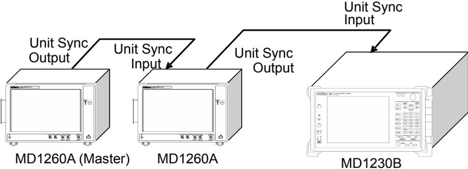
Figure E.1-3 Order of Connecting Coaxial Cable of Two or More Units
