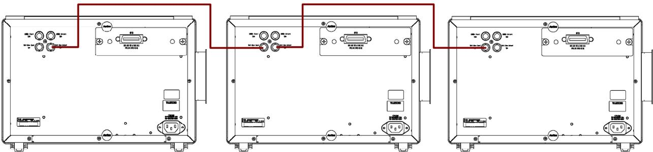
**Figure 2.9-1 Connecting Coaxial Cables**
