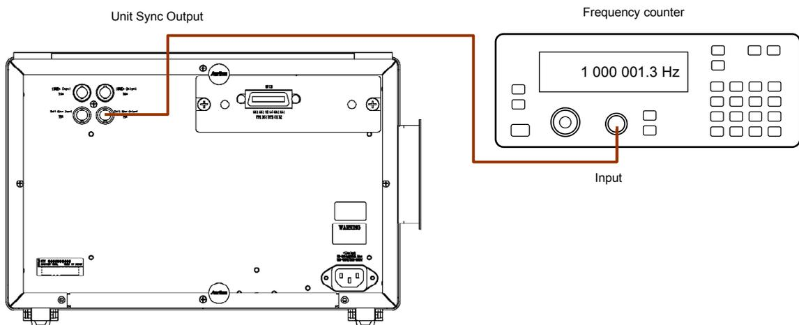
**Figure 8.4-5 Measurement System for Unit Sync Output Terminal**
