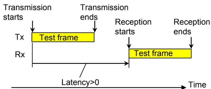
Figure 4.3.1-4 Latency Measurement
