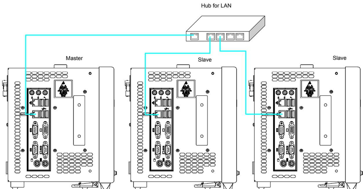
Figure 7.2.3-3 Ethernet Cable Connection (3 MD1260A Units)
