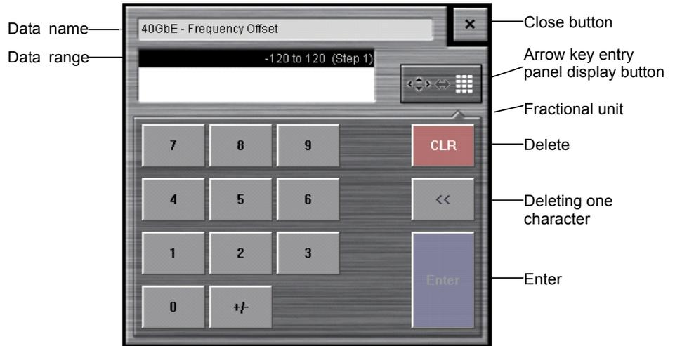
Figure B-2 Numeric Value Entry Panel
