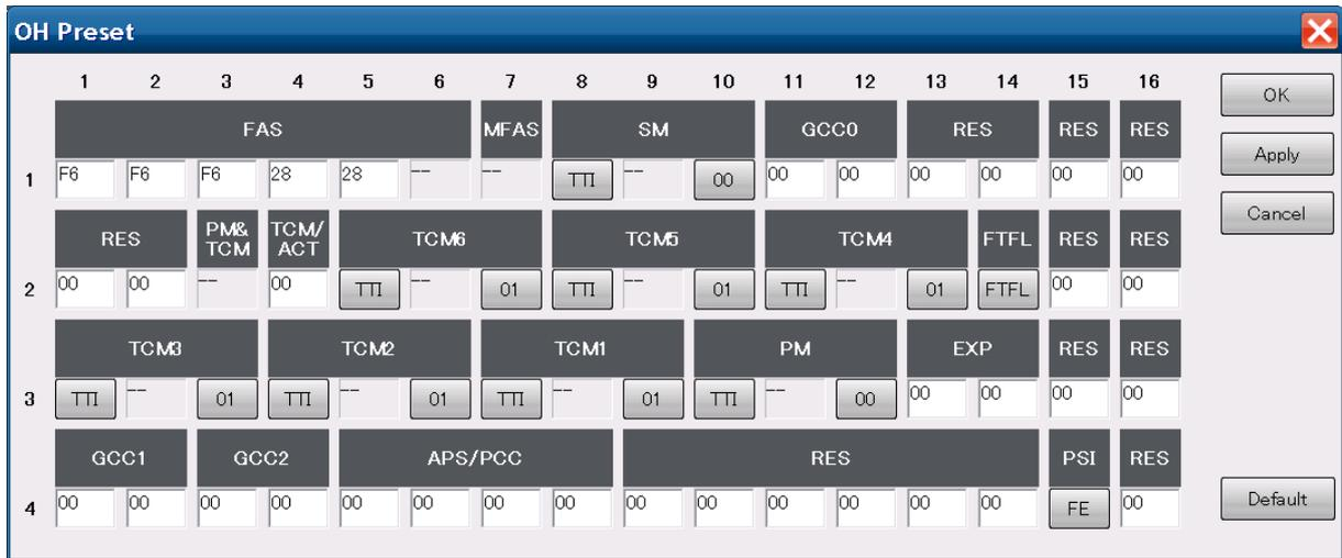
Figure 5.4.3-1 OH Preset Screen (ODU4-PRBS/ODU4-PRBS)
