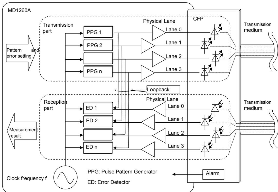
Figure 6.1-1 Signal Flow when Measuring Physical Lane
