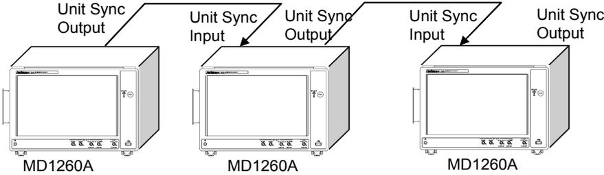
Figure 7.1-3 MD1260A Time Synchronize Method
