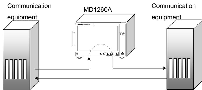
Figure 5.3.1-1 Usage Example of Through Mode
