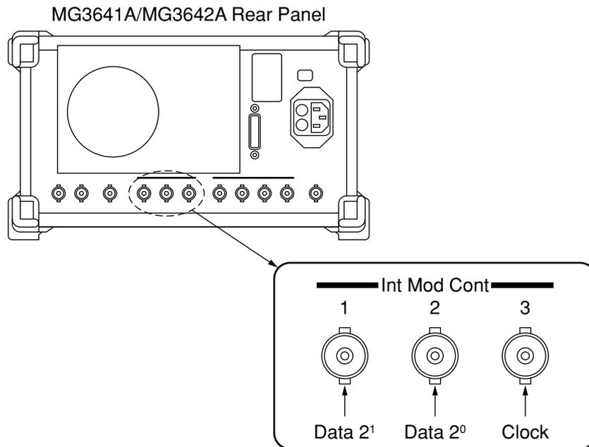
By sticking the attachment labels on near connectors, the erroneous wiring to the connectors can be prevented.
