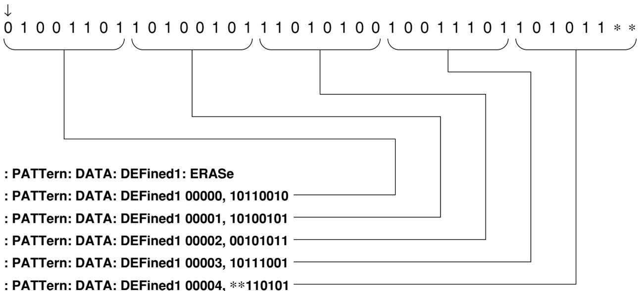
After the data are written, the first delivery address is set to “00000” and the data bit length is set to 38 bits before the delivery.
