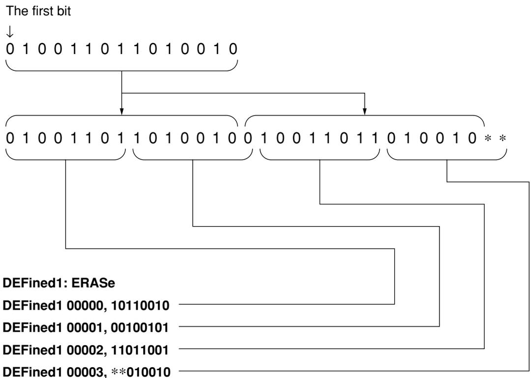
After the data are written, the first delivery address is set to “00000”, the data bit length is set to 30-bits (15 bits×2), and the delivery method is set to 2-bit NRZ output before the delivery.
