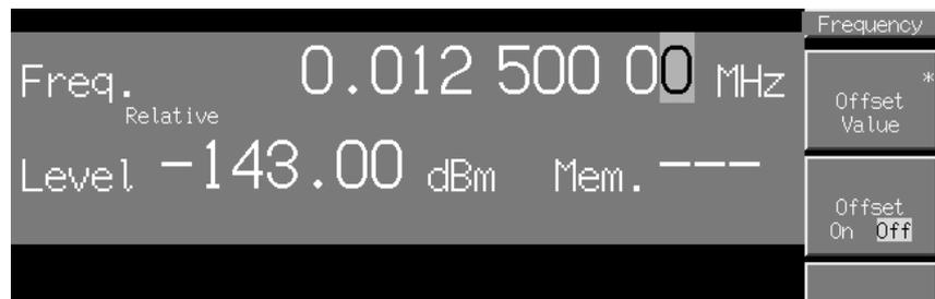
To identify the actual output frequency, press  (Current Frequency). The output frequency will be displayed for about one second.
