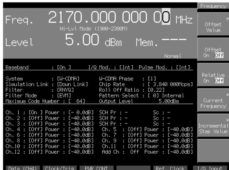
The performance of the RF High Level Output mode is assured only in the range of 1.9 to 2.3 GHz. When the set frequency is out of the range, “Uncal” appears.
