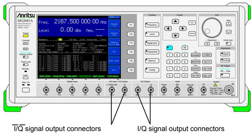
Sample operation: Output  $\overline{I}/\overline{Q}$  signals .
