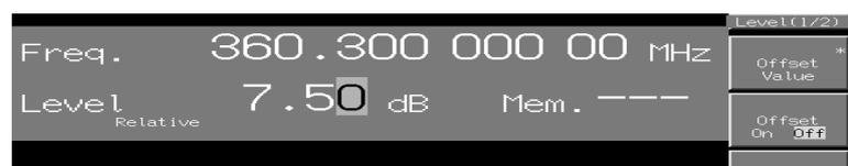
To identify the actual output level, press  $\left[ \begin{array}{c} \text{F4} \\ \text{Current Frequency} \end{array} \right]$  (Current Frequency). The output level will be displayed for about one second.
