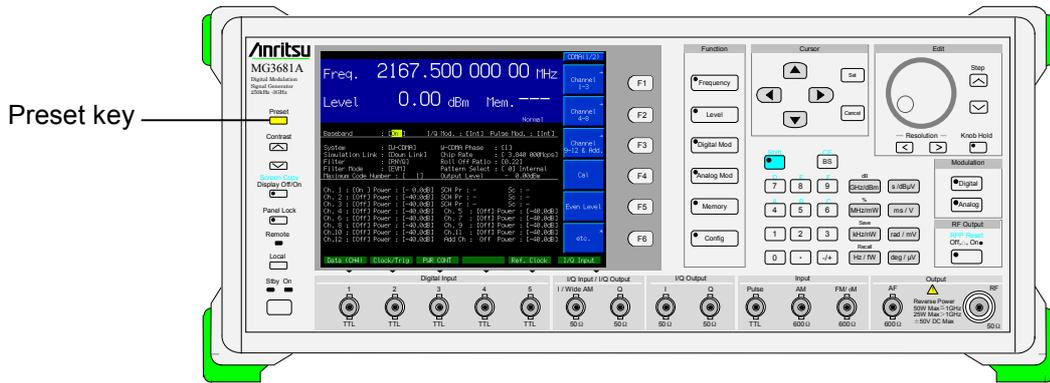
To initialize the entire instrument to the status in which it has been purchased, turn the power on by holding down
