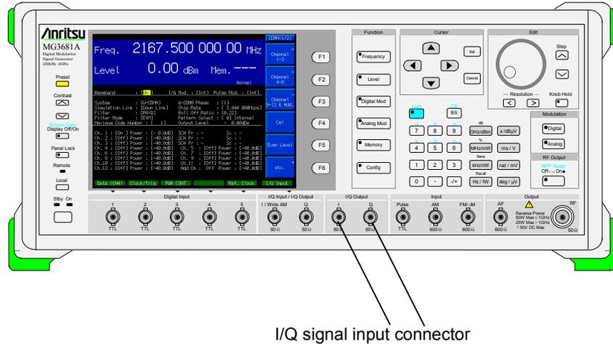
The I/Q signal input connectors are internally terminated at 50Ω. If the rms voltage of  $\sqrt{I^2 + Q^2}$  is 0.5 V in the 50Ω termination state, an RF signal matching the output level setting is outputted. For carrying out vector modulation, input I/Q signals that make the rms voltage of  $\sqrt{I^2 + Q^2}$  equal to 0.5 V. Also set the maximum values of the I/Q signals so that they do not exceed ±1.5 V.
