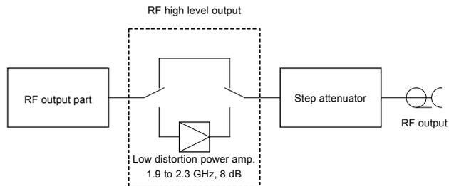
The maximum RF level of W-CDMA modulated wave within the range of 1.9 to 2.3 GHz can be increased 8 dB by turning on the RF High Level Output mode. Also, it is possible to gain the RF Output Signal, which is 8 dB higher, without encouraging the adjacent-channel leakage-power.
