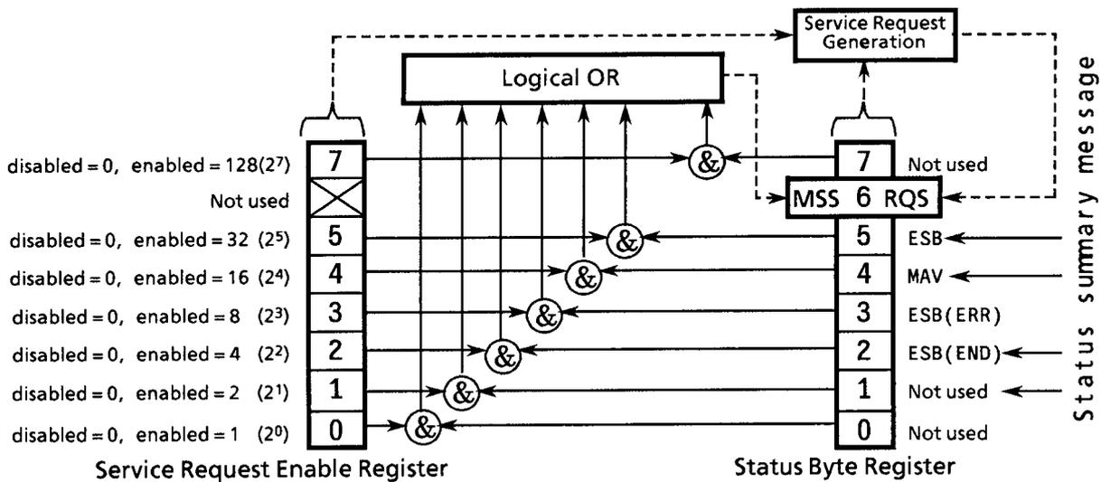
**Use Example** \*SRE48 Controller → This instrument
