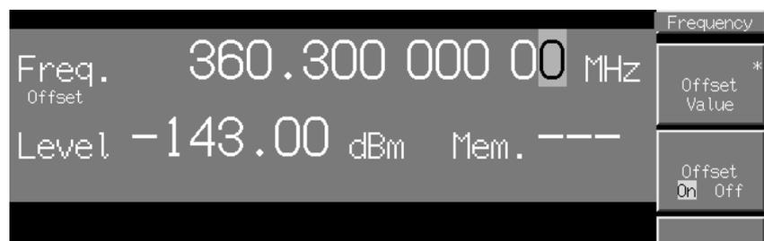
To identify the actual output frequency, press **F4** (Current Frequency). The output frequency will be displayed for about one second.
