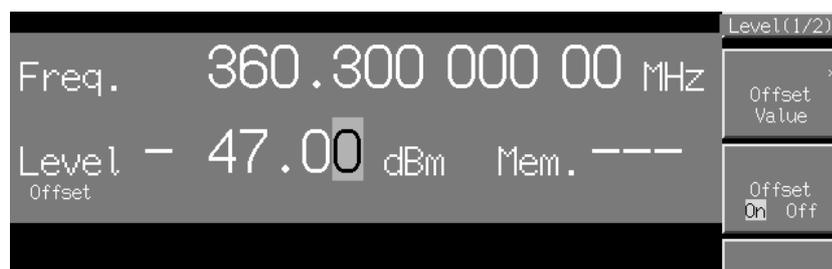
To identify the actual output level, press **F4** (Current Level). The output level will be displayed for about one second.
