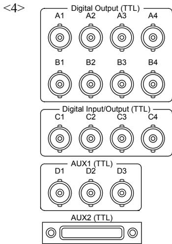
**Digital Signal Input/Output Connectors**
