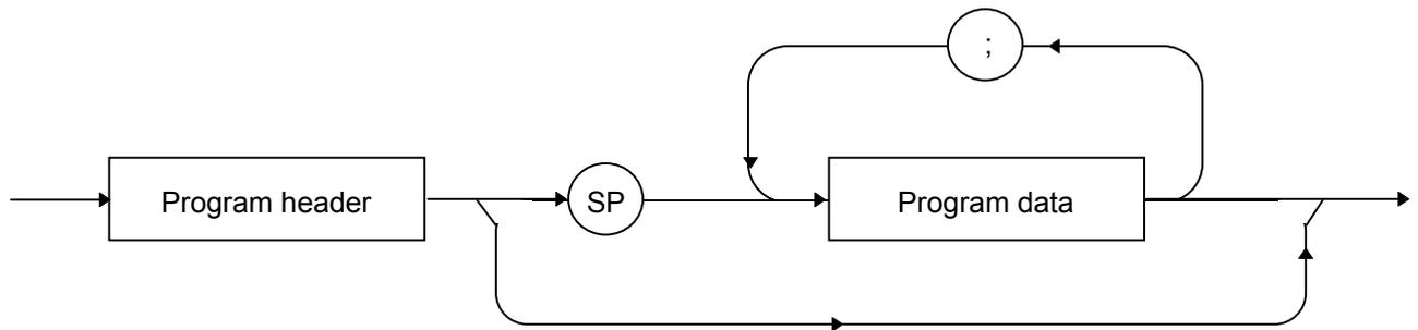
The program header of each IEEE488.2 common command begins with an asterisk (\*). The program header of each program query (query) generally ends with a question mark (?).
