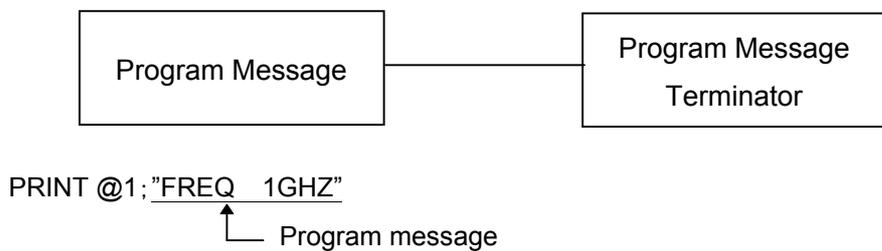
A program message, when transmitted from the controller to this instrument, is terminated by a specified terminator.
