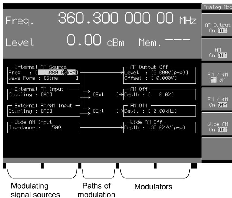
The analog modulation setup screen shows the flow of signals from the modulating signal sources to analog modulation.
