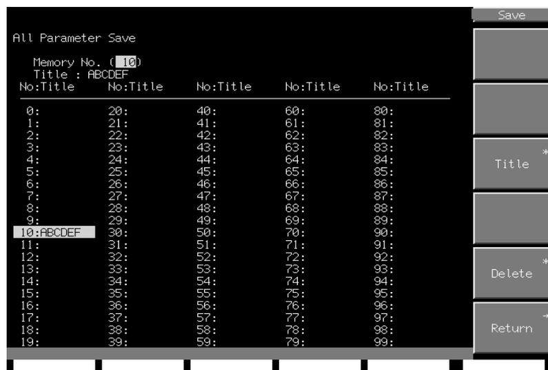
The reverse cursor in the memory location number field and that in the character set can also be moved using the rotary knob or step keys. The digits (0 to 9) and certain letters (A to F) can be entered using the numeric keypad as well. If the numeric keypad is used, the reverse cursor in Entry moves to right without **F2** being pressed.
