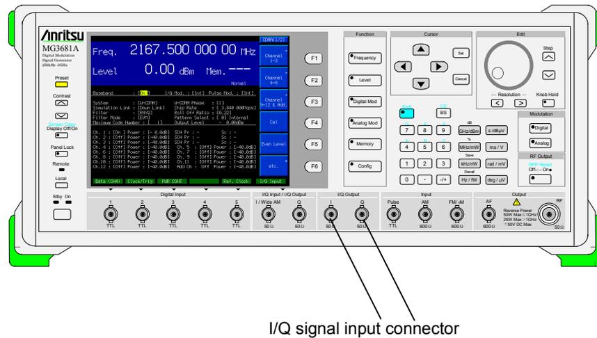
The I/Q signal input connectors are internally terminated at 50Ω. If the rms voltage of  $\sqrt{I^2 + Q^2}$  is 0.5 V in the 50Ω termination state, an RF signal matching the output level setting is outputted. For carrying out vector modulation, input I/Q signals that make the rms voltage of  $\sqrt{I^2 + Q^2}$  equal to 0.5 V. Also set the maximum values of the I/Q signals so that they do not exceed ±1.5 V.
