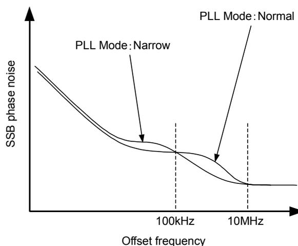
**Sample operation:** Improves the SSB phase noise characteristics at far offset frequency in PLL Mode: Narrow.
