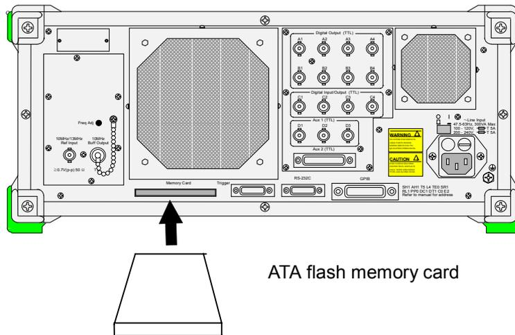
With the target screen displayed, pressing  and then  stores the screen data in the root directory of the ATA flash memory card as a bitmap file. Bitmap file names are automatically assigned in the specified order:
