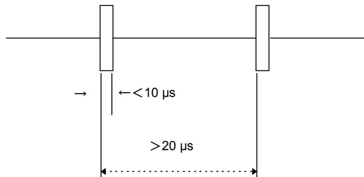
Use the ALC Off mode when using such a modulation signal. In the ALC Off mode, the pulse modulation signal is directly modulated. In this case, level calibration is required because the ALC loop circuit is released in the ALC Off mode.
