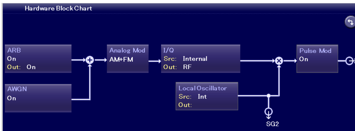
Figure 7.1-1 Outline of MG3710A/MG3710E/MG3740A modulation circuit
