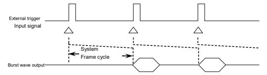
Figure 7.3.8-2 Frame Trigger Timing
