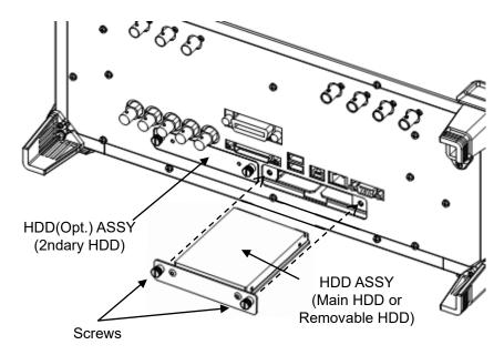
Figure 11.5-1 HDD ASSY Replacement
