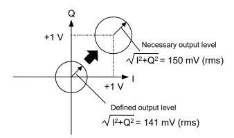
Figure 7.6.3-1 I/Q Signal Output Adjustment Image
