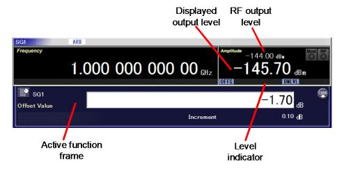
Figure 5.3.2-2 Offset Level Setting
