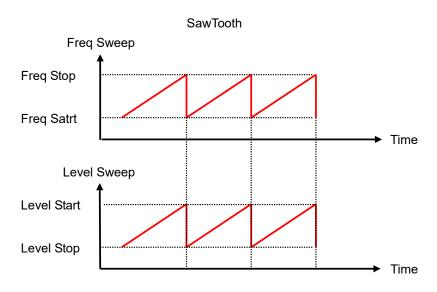
Figure 6.3.1-7 Saw Tooth (Normal) Sweep
