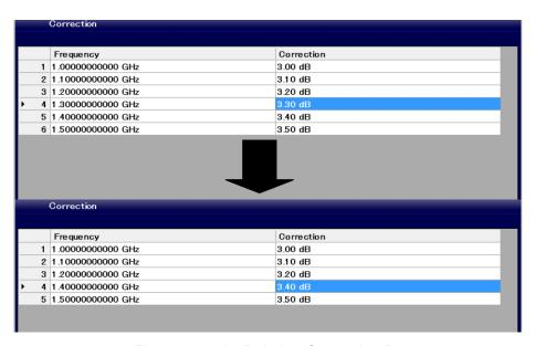
Figure 5.4.4-1 Deleting Correction Data
