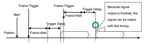
Figure 7.3.9-2 Frame Trigger No Retrigger
