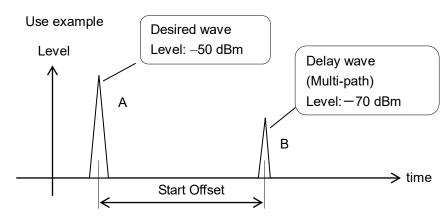
Figure 7.3.2-10 Example of Desired Wave and Delay Wave with Same Frequency
