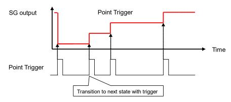
Figure 6.5-2 Point Trigger
