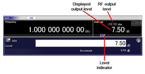
Figure 5.3.1-1 Relative Level Display
