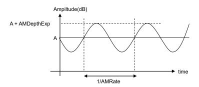
Figure 7.2.1-2 AM Modulation (Log)
