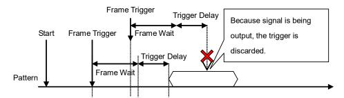
Figure 7.3.9-1 Frame Trigger No Retrigger
