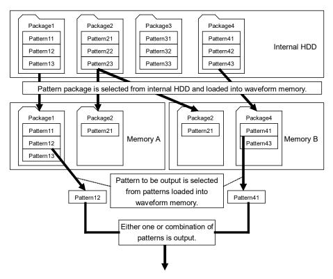
Figure 7.3-2 Outline of Waveform Pattern Output
