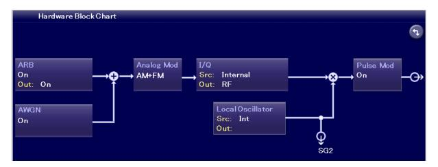
Figure 7.1-1 Outline of MG3710A/MG3710E/MG3740A modulation circuit
