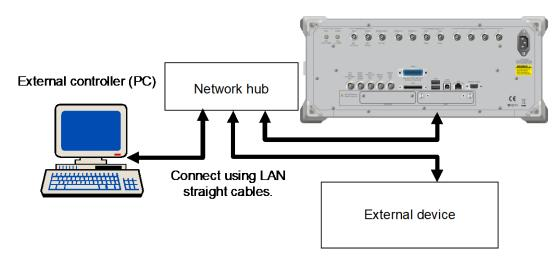
Figure E.2.2-2 Sample connection with multiple external devices
