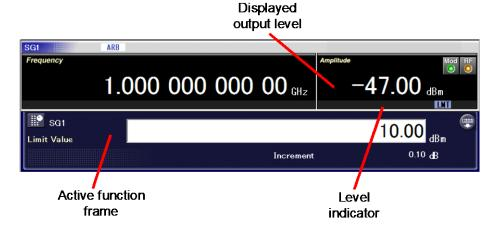
Figure 5.3.3-1 Output Limit Level
