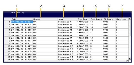
Figure 8.6-1 BER Test Log
