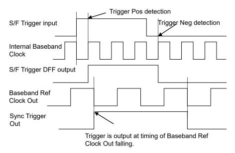
Figure 7.4.2-1 Sync Trigger Out
