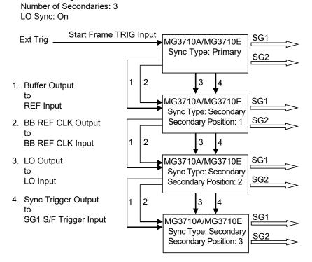
Figure 7.3.15-1 Sync Multi SG Configuration
