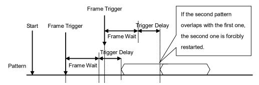
Figure 7.3.9-4 Frame Trigger Restart on Trigger
