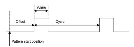
Figure 7.3.12-2 Offset, Width, Cycle
