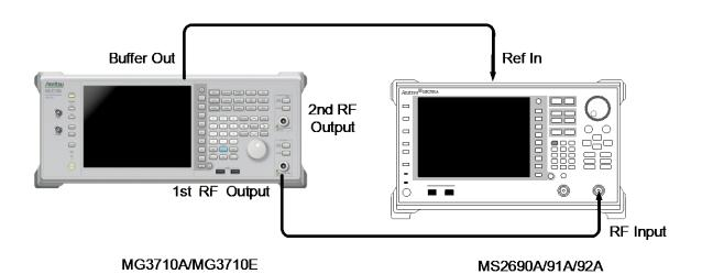
Test procedure W-CDMA (Test Model 4)
