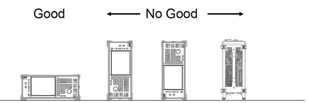
Figure 2.1.1-1 Installation Orientation
