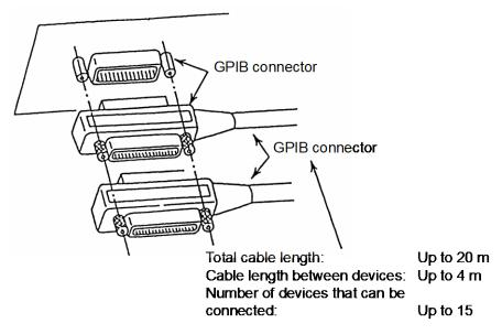
Figure E.2.1-1 GPIB cable connection
