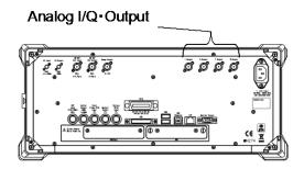
Figure 7.6-5 Analog I/Q Output Connector
