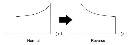
Figure 4.6.3-1 RF Spectrum: Two Waves Not Added
