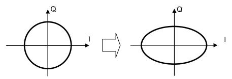
Figure 7.6.4-1 Gain Balance
