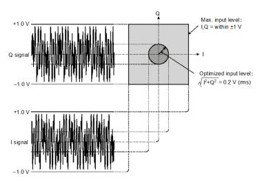
Figure 7.6-2 I/Q Signal Input Level
