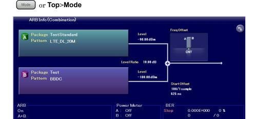
Figure 7.3.2-9 Two Waves Added Output
