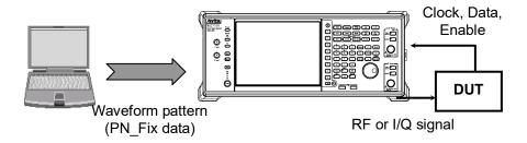
Figure 8.4.3-2 BER Measurement with PN\_Fix Data
