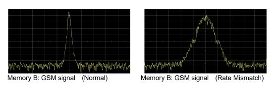
Figure 7.3.2-8 Memory B Waveform of Rate Mismatch
