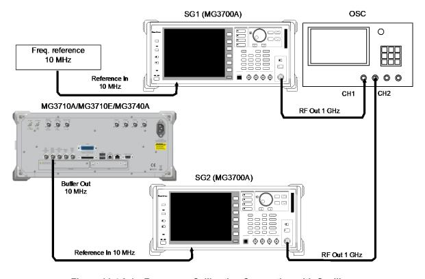
Figure 11.4.3-1 Frequency Calibration Connection with Oscilloscope
