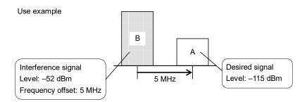
Figure 7.3.2-12 Example of Frequency Offset
