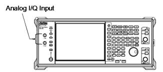
Figure 7.6-1 Analog I/Q Input Connector
