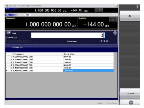
Figure 5.4.2-2 Correction Level Setting
