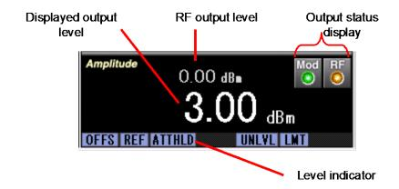
Figure 5.1.1-1 Output Level Setting Screen
