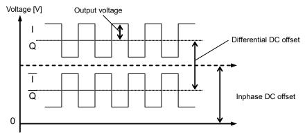
Figure 7.6.3-2 I/Q Signal Output Image
