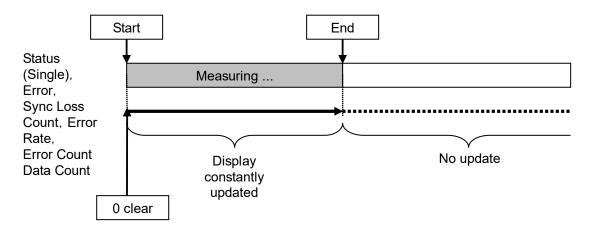
Figure 8.3.2-2 Measure Mode: Single or Endless
