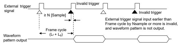
Figure 7.3.8-3 Frame Trigger Cycle
