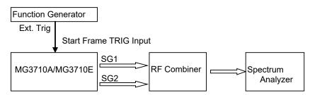
Figure 7.3.15-2 Phase Synchronization/Timing Synchronization
