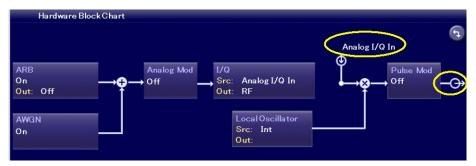
Figure 7.6-4 Modulation Status with External I/Q Signal
