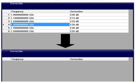
Figure 5.4.5-1 Deleting Correction Table
