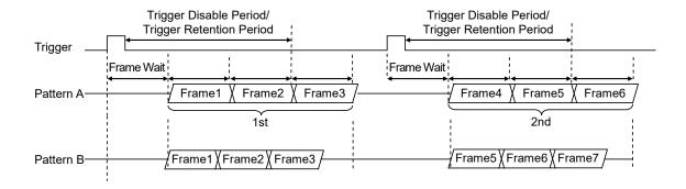
Figure 7.3.10-4 Frame Trigger to add two waves
