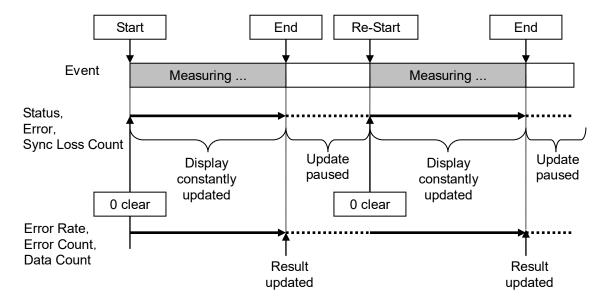
Figure 8.3.2-1 Measure Mode: Continuous
