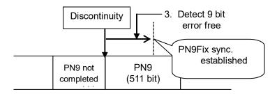
Figure 8.4.2-1 Example: Synchronization Establishing of PN9Fix Pattern
