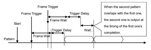
Figure 7.3.9-3 Frame Trigger Buffered Trigger
