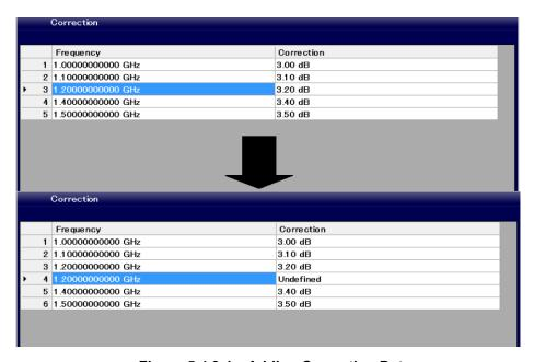
Figure 5.4.3-1 Adding Correction Data
