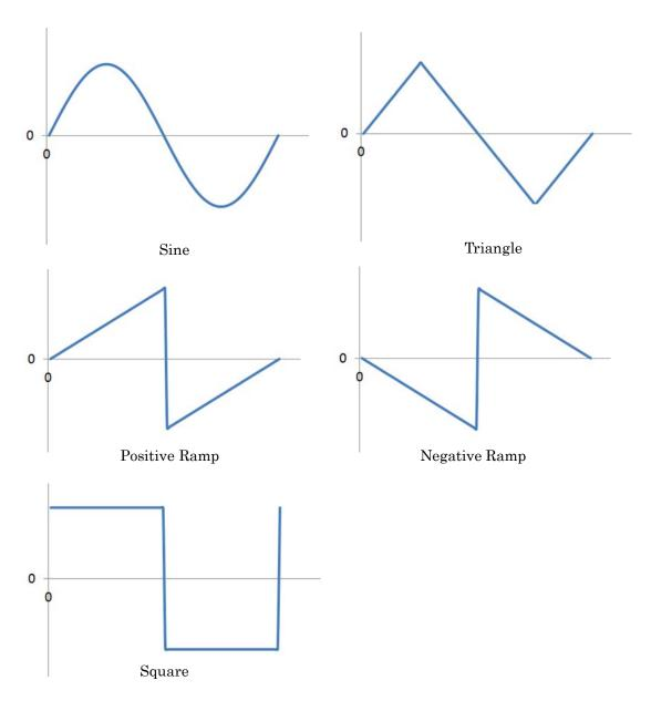
Figure 7.2.1-3 Type of Analog Waveform
