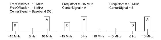
Figure 7.3.3-1 Example of Frequency Offset Setting
