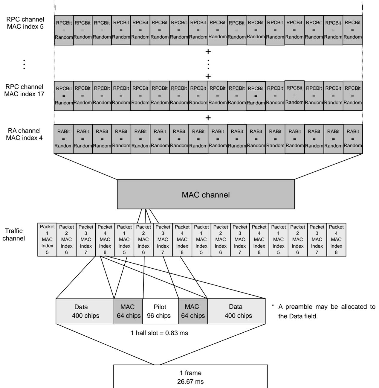
Figure 3.9.1-5 Multiplexing channels
