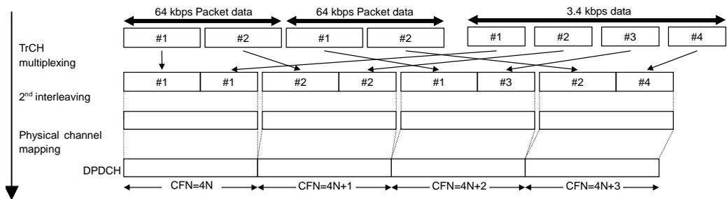
Figure 3.1.2-6 Multiplexing for UL 64 kbps packet
