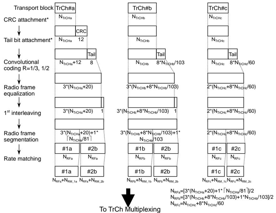
\* CRC and tail bits for TrCH#a is attached even if  $N_{TrCHa}=0$  bits since CRC parity bit attachment for 0 bit transport block is applied.
