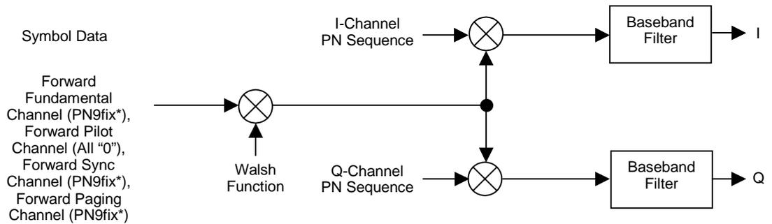
**Figure 3.8.7-1 Signal generation block diagram of waveform pattern FWD\_RC1-2 9channel**
