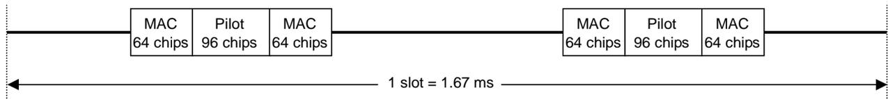
Figure 3.9.3-2 Format of 1xEV-DO forward idle slot waveform pattern
