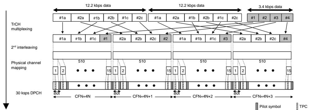
Figure 3.1.5-2 Channel coding and multiplexing for DL AMR TFCSx (2 of 2)
