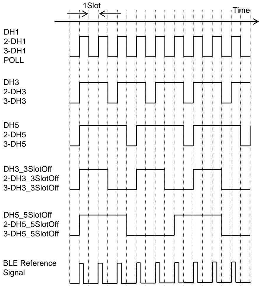
Figure 3.12-1 Timing chart of waveform patterns
