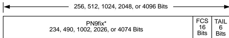
**Figure 3.9.2-1 Format of 1xEV-DO reverse packet**
