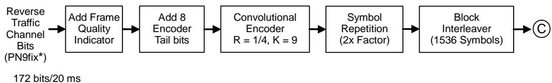
**Figure 3.8.3-2 Signal generation block diagram of waveform pattern RVS\_RC3\_FCH (1/2)**
