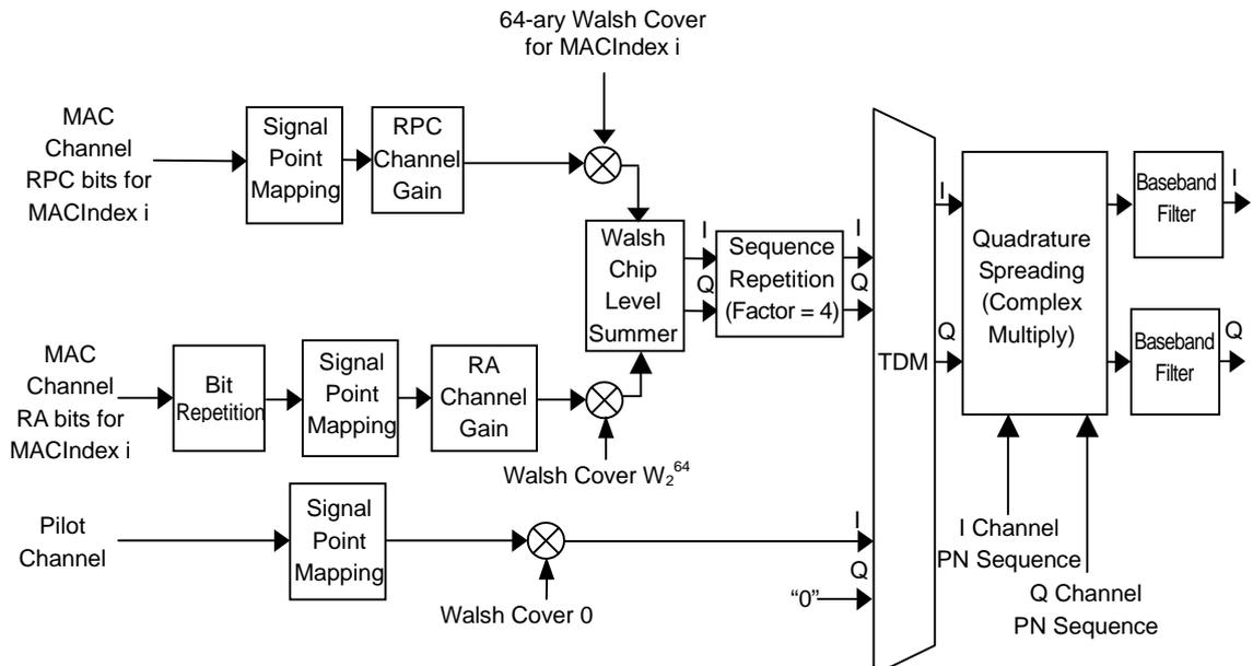
Figure 3.9.3-1 Signal generation block diagram of 1xEV-DO forward idle slot waveform pattern
