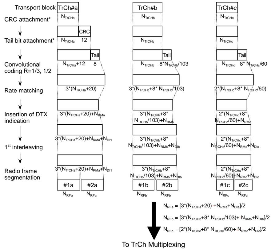
\* CRC and tail bits for TrCh#a is attached even if N<sub>TrCh#a</sub>=0 bits since CRC parity bit attachment for 0 bit transport block is applied.
