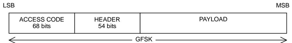
Figure 3.12.1-1 Packet configuration for Basic Rate waveform
