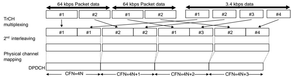
Figure 3.1.2-4 Multiplexing for UL ISDN
