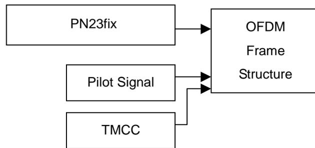
**Figure 3.11.1-2 Generation of the waveform patterns for ISDB-T**
