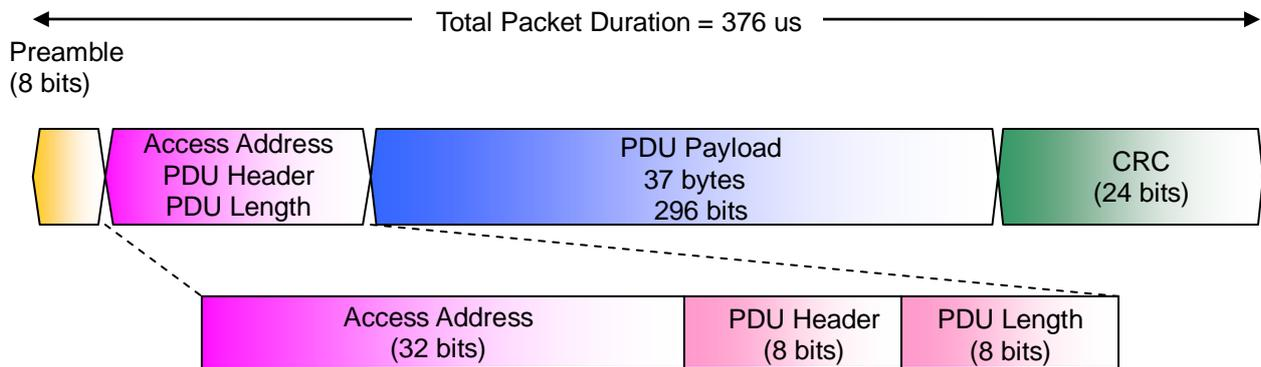
Figure 3.12.3-1 Packet Configuration for BLE Waveform
