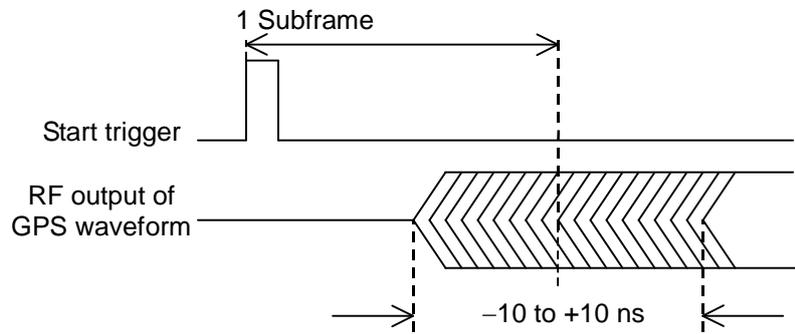
Figure 3.13-1 SYNC\_ADJ output timing
