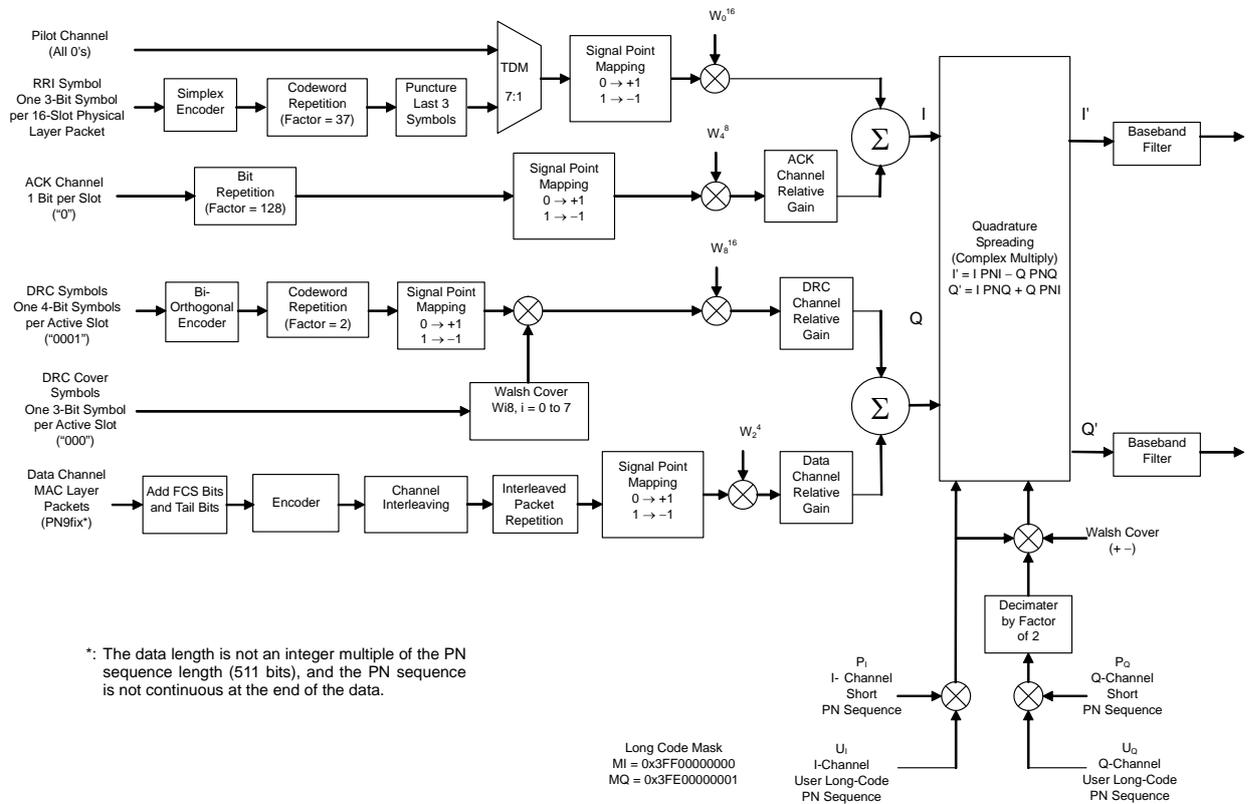
Figure 3.9.2-2 Signal generation block diagram of 1xEV-DO reverse waveform pattern
