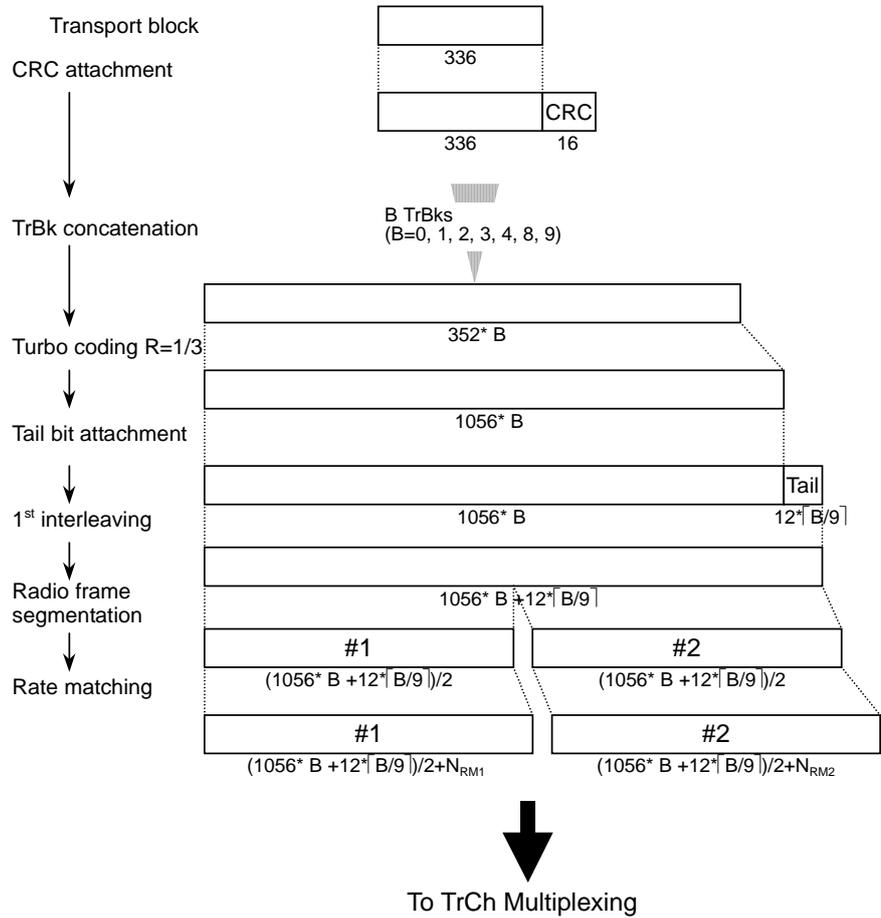
Figure 3.1.2-5 Channel coding for UL 64 kbps packet
