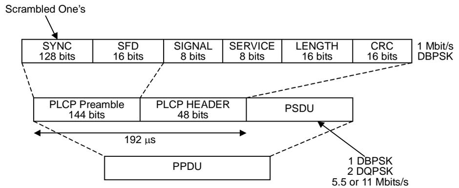
**Figure 3.10.2-1 IEEE802.11b Long PLCP PDU frame format**
