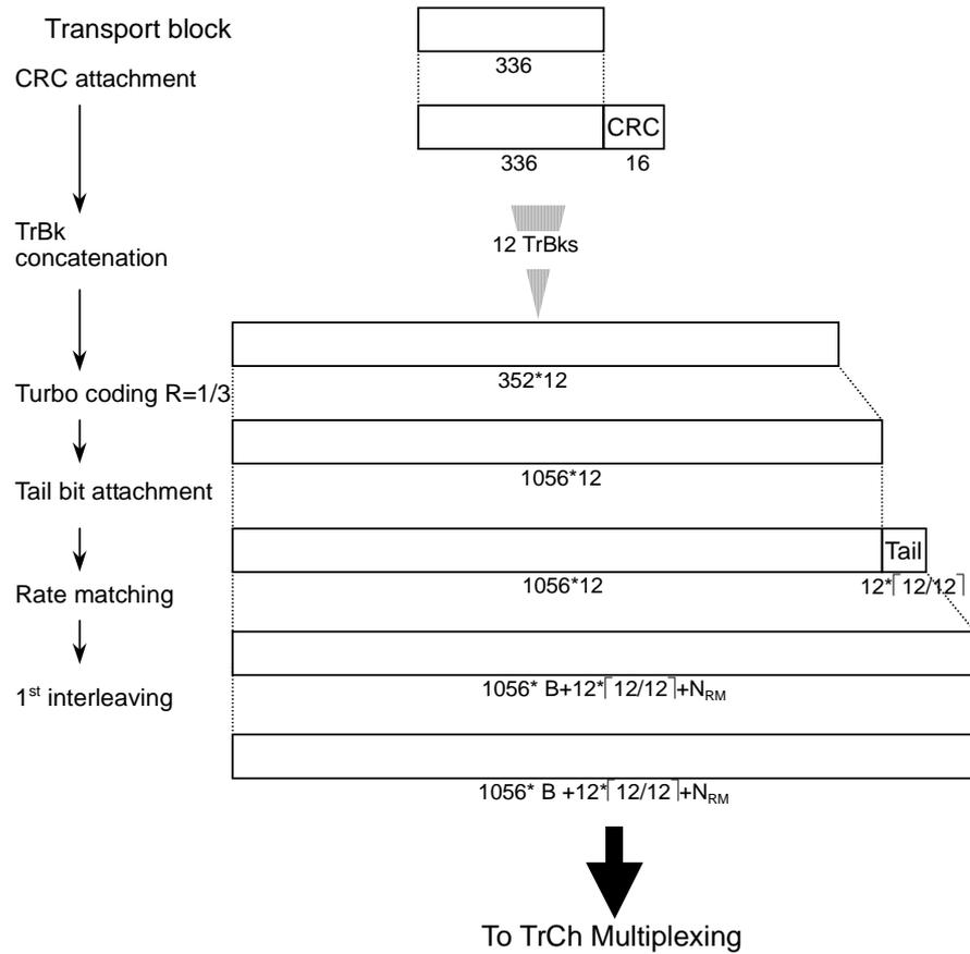
**Figure 3.1.5-4 Channel coding for DL 384 kbps packet**
