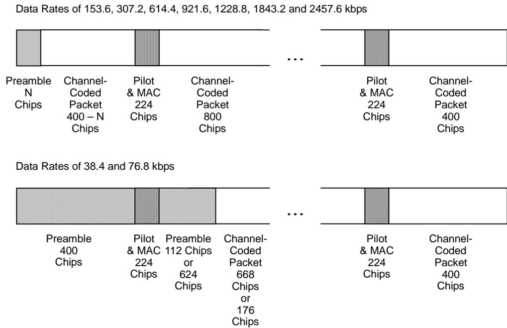
Figure 3.9.1-4 TDM timing diagram
