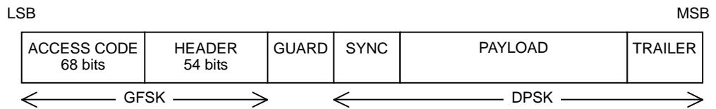
Figure 3.12.2-1 Packet configuration for Enhanced Data Rate waveform
