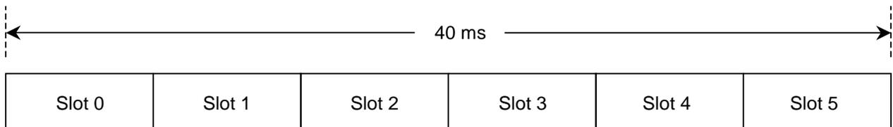
Figure 3.4.1-2 Frame configuration at half rate
