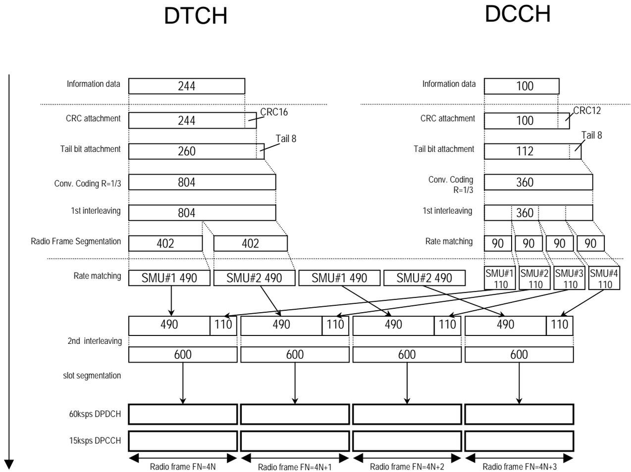
Figure 3.1.1-2 Channel coding for UL reference measurement channel (12.2 kbps)
