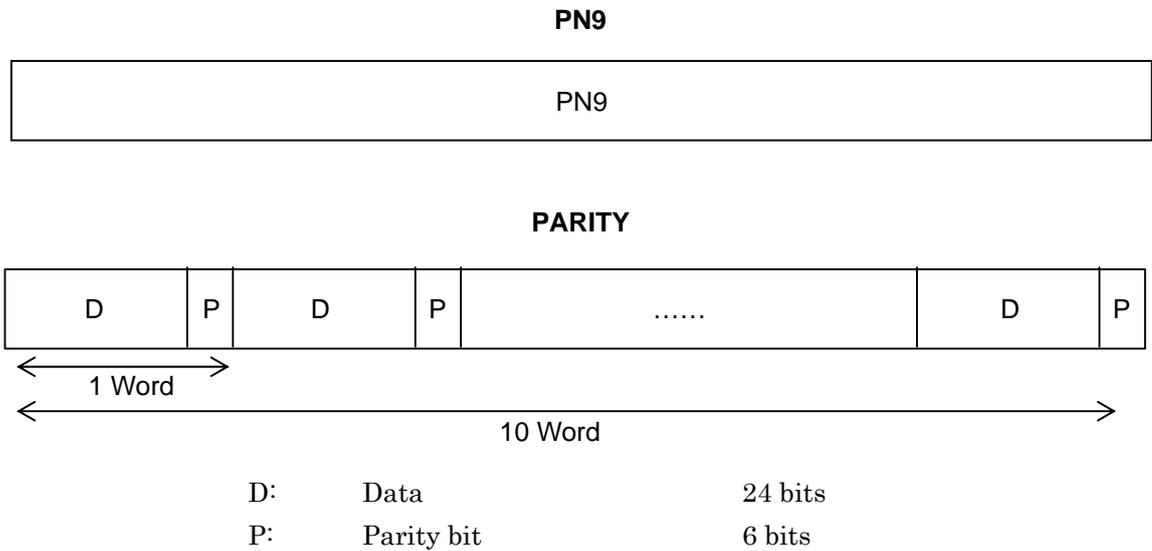
PN9fix data is allocated to the Data part. Adjacent Word PN data is contiguous but the PN data is discontinuous at the 10th Word and the 1st Word of the next cycle.
