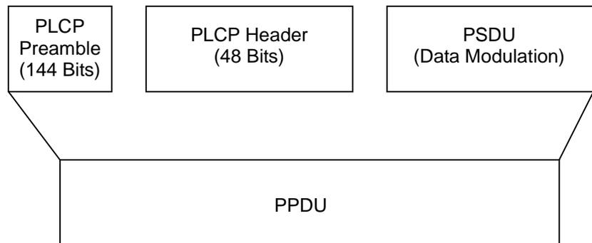
**Figure 3.10.3-1 IEEE802.11b Long preamble PDU frame format**
