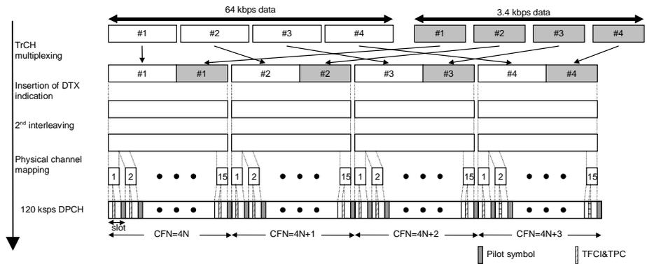
Figure 3.1.5-3 Channel coding and multiplexing for DL ISDN
