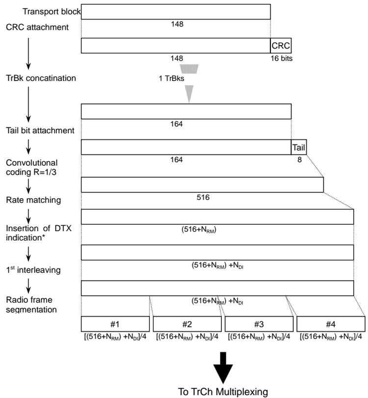
\* Insertion of DTX indication is used only if the position of the TrChs in the radio frame is fixed.
