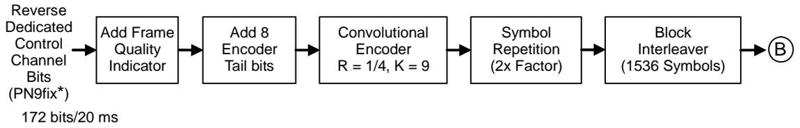
Figure 3.8.5-2 Signal generation block diagram of waveform pattern RVS\_RC3\_DCCH (1/2)
