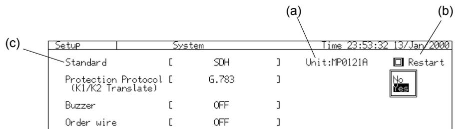
(a) : Displays the unit that is currently being used in either the MP0122A/B slot or Slot 1.
