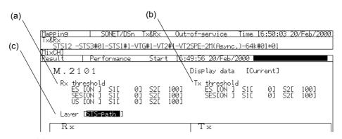
(a) Rx threshold ..... sets the threshold for judging the received signal.
