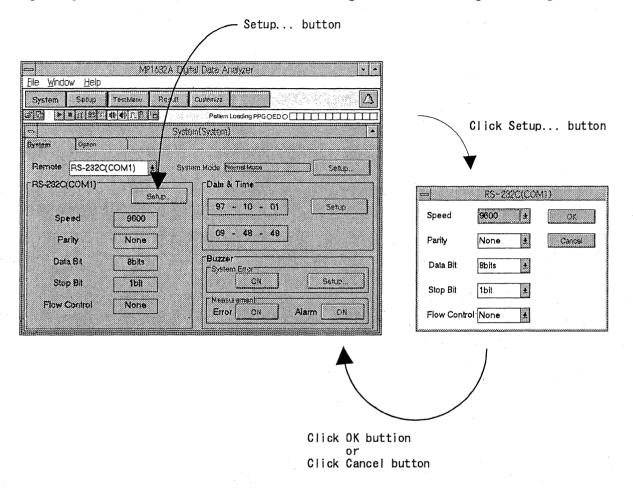
Fig. 5-9 Basic Setup Procedures
