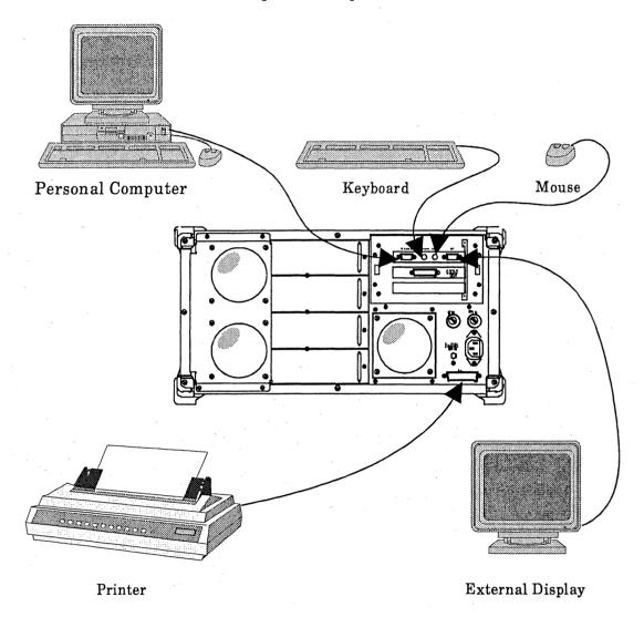
Fig. 3-4 Connecting peripherals and external instruments
