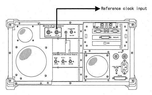
Fig. 3-7 Connection to peripherals
