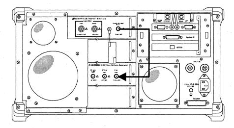
Fig. 3-5 Connection between internal synthesizer and PPG
