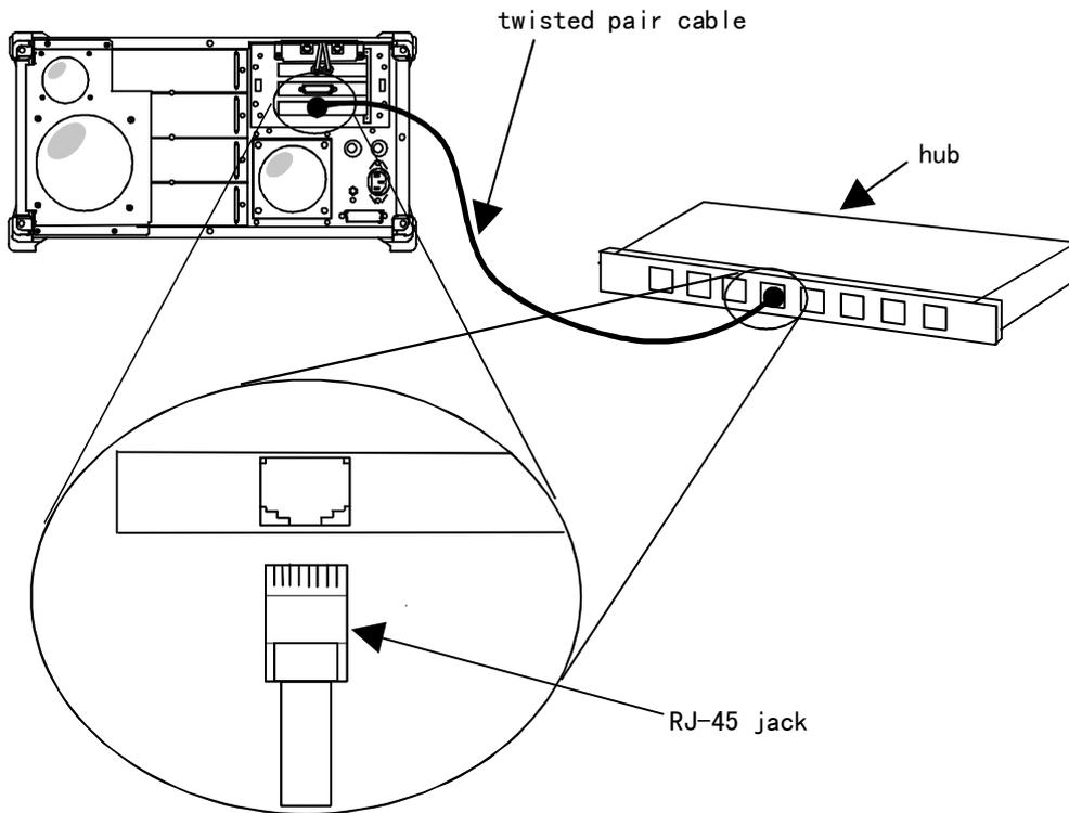
**Fig. 2-1 Connecting the Ethernet Cable**
