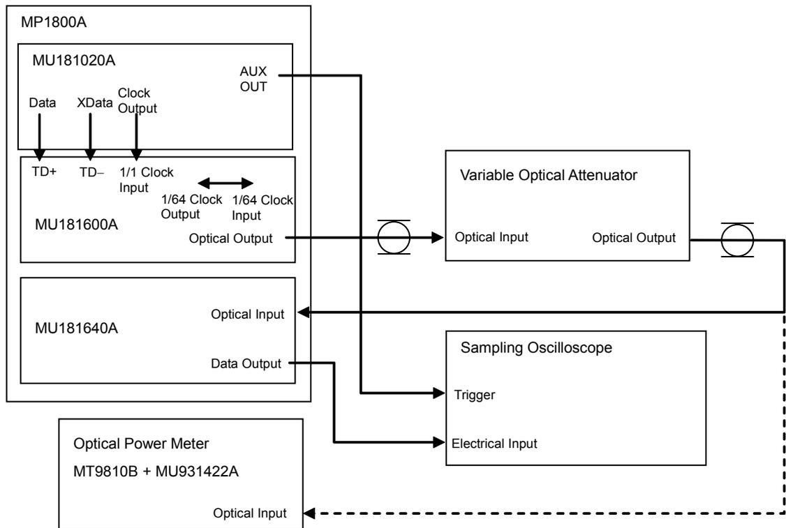
**Fig. 6.3.2-1 Connection diagram for receiver data output level measurement (850 nm)**
