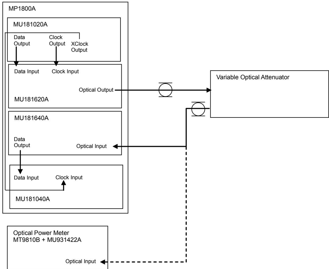
**Fig. 6.3.1-2 Connection diagram for receiver light receiving sensitivity measurement (1310 nm, 1550 nm)**
