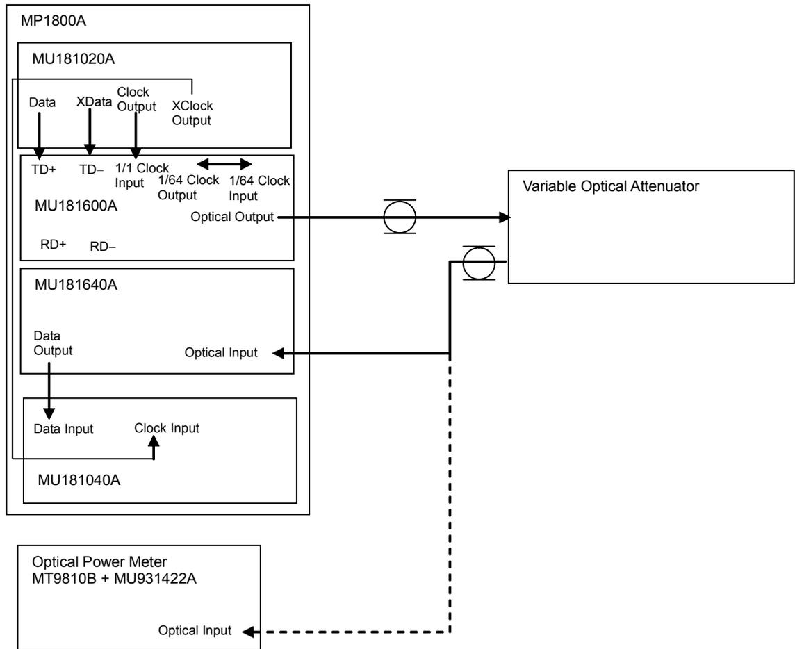
**Fig. 6.3.1-1 Connection diagram for receiver light receiving sensitivity measurement (850 nm)**
