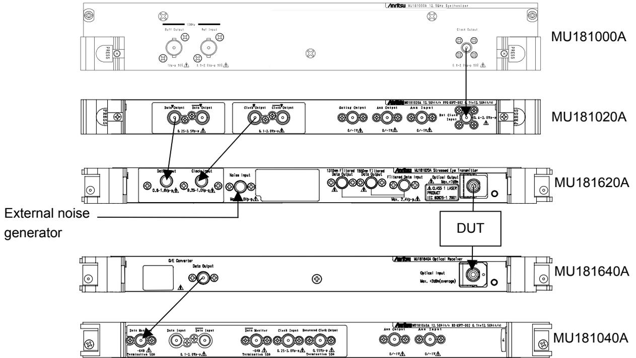
Fig. 3.2-1 Example of inter-module connection
