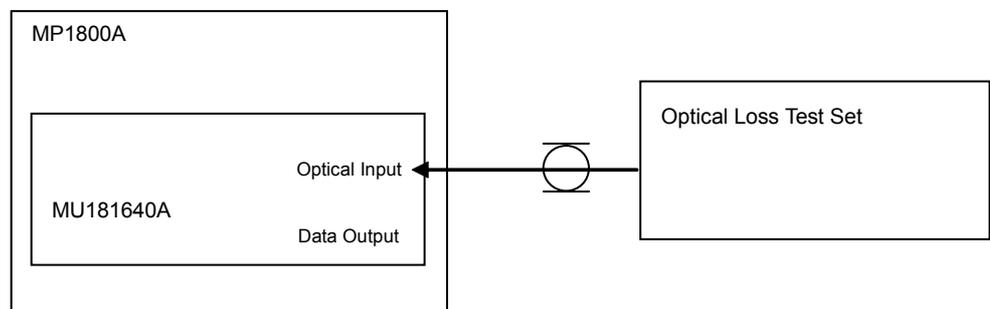
**Fig. 6.3.3-1 Connection diagram for return loss measurement**
