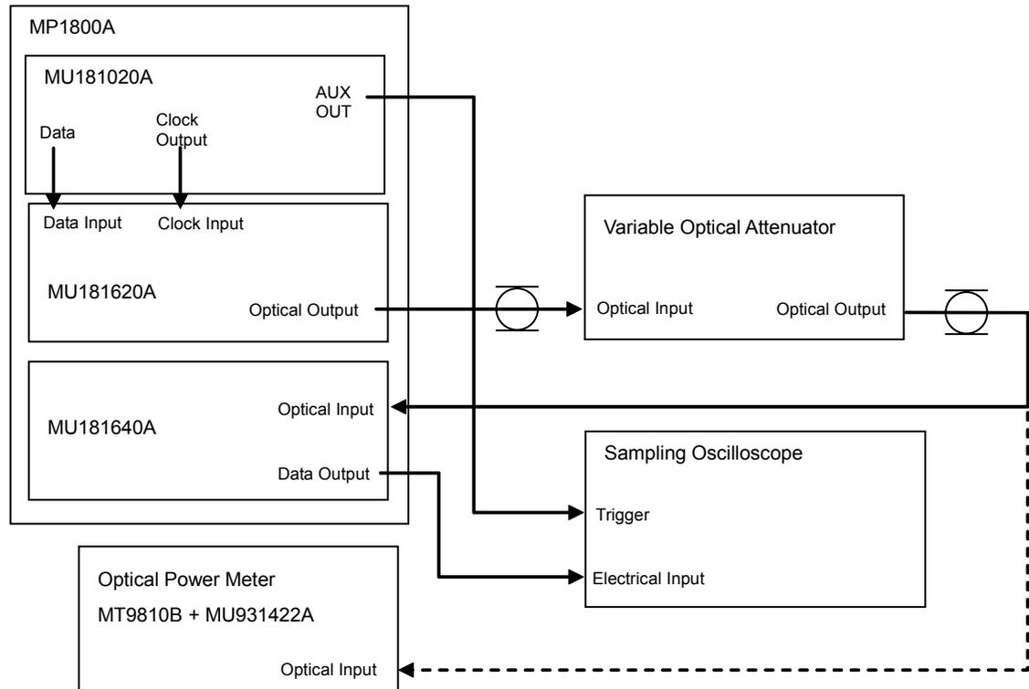
**Fig. 6.3.2-2 Connection diagram for receiver data output level measurement (1310 nm, 1550 nm)**
