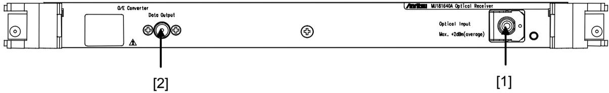
Fig. 3.1.1-1 Panel of MU181640A
