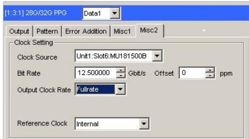
Figure D.3-2 Output Clock Rate Setting on the Misc2 Tab of MU183020A
