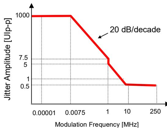
**Figure 3.5-5 Total Jitter Added (When Interacting With 64G PPG)**
