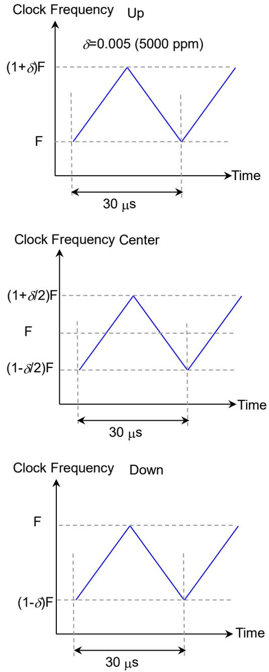
**Figure 3.4.2-2 Setting Type and Changing Frequency (Frequency: 33 kHz)**
