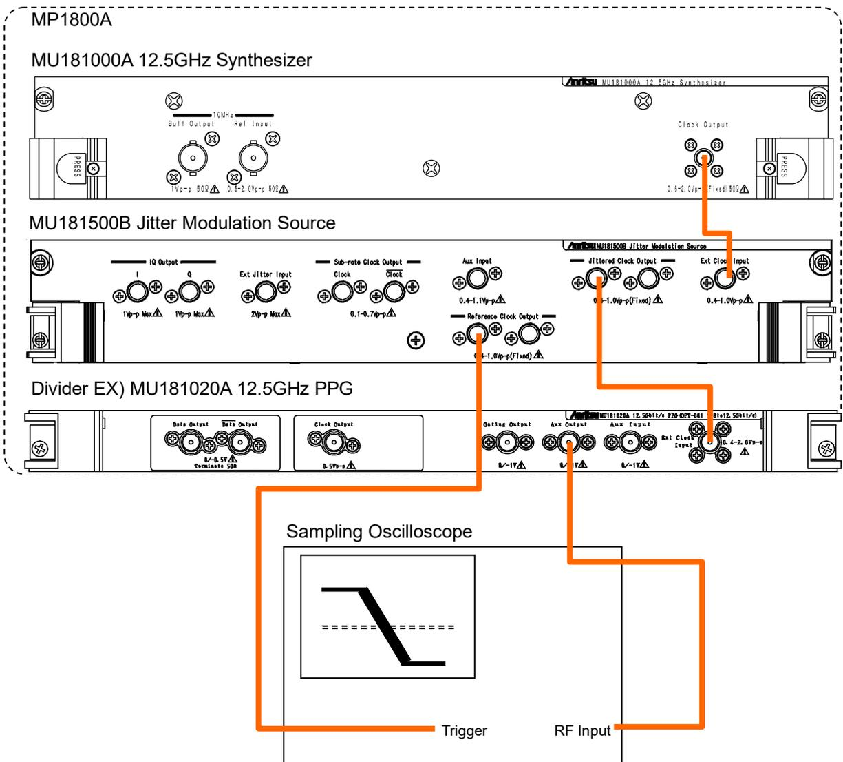
Figure 6.3.3-1 BUJ Measurement Setup
