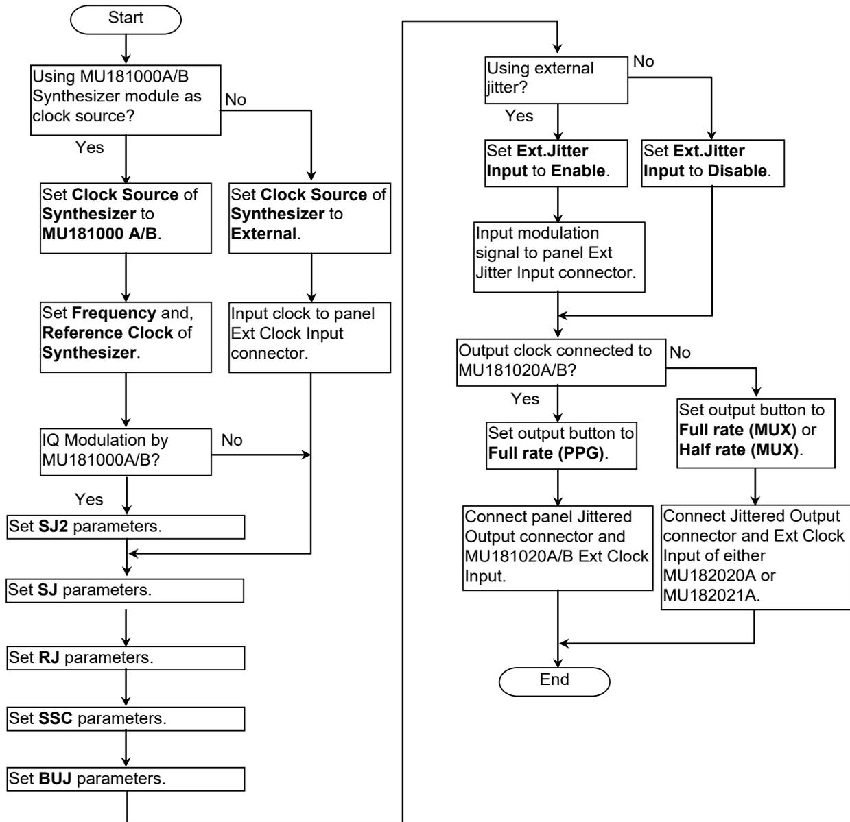
Figure 3.1-1 Jitter Modulation Source Basic Setting Procedure
