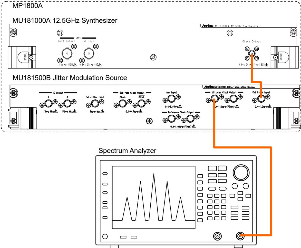
Figure 6.3.1-1 Setup when SJ Amplitude  $\leq 0.4$  Ulp-p
