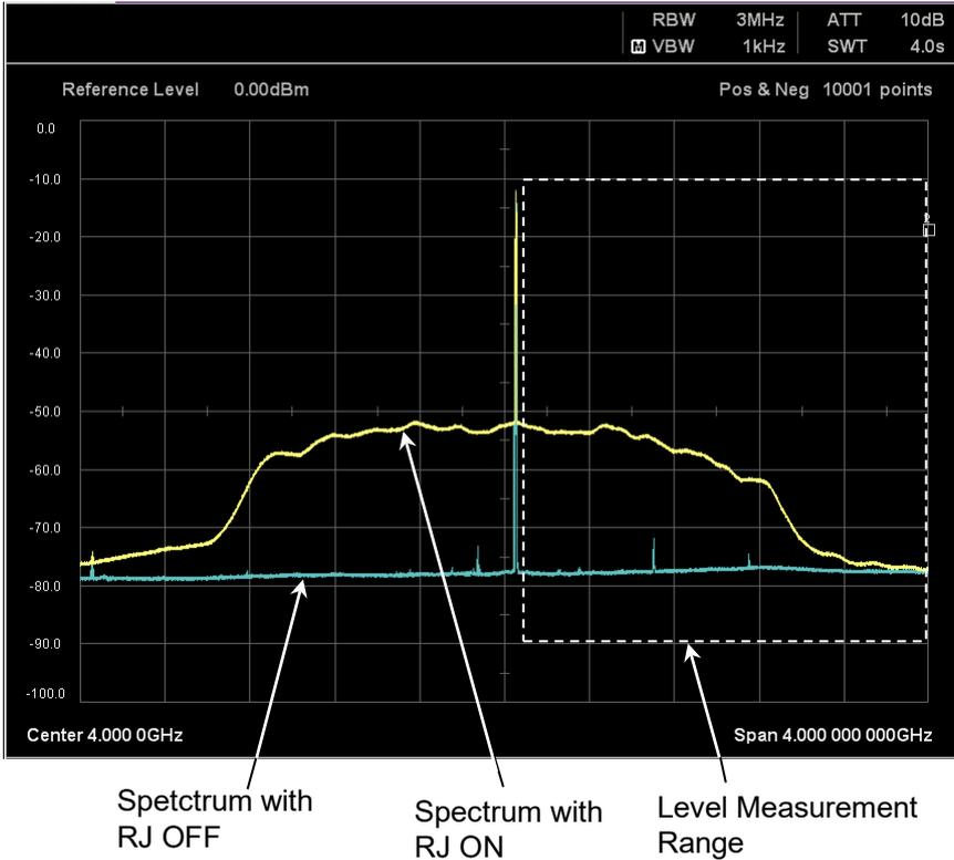
Figure 6.3.2-1 Power Measured by Spectrum Analyzer
