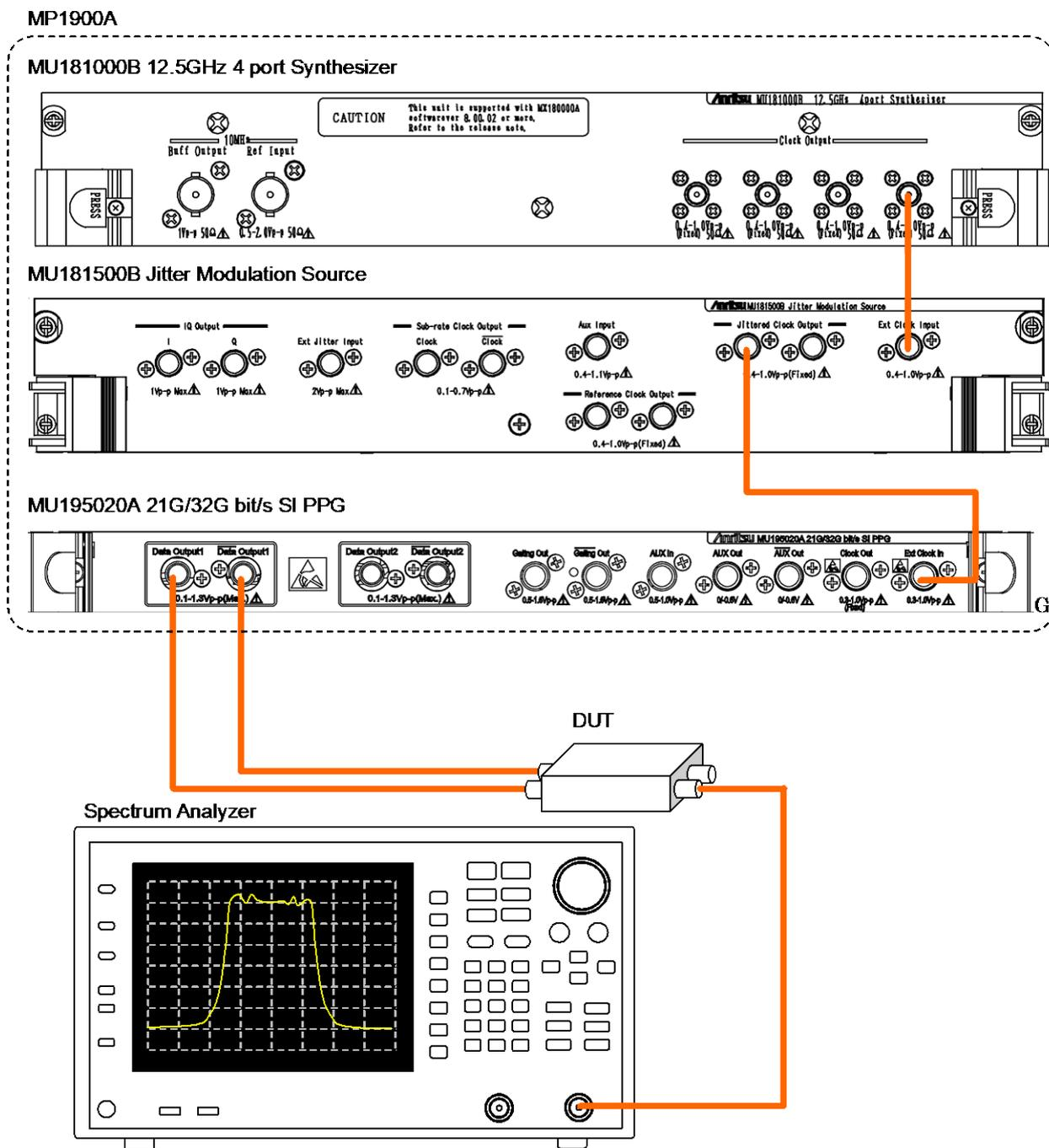
Figure 4.3-1 Spectrum Spread Measurement System Setup (USB4 SSC Profile)
