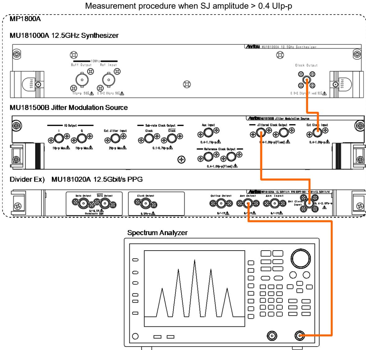
Figure 6.3.1-3 Setup when SJ Amplitude > 0.4 UIp-p
