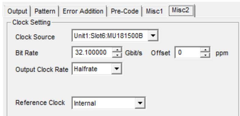
**Figure 3.3.1-2 MU183020A Clock Source Settings (When Tracking Operation of Jitter and Synthesizer)**
