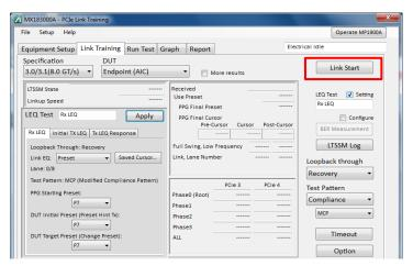
When LTSSM State is Loopback.Active.Master, click on Saved Cursor button on LEQ Test window.
