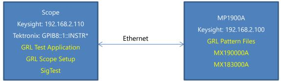
\* TCP/IP cannot be used when the GRL software is installed on a Tektronix scope. Set the GPIB address as "GPIB8::1::INSTR".
