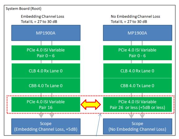
When operating with "No Embedding", the physical IL (Insertion Loss) must be added on here. If EH / EW calibration is failed, reduce the Pair number.
