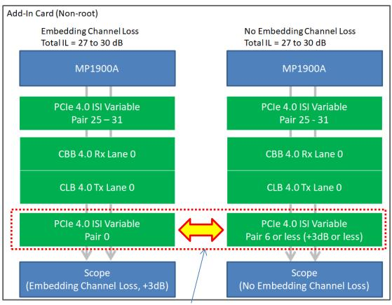
When operating with "No Embedding", the physical IL (Insertion Loss) must be added on here.
