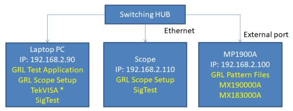
\* TekVISA is needed to control Tektronix scopes. But, the PC on which TekVISA is installed cannot control Keysight scopes. Also, this configuration makes the remote control speed slower than the recommended configuration.
