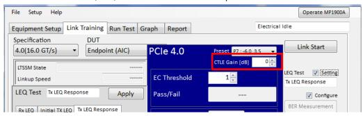
c. On the Tx LEQ Response tab of the LEQ test pane, set PPG Starting Preset to 7, DUT Initial Preset to 7 and Target Preset to P4.
