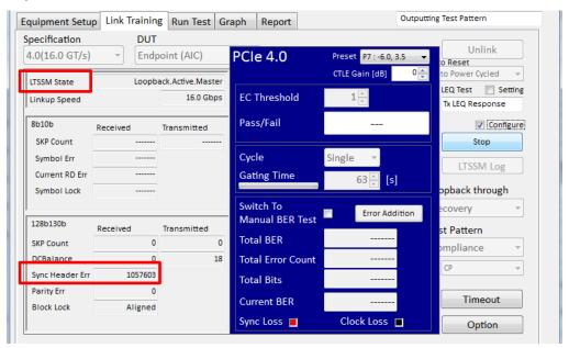
f. Increment the CTLE Gain value, and run Link Training again until Sync Header Err becomes 0 (zero) and Total Error Count becomes 0 (zero). In this case, it is considered to be error free with -6 dB.
