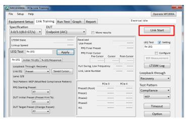
i. When LTSSM State is Loopback.Active.Master, click on Saved Cursor button on LEQ Test window.
