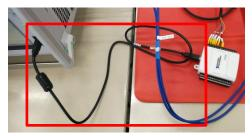
2. Connect the USB-6501 to the control pins on CBB 4.0 using cables as shown in the figure below. Always turn the CBB power switch to the OFF position when this function is used because the power supply to CBB is controlled from USB-6501.
