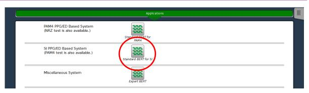
Figure 4.1.1-1 How to Start Standard BERT for SI Application
