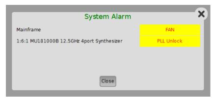
Figure 3.2.2.13-2 System Alarm Dialog Box (FAN Error and PLL Unlock Error)
