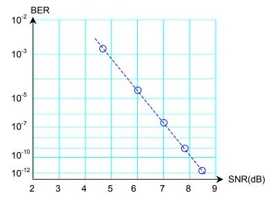
Figure 1.5-12 Relationship between SNR and BER
