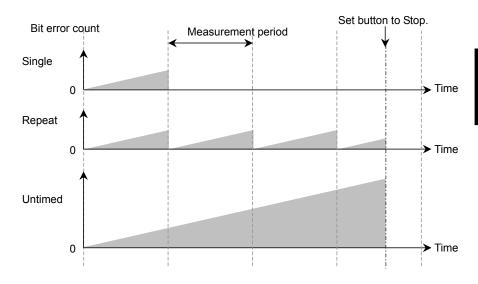
Figure 6.4-1 Gating Cycle Settings and Bit Error Count
