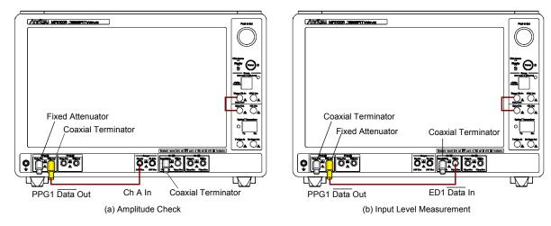
Figure 9.2.2-2 ED1 Data In Input Sensitivity Test Connection Diagram
