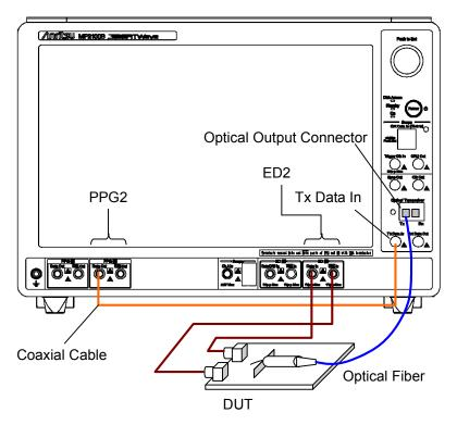
Figure 3.1-2 Connection when DUT is Optical Receiver
