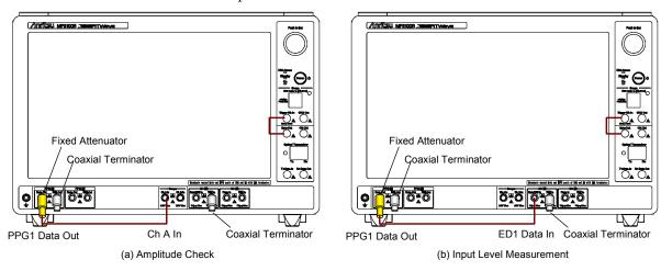
Figure 9.2.2-1 ED1 Data In Input Sensitivity Test Connection Diagram
