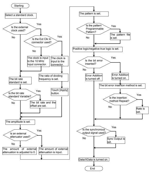
Figure 5.3-1 Basic Procedure of Generating Pulse Signal
