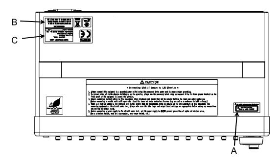
Figure 1 Locations of Labels (Top View)
