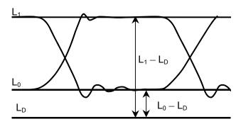
Figure 1.5-8 Extinction Ratio Measurement Level
