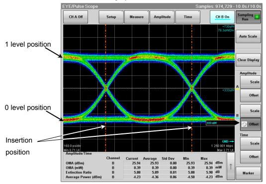
Figure 7.10.1-1 Waveform Display after Auto Scale (Eye/Pulse/Coherent Mode)
