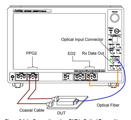
Figure 3.1-4 Connection when DUT is Optical Transmitter
