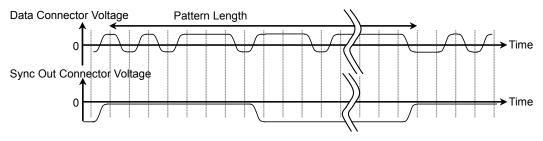
Figure 5.8-3 Voltage Waveform Output to Connector Corresponding to Sync Output
