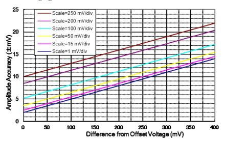
Figure 9.3.2-1 Offset Amplitude Accuracy
