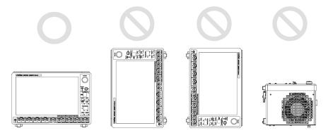
Figure 2.1.2-1 Installation Orientation
