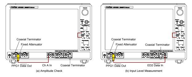
Figure 9.2.2-4 ED2 Data In Input Sensitivity Test Connection Diagram
