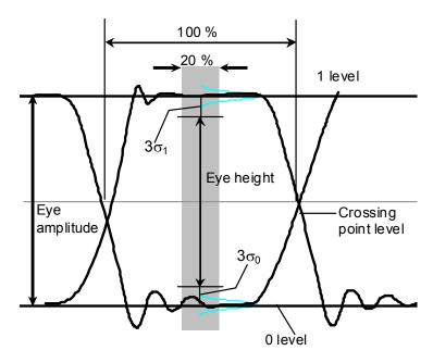
Figure 1.5-1 0 Level, 1 Level, Eye Amplitude and Eye Height
