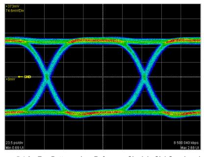
Figure 5.4-3 Eye Pattern when Reference Clock is Ch1 Synchronized
