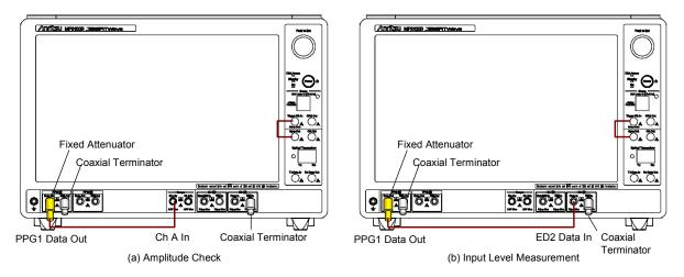
Figure 9.2.2-3 ED2 Data In Input Sensitivity Test Connection Diagram
