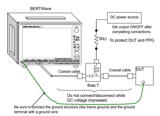
Figure 2.15.2-1 Bias-T Connection Example
