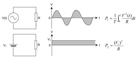
Figure 1.5-2 AC and DC Voltage Power Consumption
