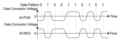
Figure 5.6-2 Relationship between Logic Setting and Output Voltage Waveform at Connector
