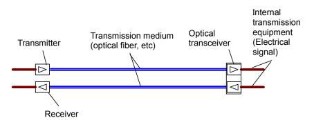
Figure 1.4-1 Uses of Receiver and Transmitter
