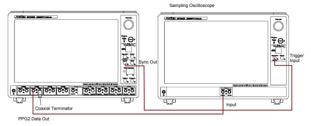
Figure 9.1.3-3 PPG2 Data Out Waveform Test Connection Diagram
