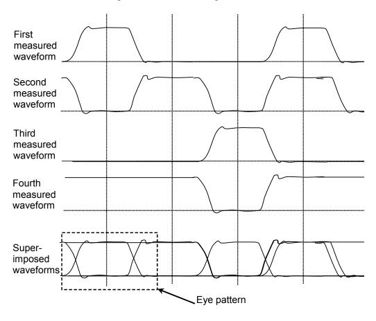
Figure 1.5-3 Eye Pattern Drawing Method
