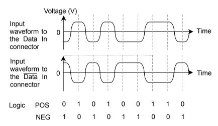
Figure 6.3-3 Values Defined as Input Waveform
