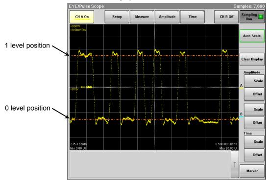
Figure 7.10.1-2 Waveform Display after Auto Scale (Pulse Mode)
