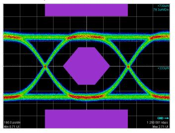
Figure 1.1-1 Mask Test Waveform
