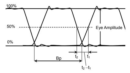
Figure 1.5-9 Duty Cycle Distortion
