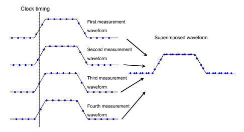
Figure 1.5-6 Drawing Method of Sampling Oscilloscope
