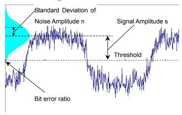
Figure 1.5-11 Bit Error Rate
