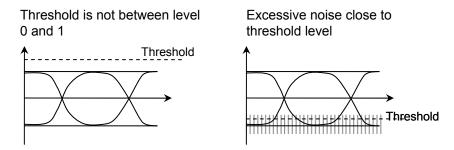
Figure 6.4-2 Examples of Improper Thresholds
