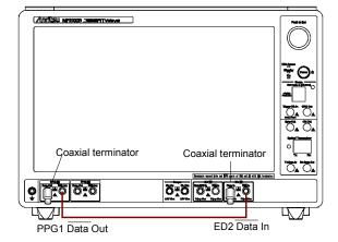
Figure 9.2.4-4 ED2 Data In Pattern Test Connection Diagram
