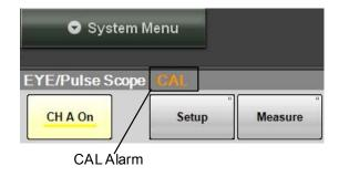
Figure 7.5.1-3 CAL Alarm Display
