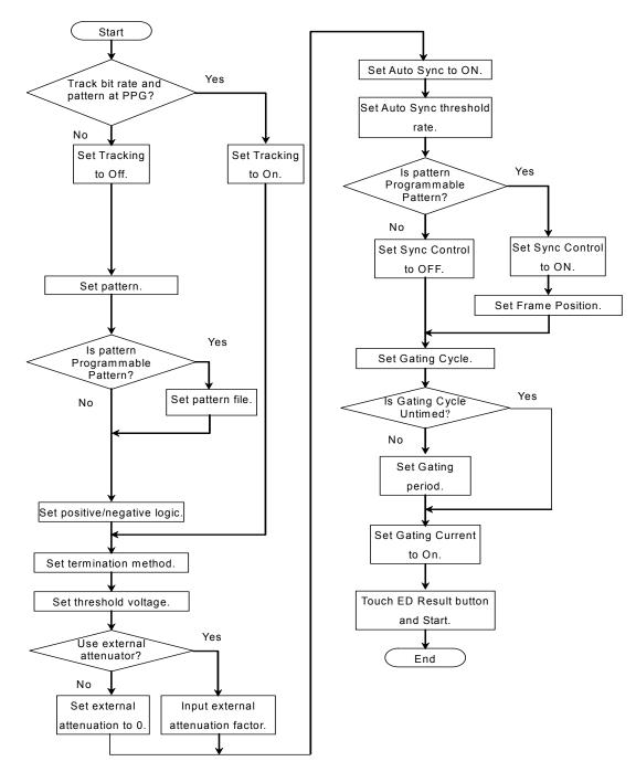
Figure 6.2-1 Basic Procedure of Bit Error Rate Measurement
