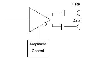
Figure 5.5-1 Output Terminal Block Diagram
