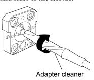
3. Press the tip of a new (dry) adapter cleaner into the ferrule end surface and then wipe in one direction 2 or 3 times to dry the surface.
