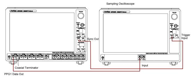
Figure 9.1.3-1 PPG1 Data Out Waveform Test Connection Diagram
