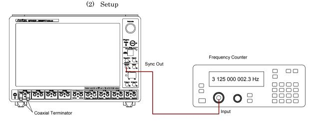
Figure 9.1.2-1 Operation Frequency Range Test Setup
