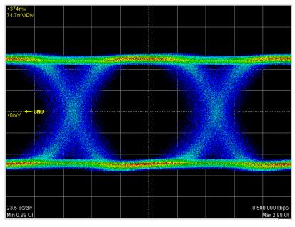
Figure 5.4-2 Eye Pattern when Reference Clock is Internal
