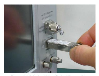
Figure 2.8.1-1 Installing Optical Transceiver
