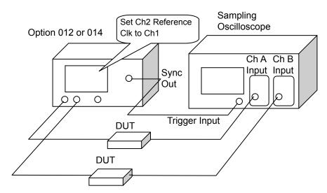
Figure 5.4-4 Setup for Simultaneous Monitoring of Two Channels
