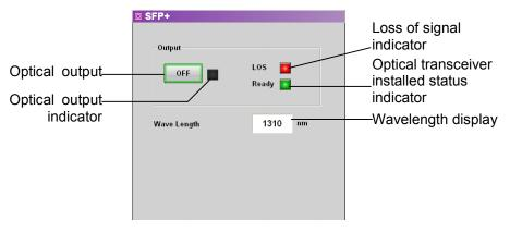
Figure 8.2.1-1 Optical Transceiver Setting Panel (SFP+)
