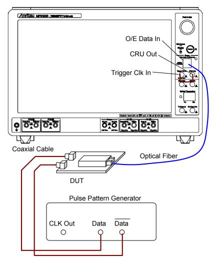
Figure 3.2-3 Optical Transceiver Used as DUT (Option 023,054)
