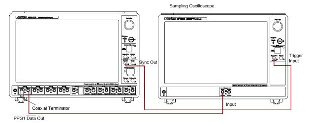
Figure 9.1.3-2 PPG1 Data Out Waveform Test Connection Diagram
