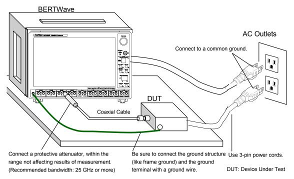
Figure 2.15.1-1 Example of Connection with DUT
