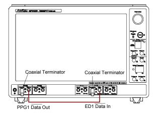
Figure 9.2.4-2 ED1 Data In Pattern Test Connection Diagram
