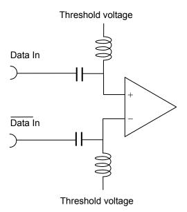
Figure 6.3-1 Input Terminal Block Diagram
