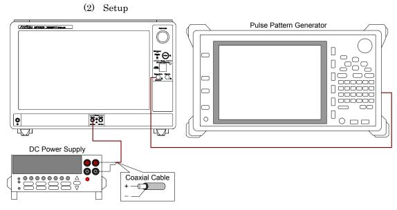
Figure 9.3.2-2 Amplitude Accuracy Test Connection Diagram
