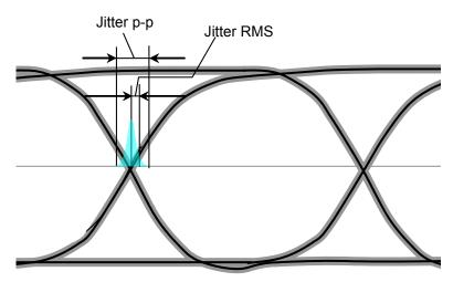
Figure 1.5-7 Jitter p-p and Jitter RMS
