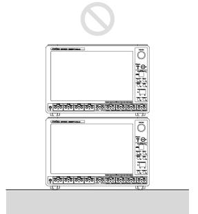
Figure 2.1.2-2 Prohibited Installation—Stacking
