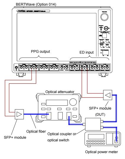
Figure 1.4-4 Receiver Test Method
