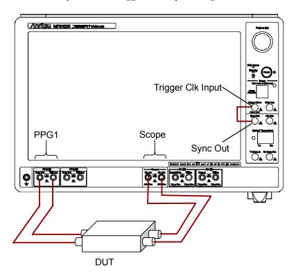
Figure 3.2-1 Electrical Signal Used for DUT Input/Output (Option 021)
