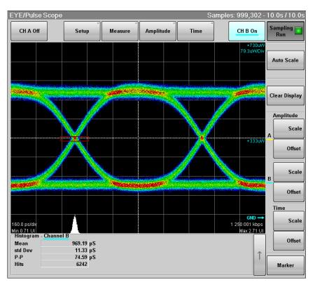
Figure 7.11.2-3 Histogram Measurement Example (Time)
