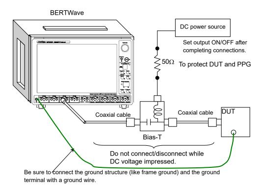
Figure 2.15.2-1 Bias-T Connection Example
