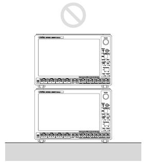
Figure 2.1.2-2 Prohibited Installation—Stacking
