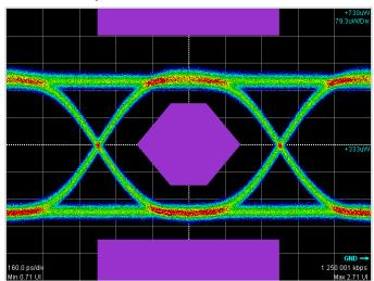
Figure 1.1-1 Mask Test Waveform
