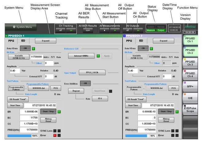
Figure 4.1-1 Names of Application Screen Elements
