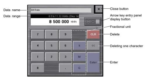
Figure 4.2-2 Numeric Value Entry Panel
