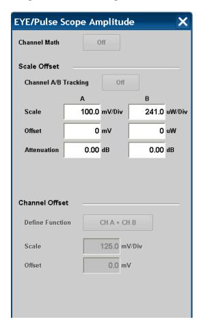
Figure 7.1.2-5 Amplitude Dialog Box (Optical/Single End Electrical Receiver)
