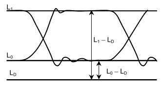
Figure 1.5-8 Extinction Ratio Measurement Level
