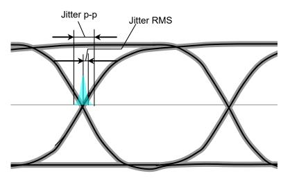
Figure 1.5-7 Jitter p-p and Jitter RMS
