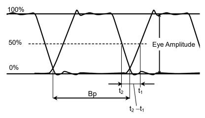
Figure 1.5-9 Duty Cycle Distortion
