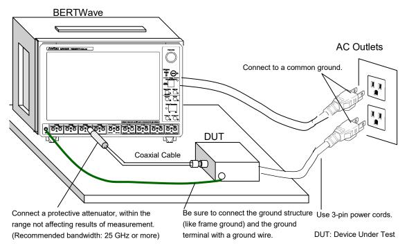
Figure 2.15.1-1 Example of Connection with DUT
