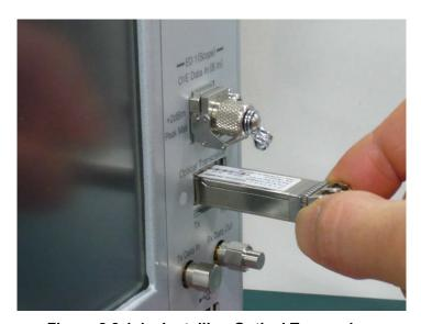
Figure 2.8.1-1 Installing Optical Transceiver
