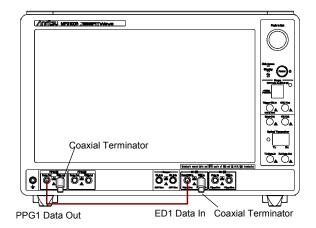
Figure 9.2.4-1 ED1 Data In Pattern Test Connection Diagram
