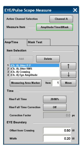
Figure 7.11.1-1 Setting Example of Amplitude/Time Measurement
