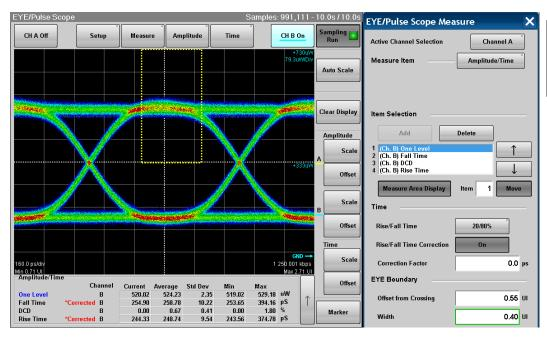
Figure 7.11.1-5 Display Example of Measurement Result
