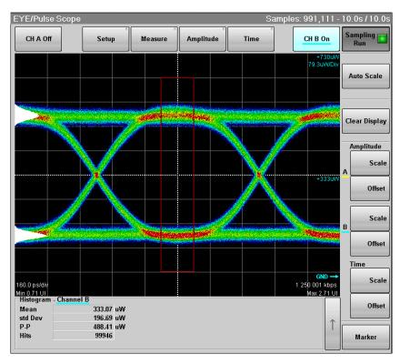
Figure 7.11.2-2 Histogram Measurement Example (Amplitude)
