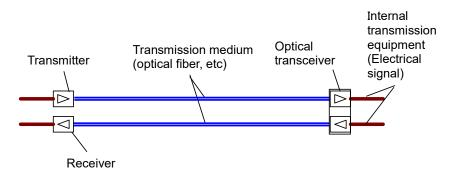
Figure 1.4-1 Uses of Receiver and Transmitter
