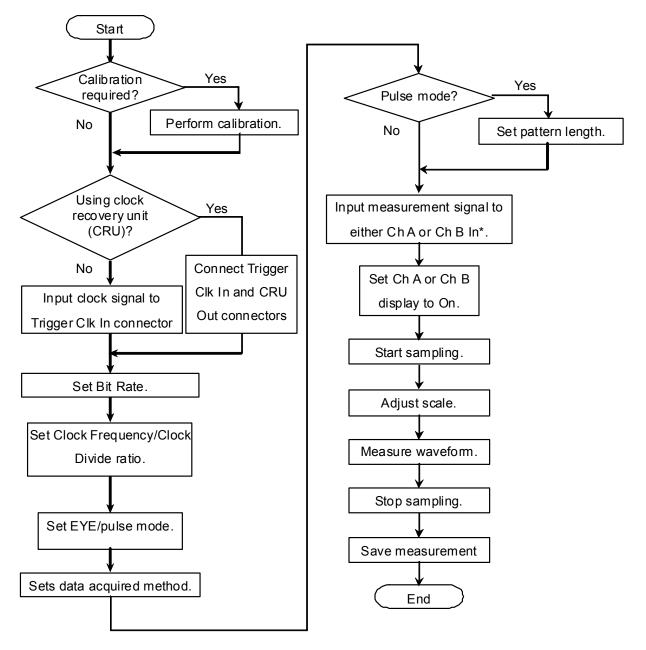
Figure 7.4-1 Basic Measurement Procedures
