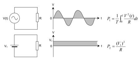
Figure 1.5-2 AC and DC Voltage Power Consumption
