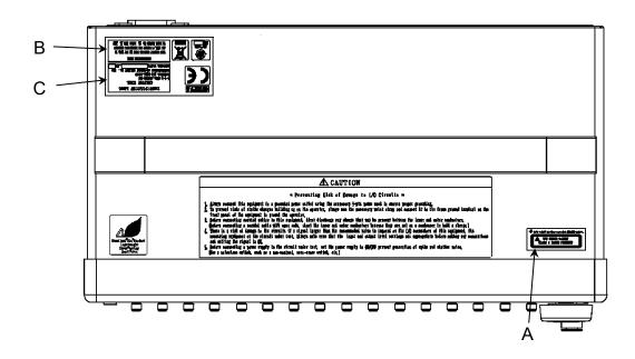
Figure 1 Locations of Labels (Top View)
