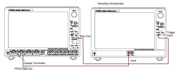
Figure 9.1.3-4 PPG2 Data Out Waveform Test Connection Diagram
