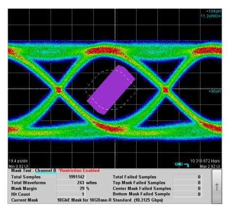
Figure 7.11.3-4 Example of Area Limited Mask Test
