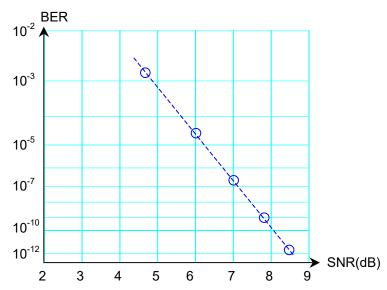
Figure 1.5-12 Relationship between SNR and BER
