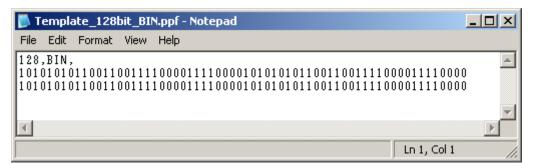
Figure D.1-2 Example of Pattern File Described by Binary Number
