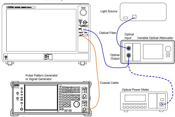
Figure 9.4.2-1 Optical Power Meter Test Connection Diagram (Option 023)
