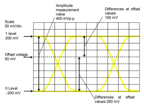
In this example, the difference between 1 level voltage (200 mV) and offset voltage (50 mV) is 150 mV. At a scale of 50 mV/div for a voltage difference of 150 mV, the amplitude accuracy is 8 mV. At 1 level accuracy, the difference is calculated as follows:
