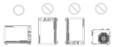
Figure 2.1.2-1 Installation Orientation
