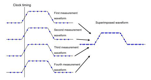
Figure 1.5-6 Drawing Method of Sampling Oscilloscope
