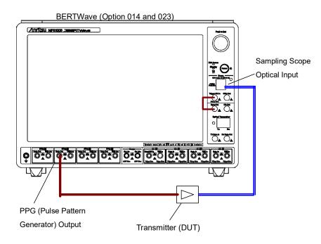
Figure 1.4-3 Transmitter Test Method
