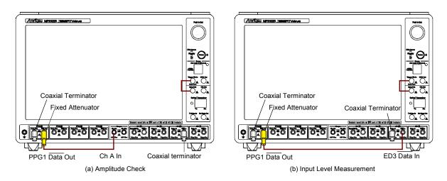
Figure 9.2.2-6 ED3 Data In Input Sensitivity Test Connection Diagram
