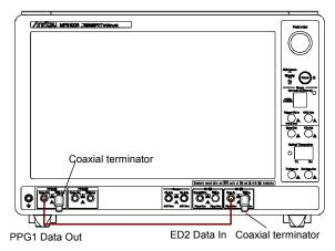
Figure 9.2.4-3 ED2 Data In Pattern Test Connection Diagram
