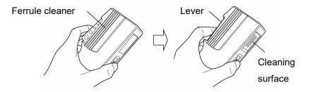
2. Hold the lever in the opened position, press the optical connector ferrule end into the cleaning surface, and then rub in one direction as shown in the following figure.
