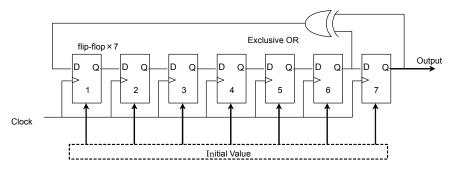
Figure 5.6-1 Block Diagram for PRBS Generating Circuit
