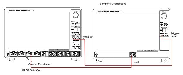
Figure 9.1.3-6 PPG3 Data Out Waveform Test Connection Diagram
