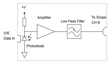
Figure 8.1-1 O/E Converter Block Diagram
