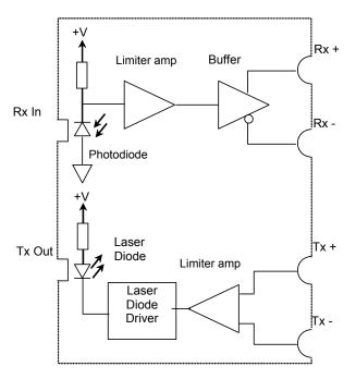
Figure 8.1-2 Optical Transceiver Block Diagram
