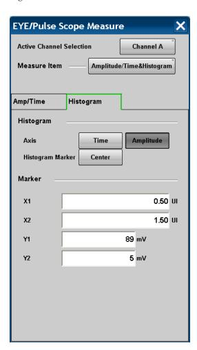
Figure 7.11.2-1 Setting Example of Histogram Measurement
