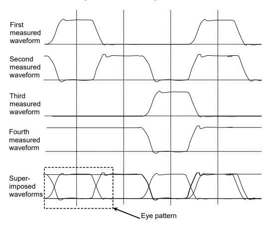
Figure 1.5-3 Eye Pattern Drawing Method
