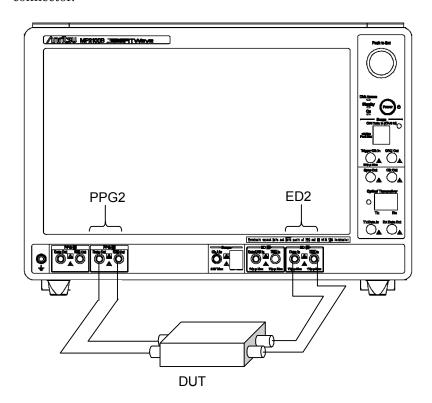
Figure 3.1-1 Making Connections Using Electrical Signal
