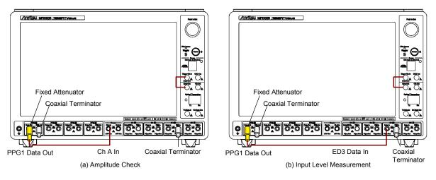
Figure 9.2.2-5 ED3 Data In Input Sensitivity Test Connection Diagram
