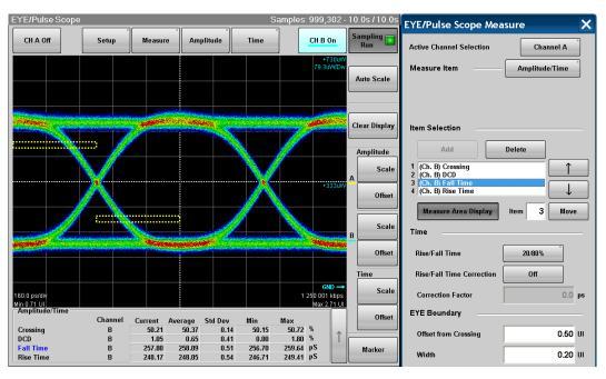
Figure 7.11.1-2 Display Example of EYE Boundary
