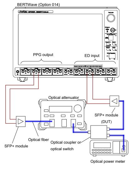
Figure 1.4-4 Receiver Test Method
