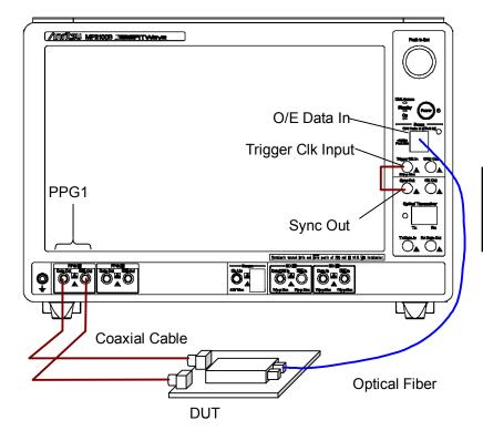
Figure 3.2-2 Optical Transceiver Used as DUT (Option 012, 023)
