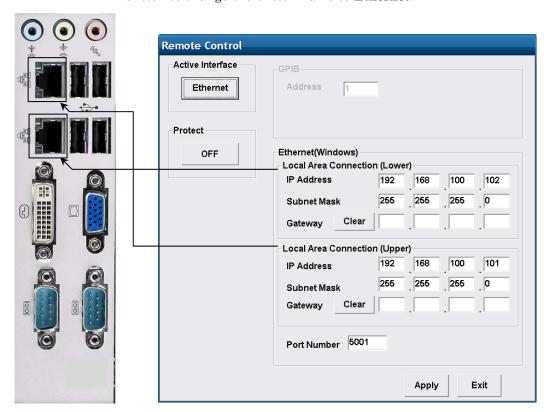
2. Set the IP address, Subnet Mask and Gateway for the Ethernet connector.
