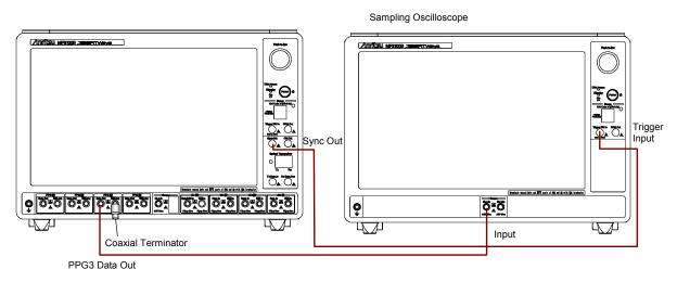
Figure 9.1.3-5 PPG3 Data Out Waveform Test Connection Diagram
