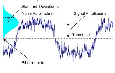
Figure 1.5-11 Bit Error Rate
