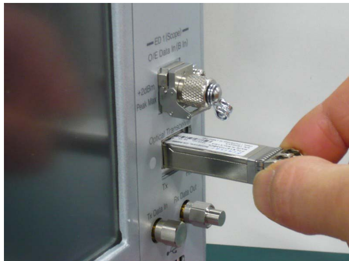
Figure 2.8.1-1 Installing Optical Transceiver
