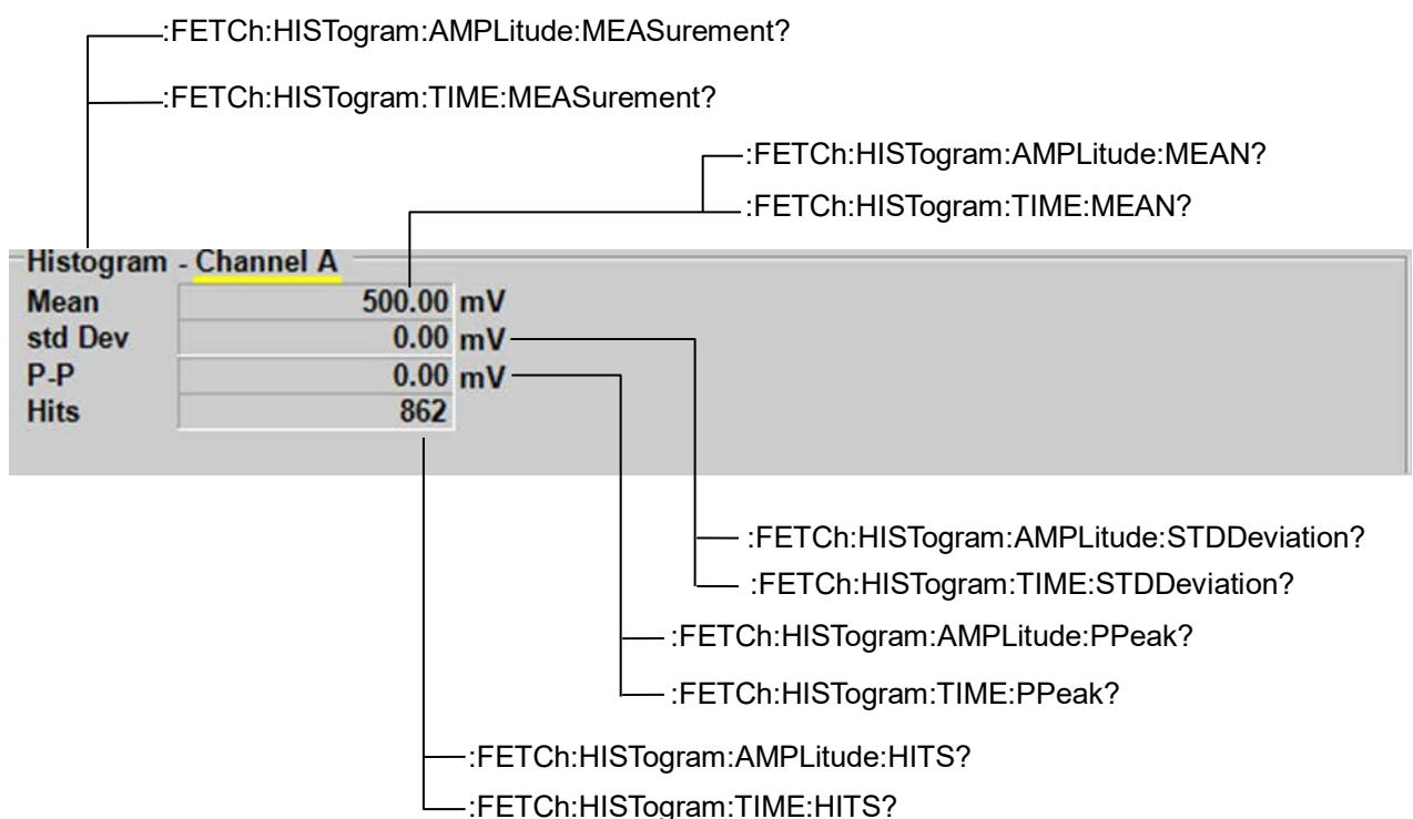
**Figure 3.2.5.1-8** Messages Corresponding to Histogram Measurement Result
