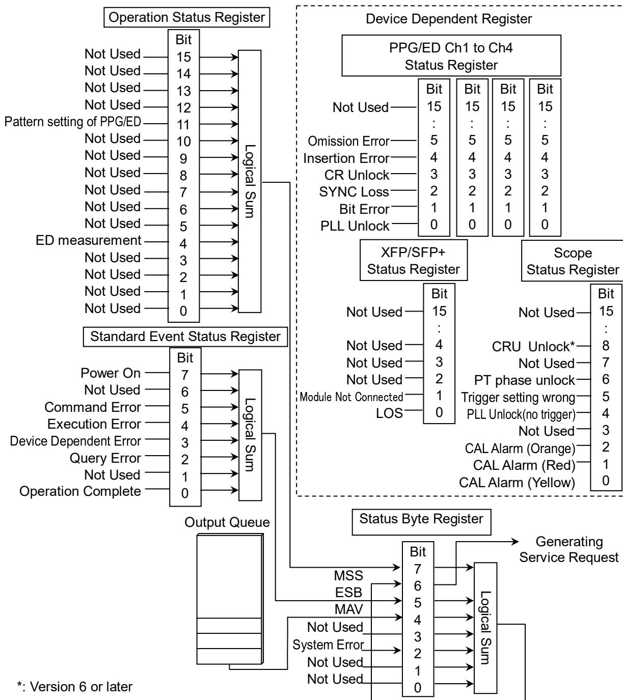
Figure 2.8.1-1 Register Structure
