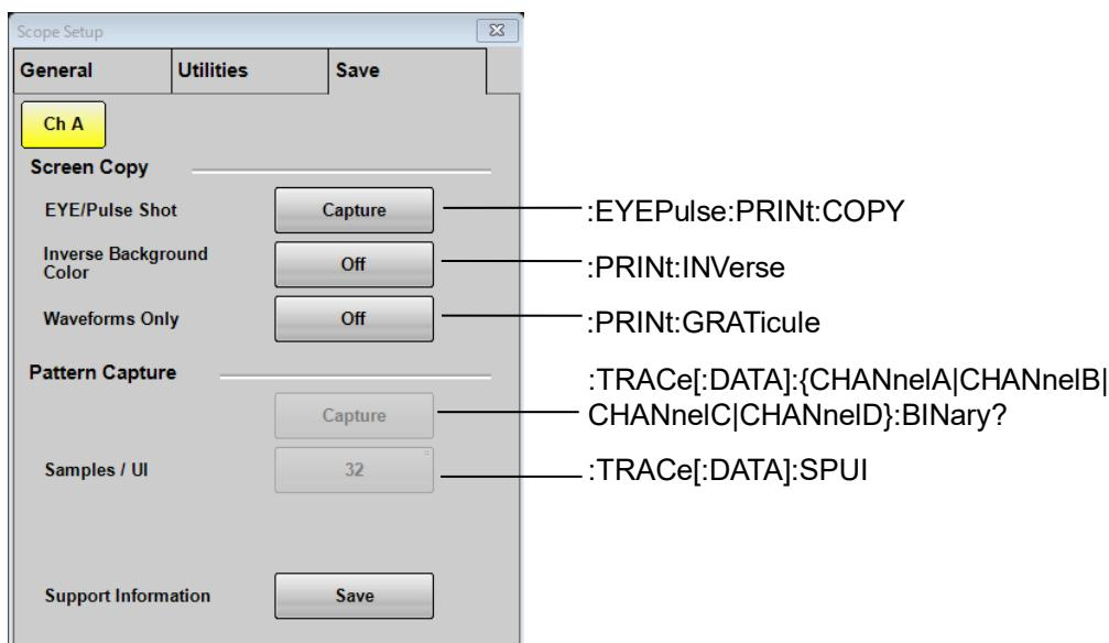
Figure 3.2.5.2-3 Messages Corresponding to Setup Dialog Box (MP2110A) (Save)
