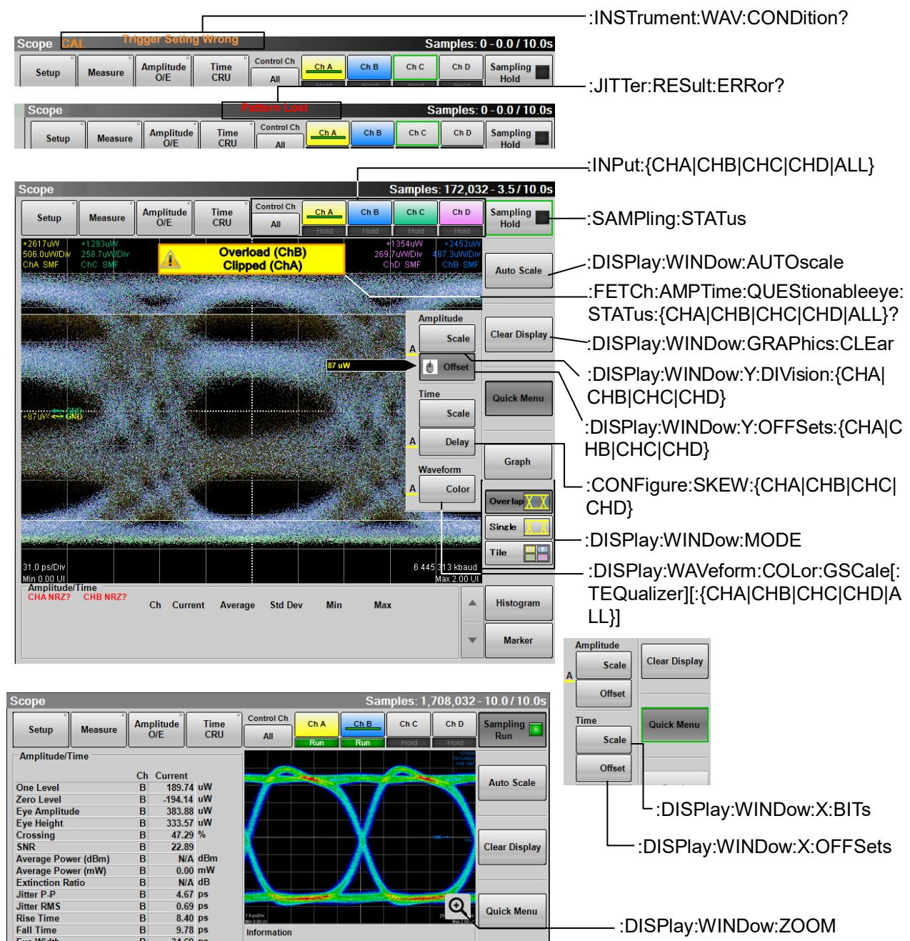
Figure 3.2.5.1-1 Messages Corresponding to Scope Panel (MP2110A)
