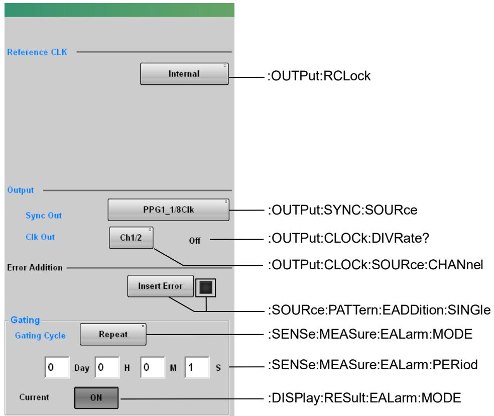
Figure 3.2.2-5 Messages Corresponding to PPG/ED Panel-2 (MP2110A)
