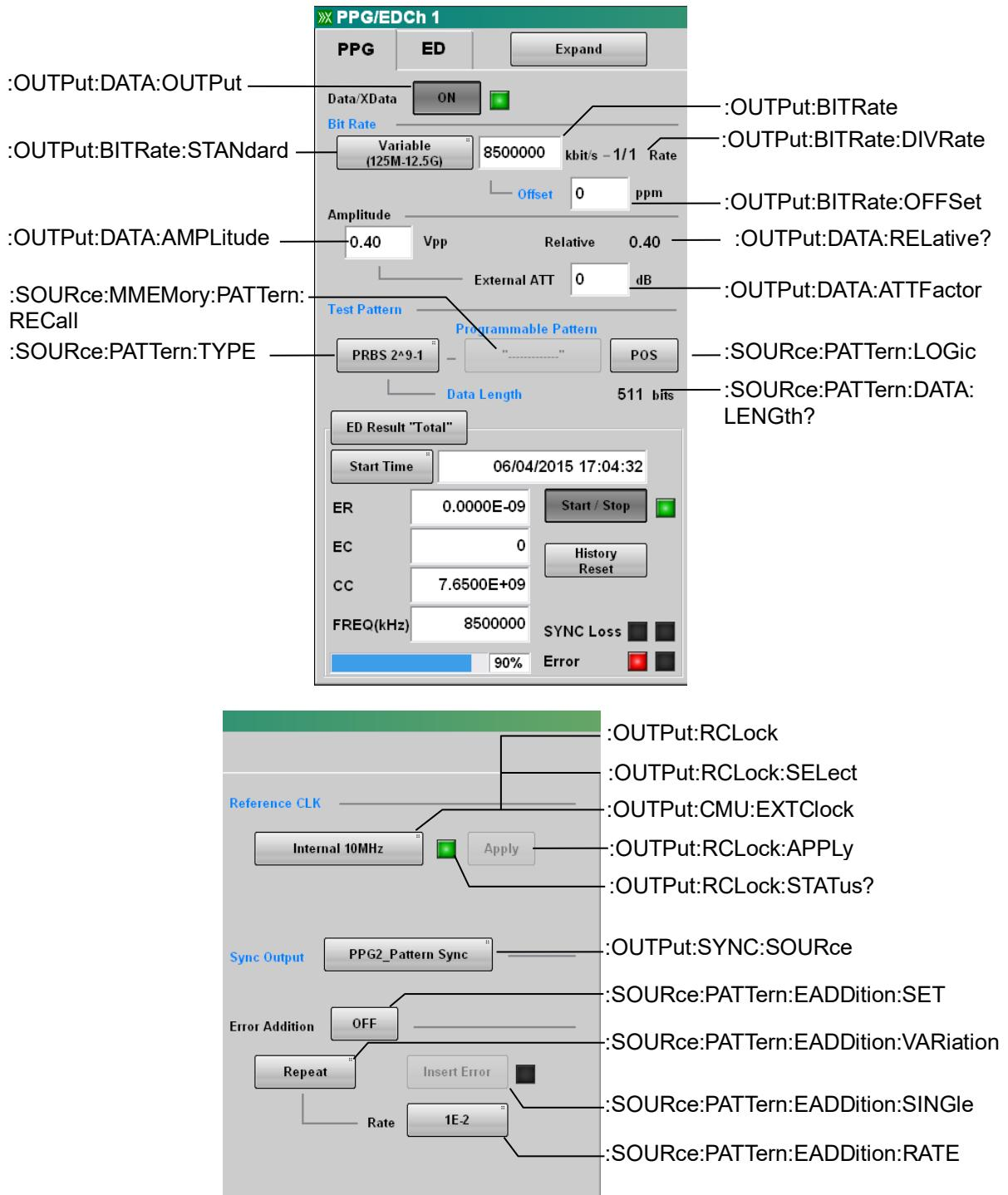
Figure 3.2.2-1 Messages Corresponding to PPG Panel (MP210xA, MP2100B)
