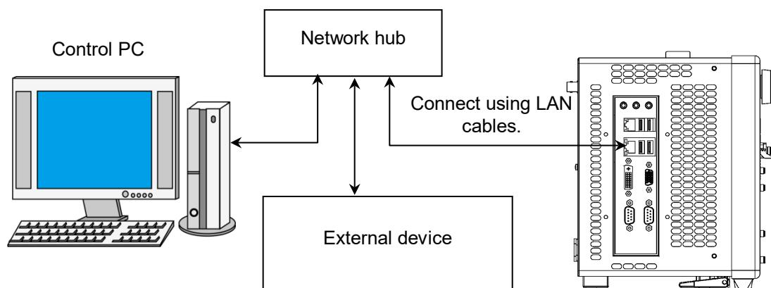
**Figure 2.4.1-2 Sample Connection with Multiple External Devices**
