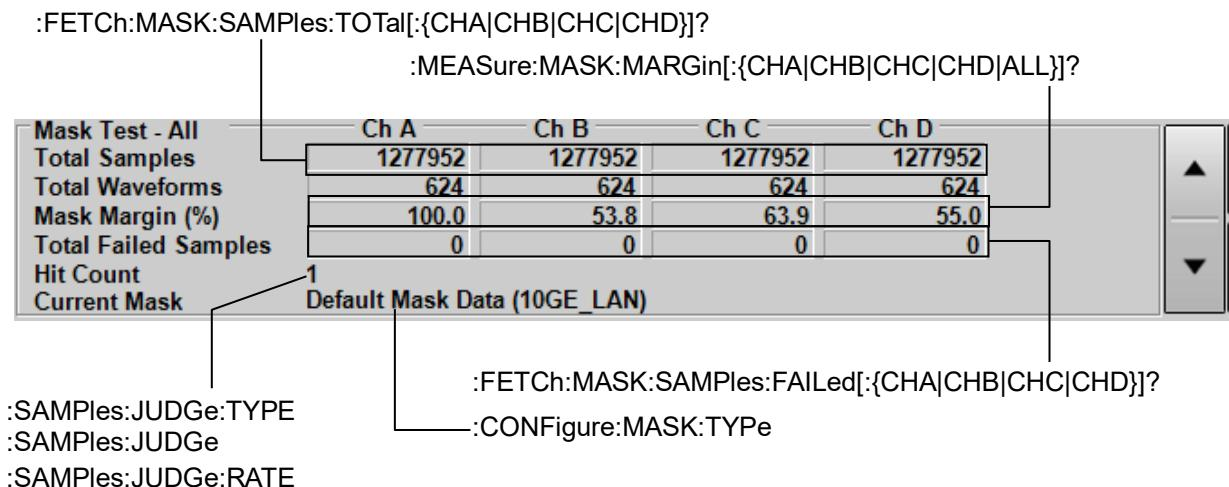
Figure 3.2.5.1-7 Messages Corresponding to Mask Test All Measurement Result (MP2110A)
