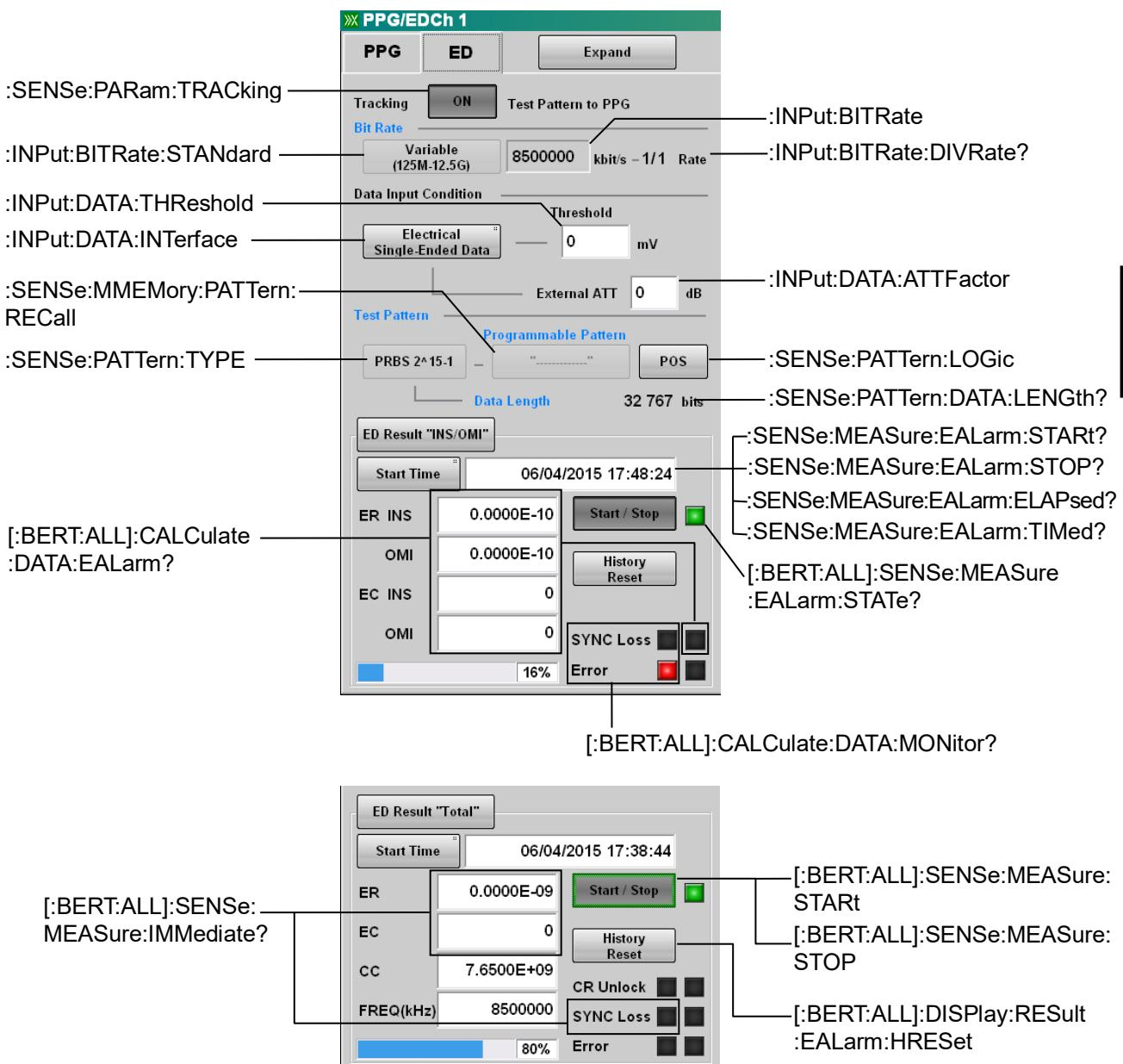
Figure 3.2.2-2 Messages Corresponding to ED Panel-1 (MP210xA, MP2100B)
