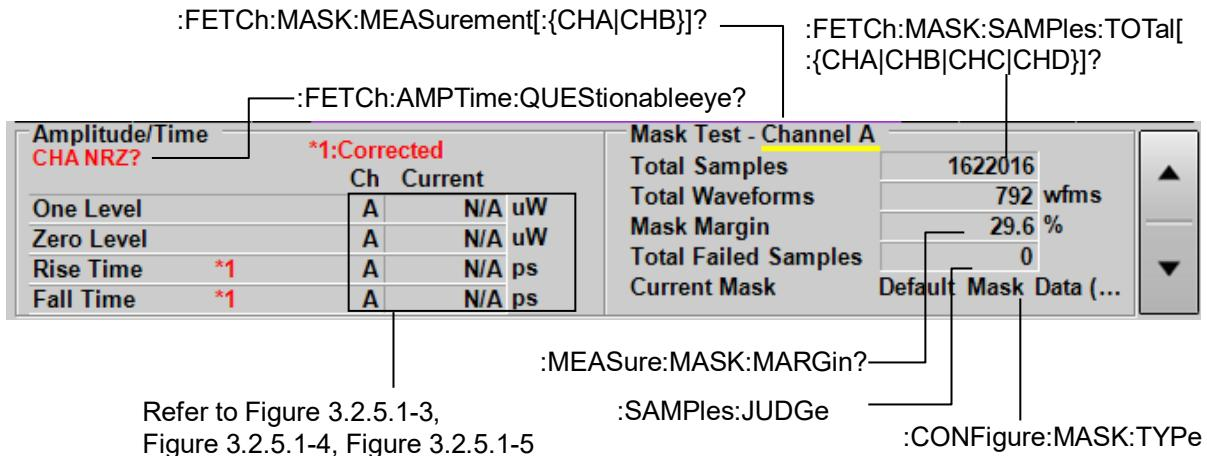
**Figure 3.2.5.1-10 Messages Corresponding to Amplitude/Time&Mask Measurement Result**
