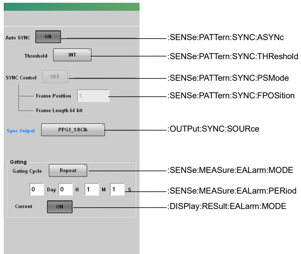
Figure 3.2.2-3 Messages Corresponding to ED Panel-2 (MP210xA, MP2100B)
