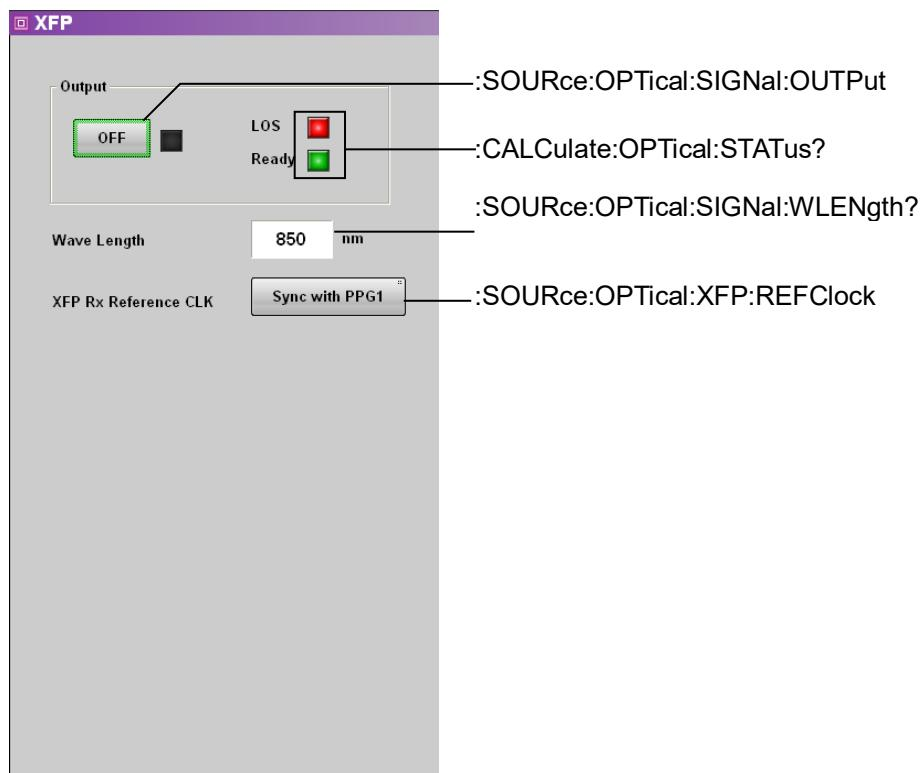
Figure 3.2.3-1 Messages Corresponding to XFP/SFP+ Panel
