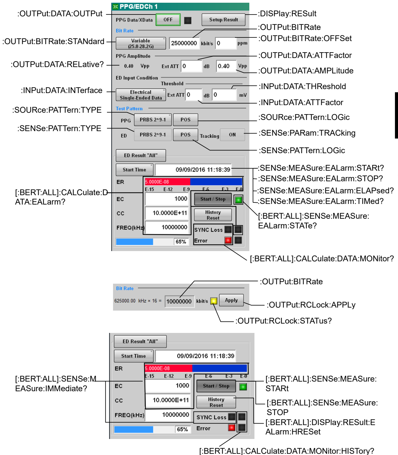
Figure 3.2.2-4 Messages Corresponding to PPG/ED Panel-1 (MP2110A)
