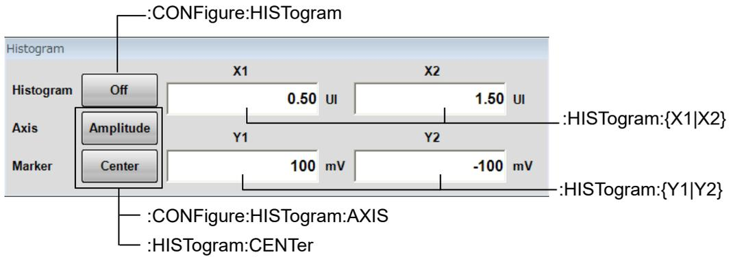
Figure 3.2.5.7-1 Messages Corresponding to Histogram Dialog Box (MP2110A)
