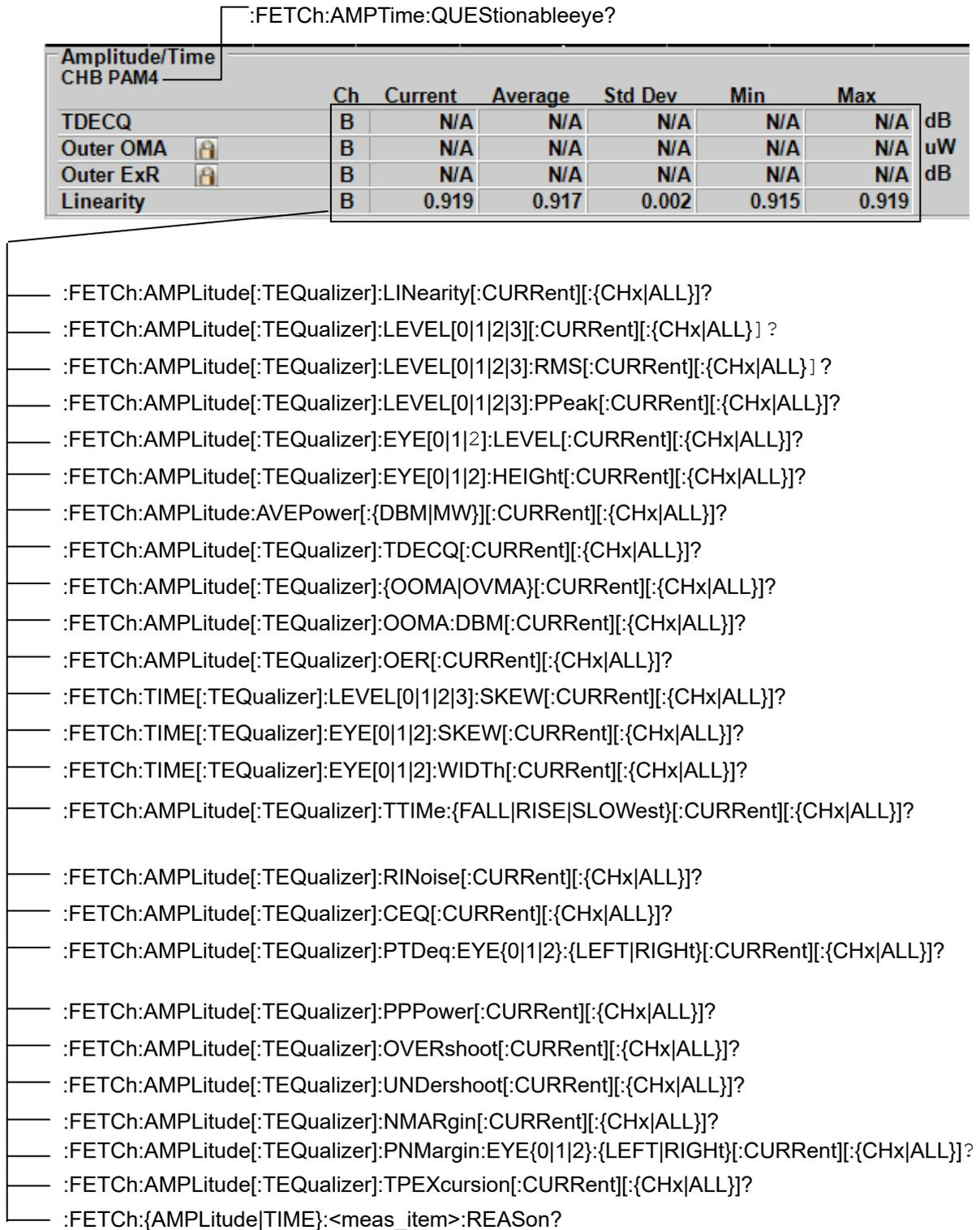
Figure 3.2.5.1-4 Messages Corresponding to Amplitude/Time Measurement Result (PAM4)
