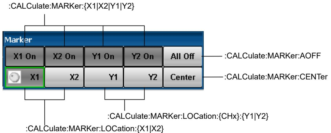
Figure 3.2.5.6-1 Messages Corresponding to Marker Dialog Box
