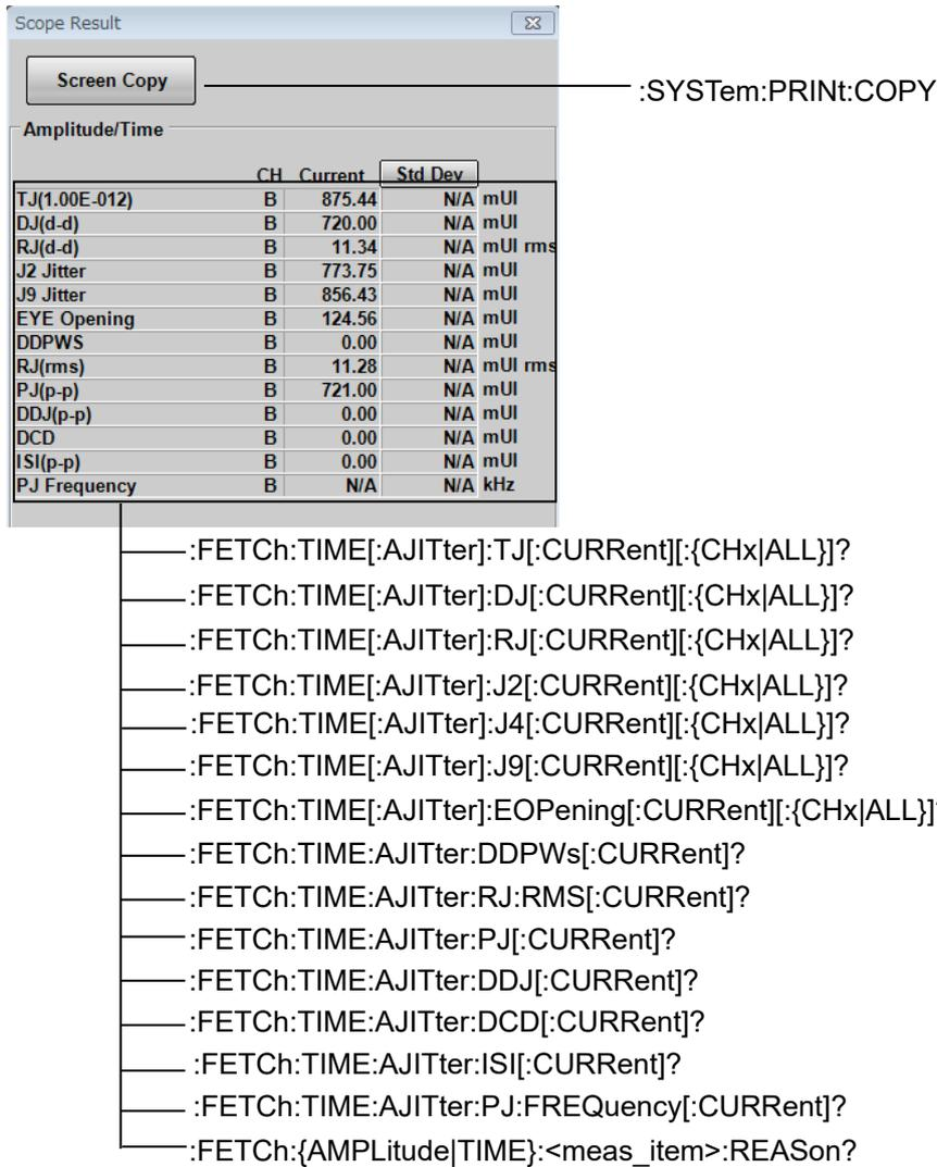
Figure 3.2.5.1-5 Messages Corresponding to Jitter Measurement Result
