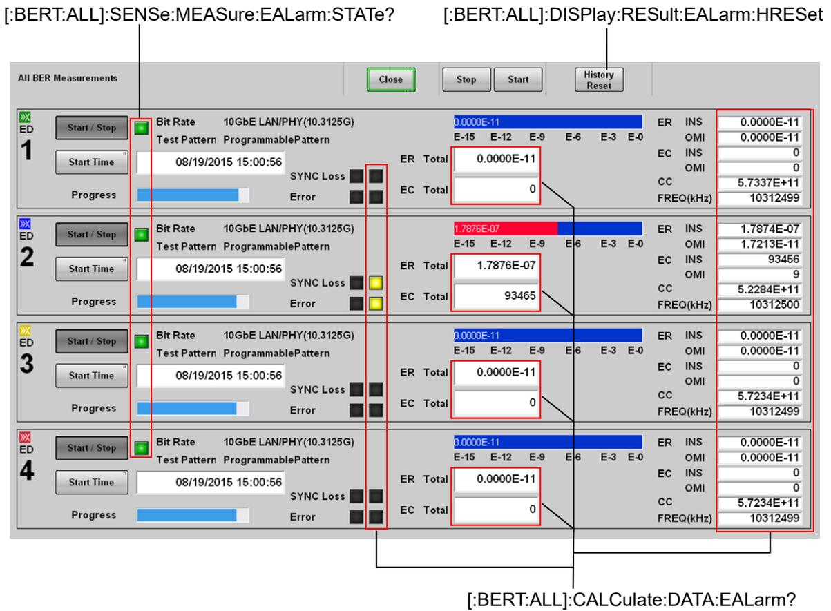
Figure 3.2.2-7 Messages Corresponding to All BER Measurement-2
