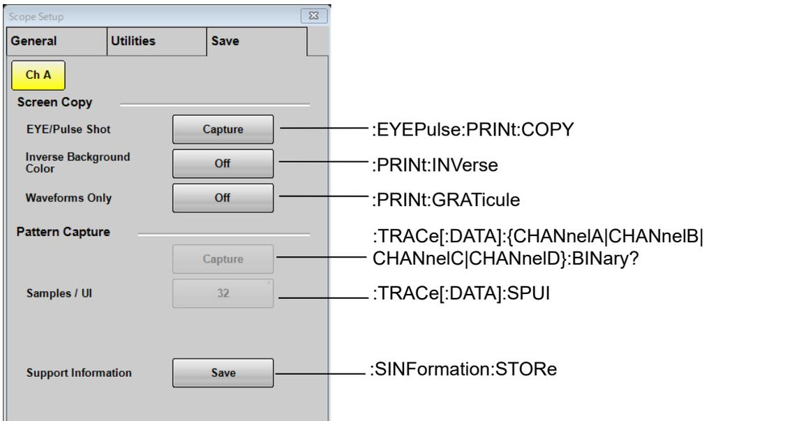
Figure 3.2.5.2-3 Messages Corresponding to Setup Dialog Box (MP2110A) (Save)
