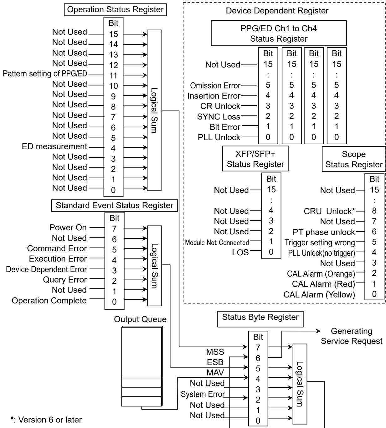
Figure 2.8.1-1 Register Structure
