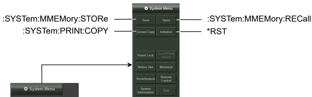
Figure 3.2.1-3 Messages Corresponding to System Menu (MP2110A)
