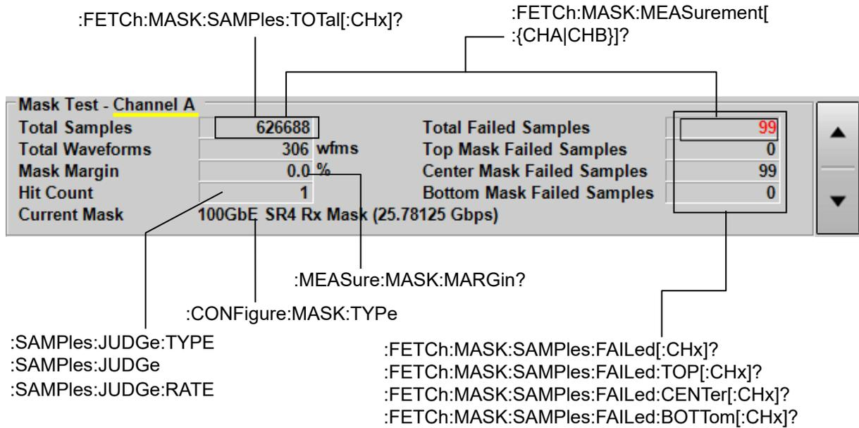
Figure 3.2.5.1-6 Messages Corresponding to Mask Test Measurement Result
