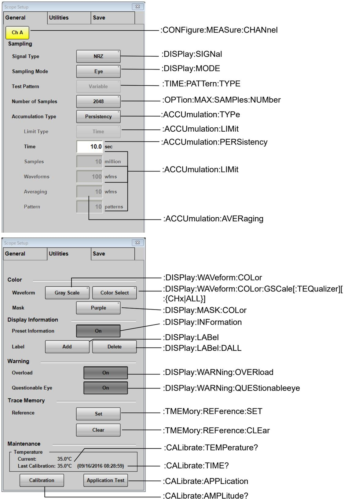
Figure 3.2.5.2-2 Messages Corresponding to Setup Dialog Box (MP2110A) (General, Utilities)
