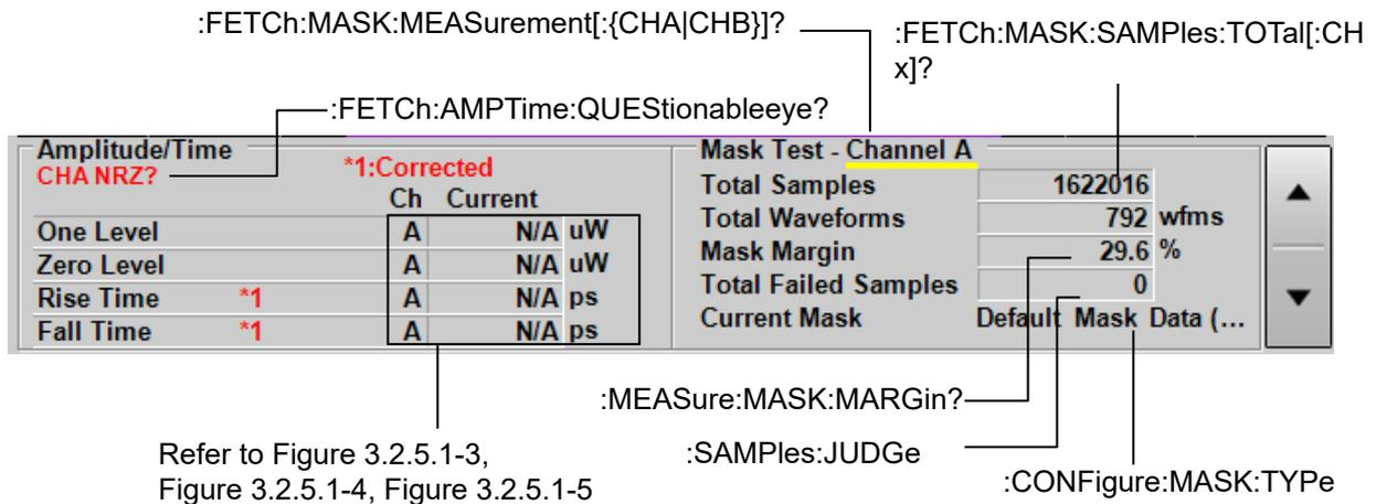
Figure 3.2.5.1-10 Messages Corresponding to Amplitude/Time&Mask Measurement Result
