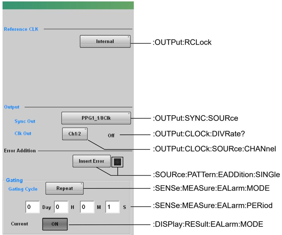
Figure 3.2.2-5 Messages Corresponding to PPG/ED Panel-2 (MP2110A)
