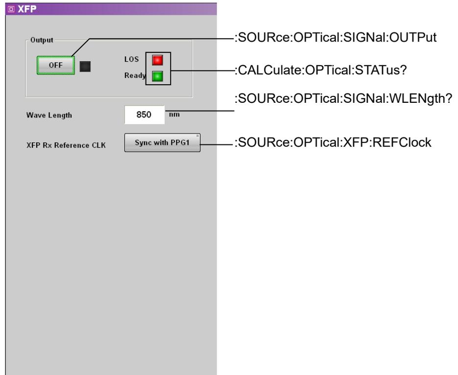
Figure 3.2.3-1 Messages Corresponding to XFP/SFP+ Panel
