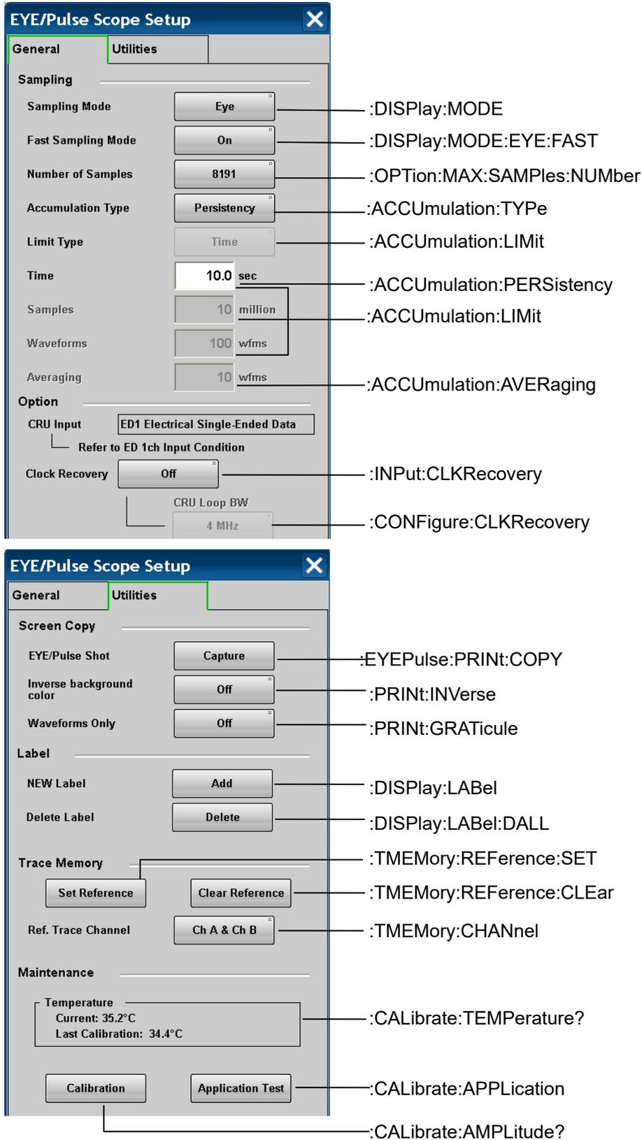
Figure 3.2.5.2-1 Messages Corresponding to Setup Dialog Box (MP210xA, MP2100B)
