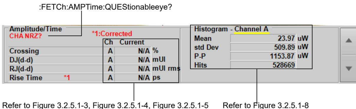
Figure 3.2.5.1-12 Messages Corresponding to Amplitude/Time&Histogram Measurement Result
