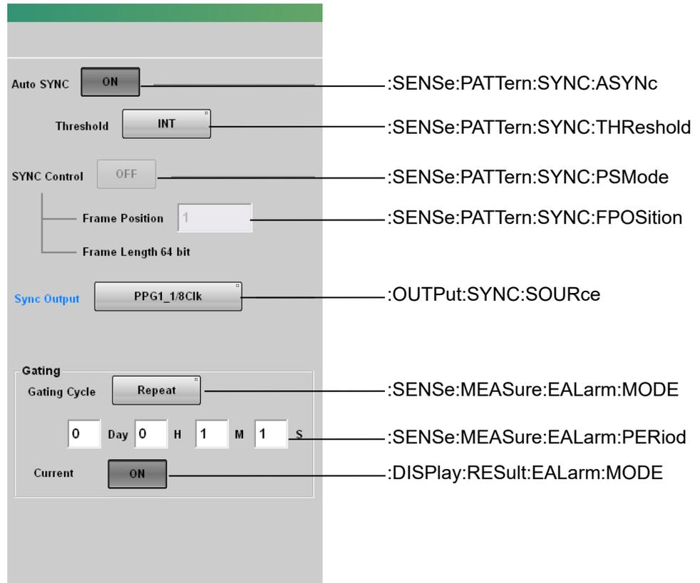
Figure 3.2.2-3 Messages Corresponding to ED Panel-2 (MP210xA, MP2100B)
