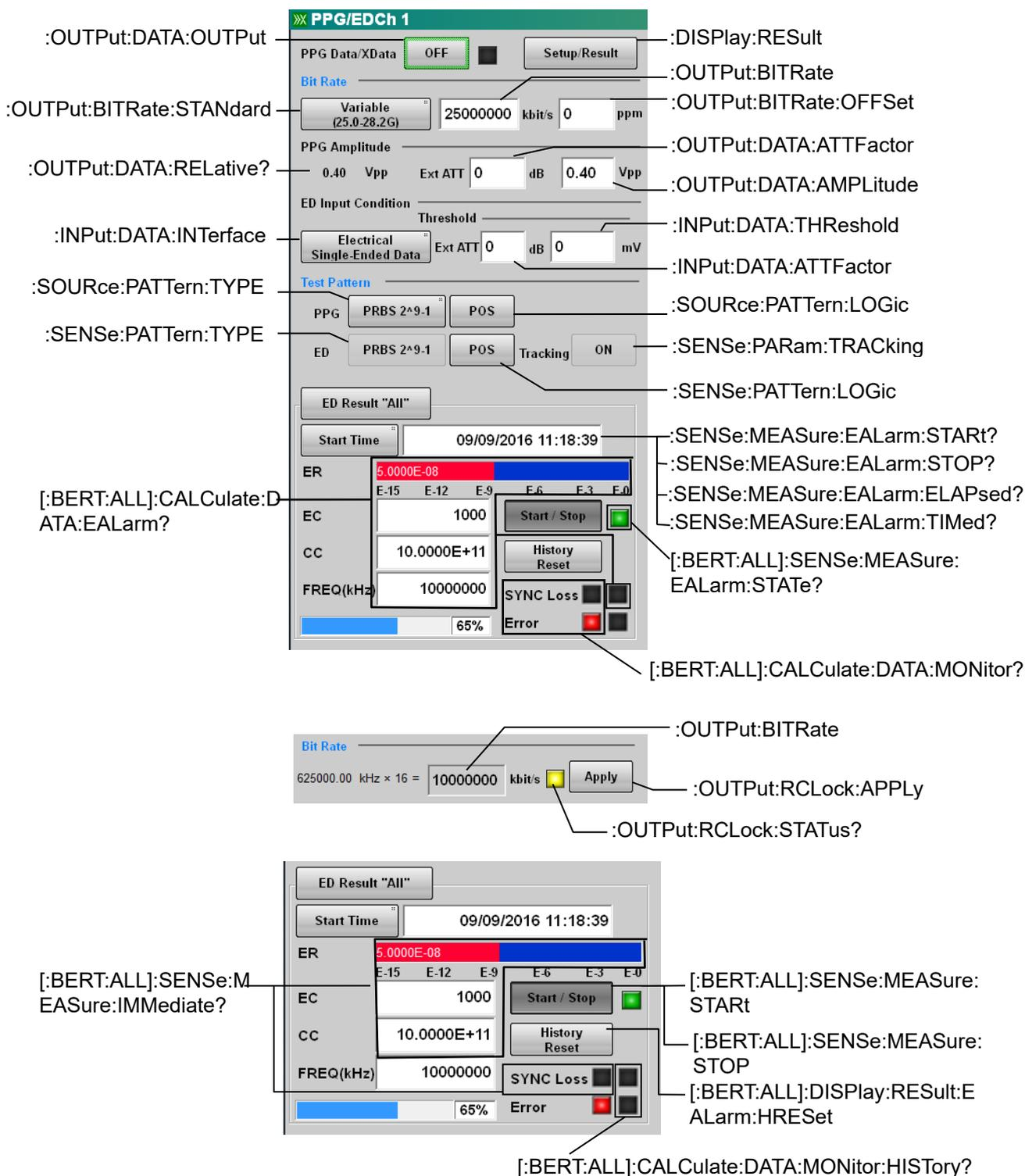
Figure 3.2.2-4 Messages Corresponding to PPG/ED Panel-1 (MP2110A)
