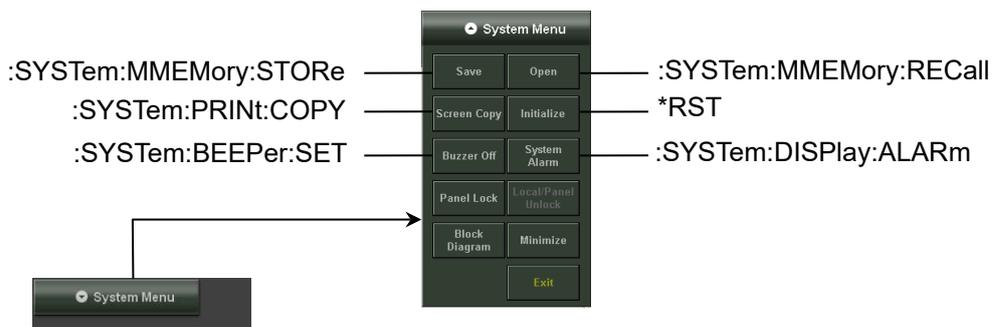
Figure 3.2.1-2 Messages Corresponding to System Menu (MP210xA, MP2100B)
