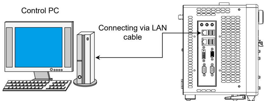
Figure 2.4.1-1 Direct Connection between BERTWave and Control PC
