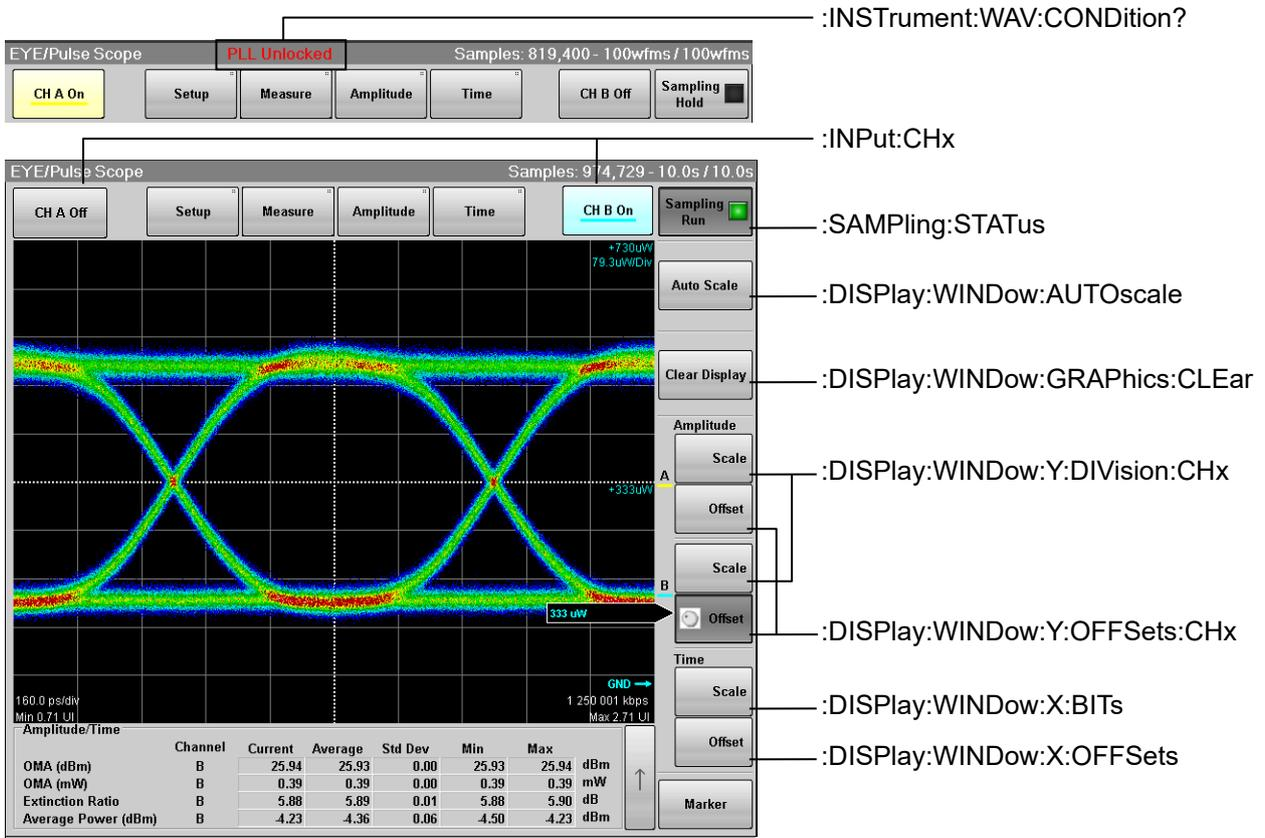
Figure 3.2.5.1-2 Messages Corresponding to Scope Panel (MP210xA, MP2100B)
