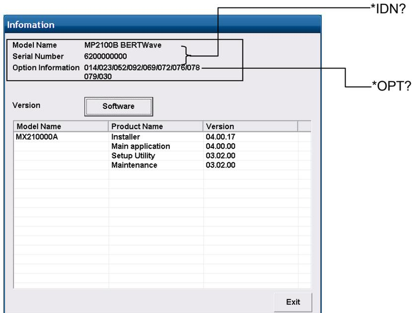
Figure 3.2.6-1 Messages Corresponding to Information Dialog Box from Setup Utility (MP210xA, MP2100B)
