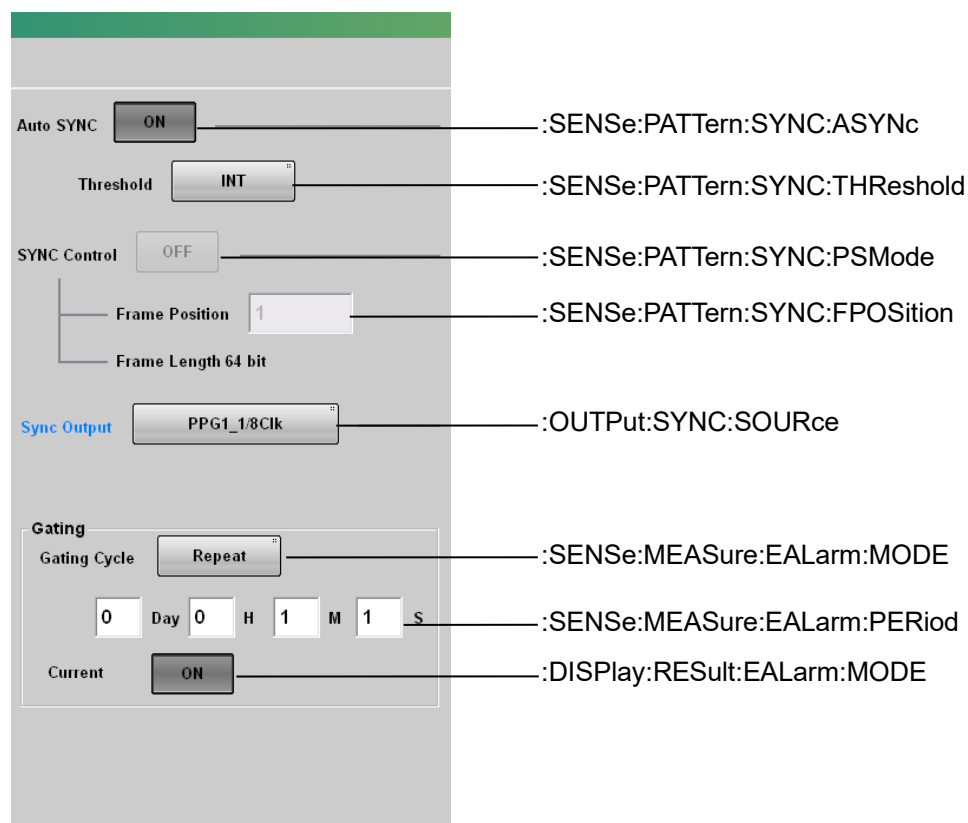
Figure 3.2.2-3 Messages Corresponding to ED Panel-2 (MP210xA, MP2100B)
