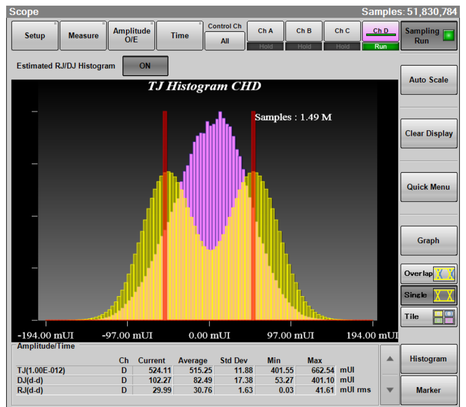
Figure 1.1.1-4 Example of Jitter Analysis
