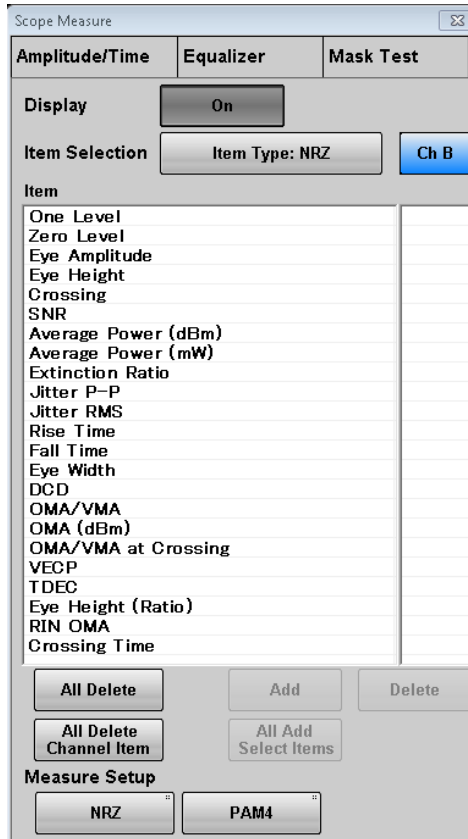
Figure 6.9.1-1 Amplitude/Time Tab When Signal Type is NRZ
