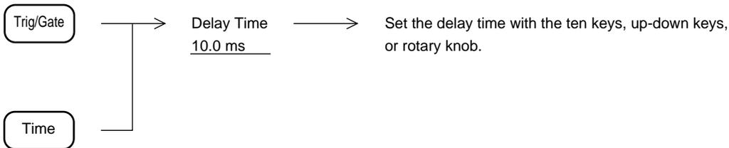
If the trigger point on the time axis on the screen was set by delay time, the trigger level indicator ► is displayed at the bottom of the screen.
