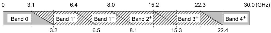
Selection of frequency bands according to range of frequencies to be observed in Auto Band mode.
