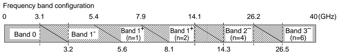
Selection of frequency bands according to range of frequencies to be observed in Auto Band mode.
