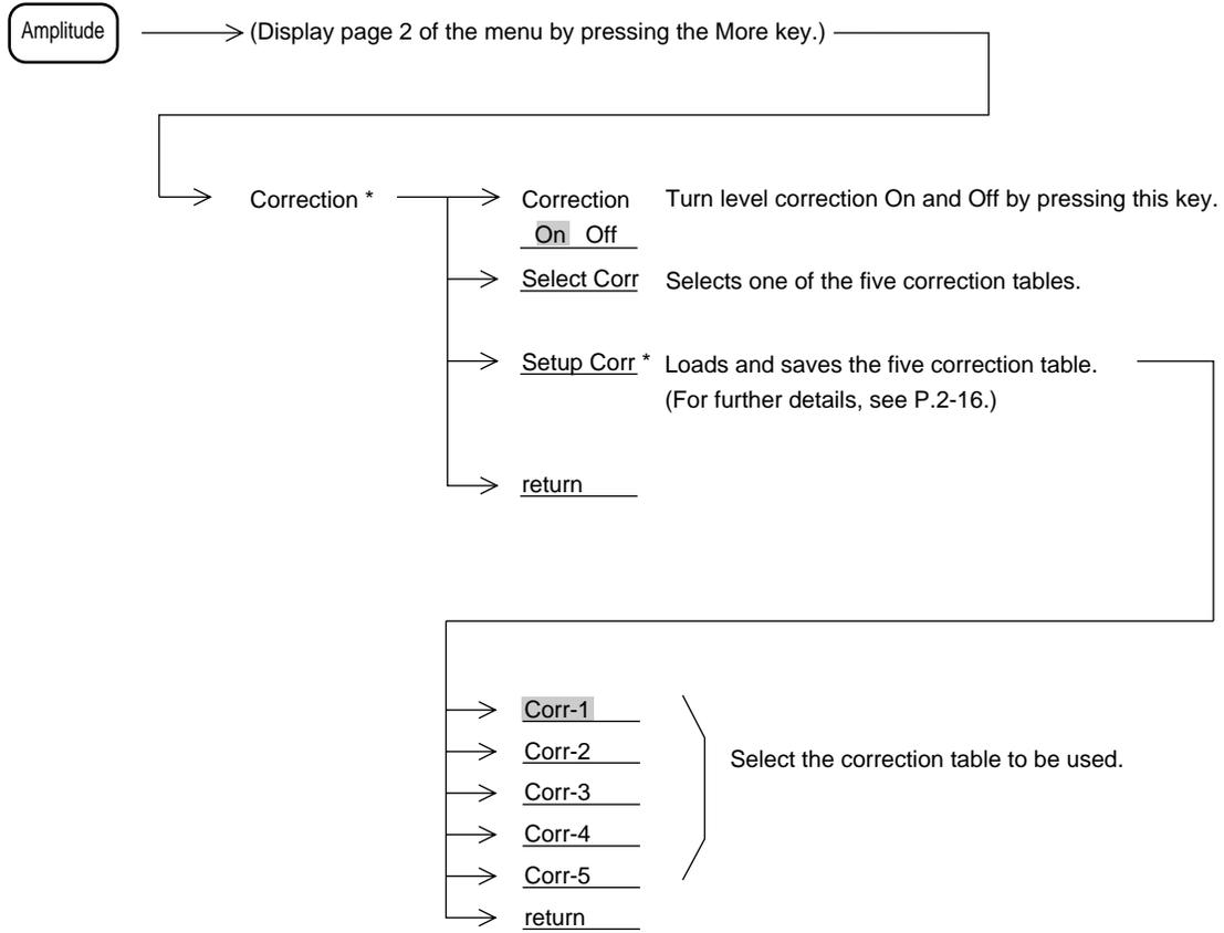
Press one of the Corr-1 to Corr-5 keys. The spectrum data is corrected and displayed by the corresponding correction value.
