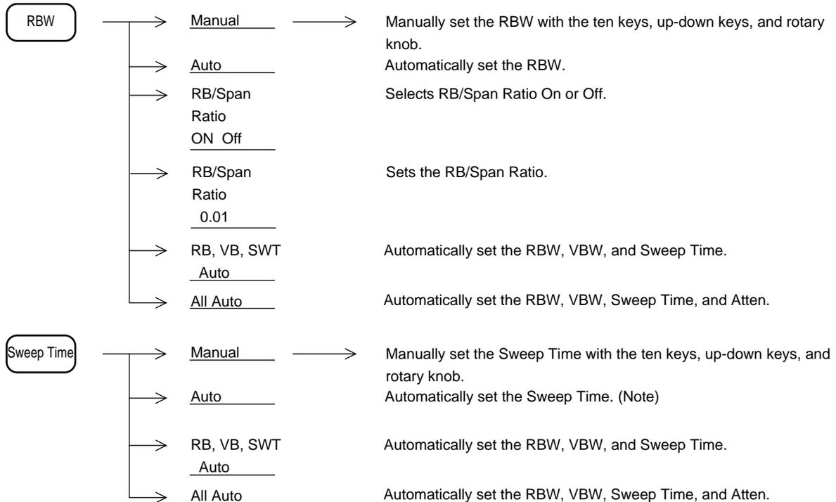
**Note:** Either of the two automatic set modes (Auto SWT: Hi-Lvl-Acc and Fast) can be selected. Normally, select the Hi-Lvl-Acc mode. See Section 9 for details.
