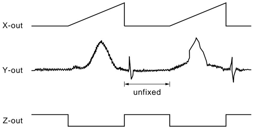
Zero Span Sweep: When trace "Time" (time axis), normally Y-out only is output, and X-out and Z-out are not output. The mode in a zero span sweep is usually set at "Digital". When X-out and Z-out signals are necessary in a zero span sweep, set the zero-span mode at "Analog".
