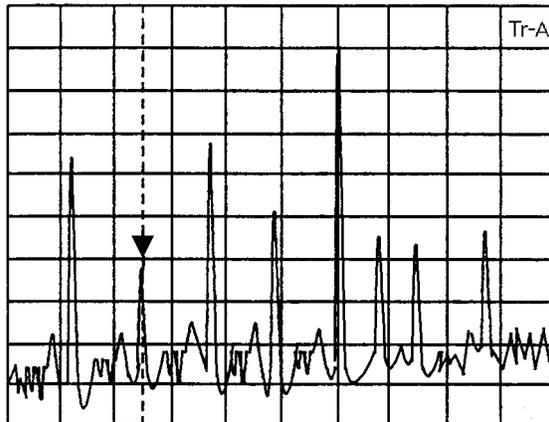
If the zone marker is set to 10 divisions when the zone center frequency is at the center of the frequency axis on the screen, the current marker will always move to the maximum peak level over the entire range of the observation frequency.
