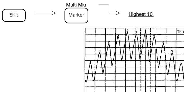
After executing Highest 10, an active marker (with the same functions as the current marker) moves to the peak point of the maximum level signal.
