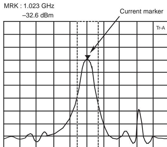
The normal marker displays the absolute level. By setting a display line, the normal marker can also display the level relative to a given level specified as a reference line.
