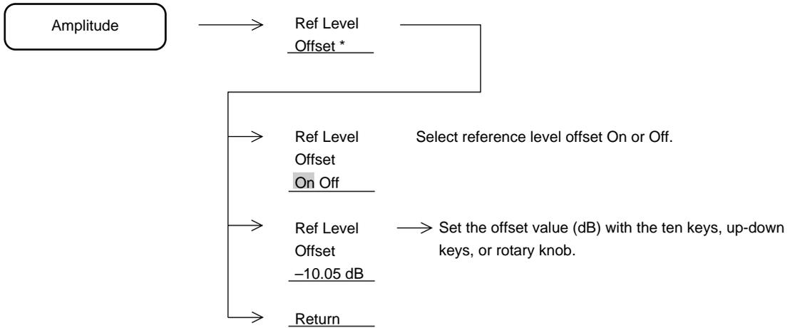
The offset value setting range is from -100 to +100 dB. The offset value resolution is 0.01 dB.
