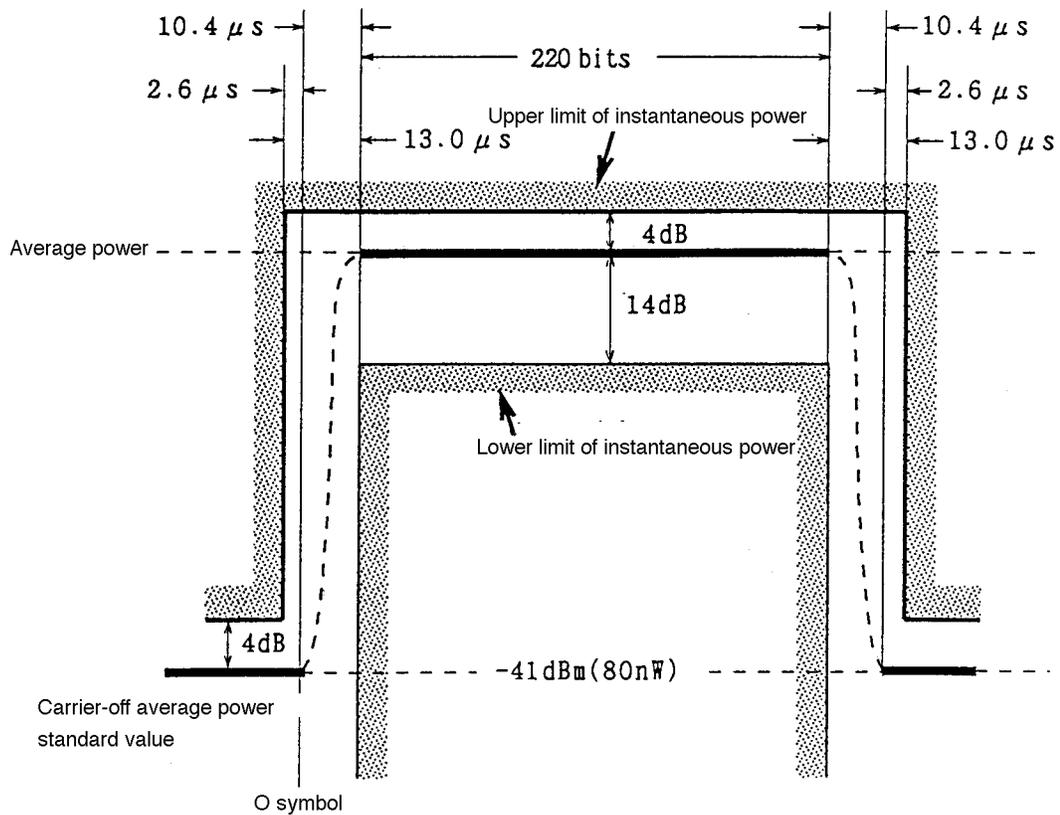
Coordinate reference line (Trigger position → left end of screen:  $-200 \mu\text{s}$ )
