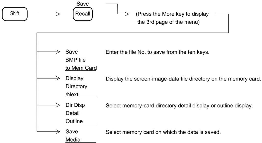
After deleting the menu and data input in this saving mode, only the screen-image-data is saved. Use the memory card which is formatted by the spectrum analyzer.
