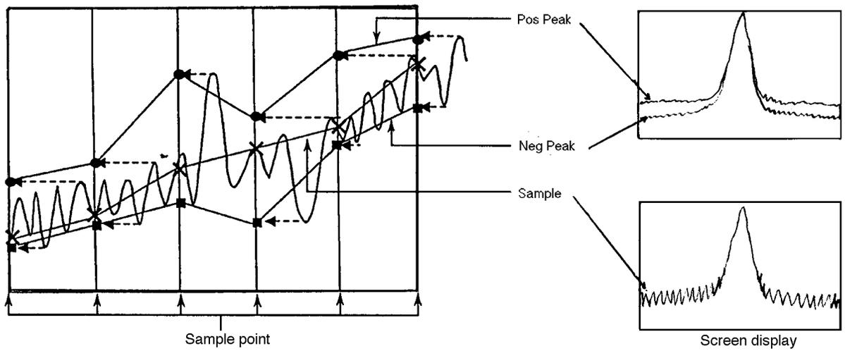
Note: When the detection mode is set to Sample or Neg Peak while the frequency span and resolution bandwidth are set so that the spectrum is displayed as discrete vertical lines, the spectrum peak is incorrectly displayed.
