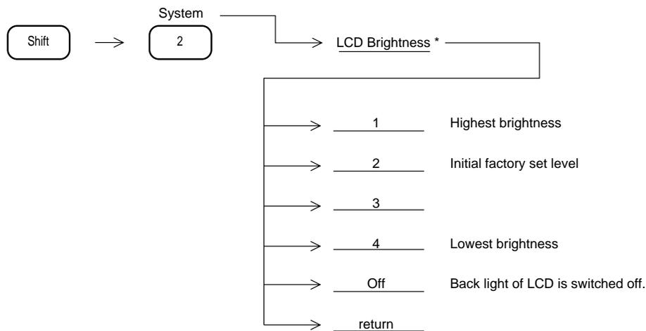
*Note:* LCD type display have a particular range of angle for comfortable viewing depending on the level of brightness of the display.
