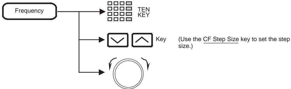
*Note:* Center frequency setting resolution is  $(1 \times N)$  Hz in frequency domain, and in case of zero span mode of MS2665C, is  $(100 \times N)$  Hz, respectively.
