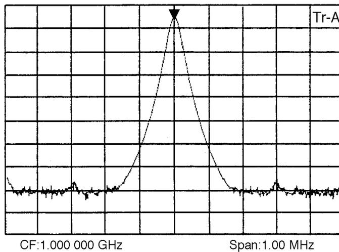
*Note:* In case of MS2665C, when frequency span is 200kHz or less, warming up might be necessary until the observation frequency becomes stable after turning on the power. When "Warm Up" message is being indicated at the top right corner of the indicator, please wait for approximately 3 minutes, and start the measurements after the message disappears.
