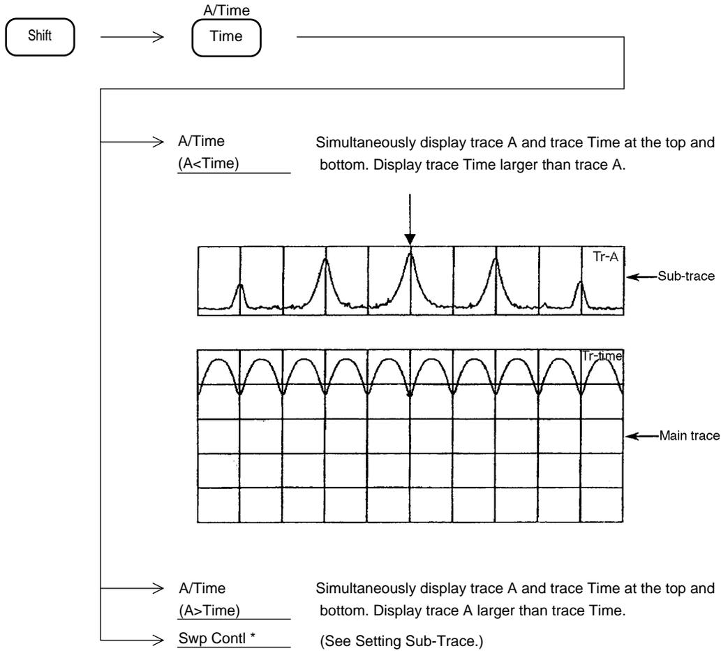
Each parameter can be set in the main trace (larger displayed trace). However, for common parameters (center frequency, reference level, input attenuator, and when system setting is coupled mode resolution bandwidth, video bandwidth, etc.), the sub-trace parameters can also be changed even when setting is performed at the main trace. Marker operation is only available for the main trace.
