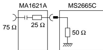
If the equipment is MS2667C/68C, recommend using the optional coaxial adaptor 34AKNF50 (K-P•N-J) when MA1621A impedance transformer is used.
