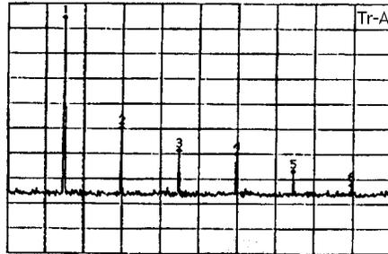
**Note:** If the fundamental and second harmonic signals are not separated by more than the marker zone width, or when there are larger level signals other than harmonic signals in the frequency range of the marker zone width centered at the harmonic signals, harmonic signals will be incorrectly detected. In this case, narrow the marker zone width.
