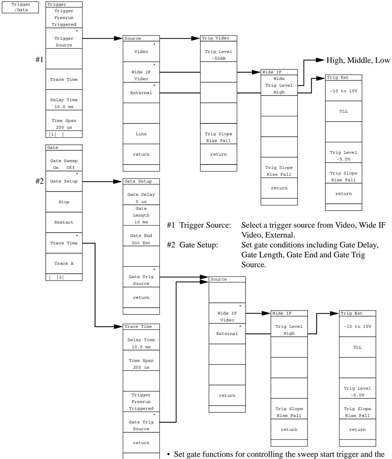
**#1 Trigger Source:** Select a trigger source from Video, Wide IF Video, External.
