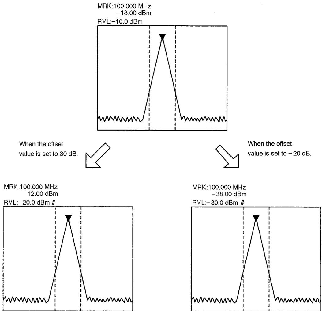
The # is displayed to the right of the reference level display above the scale.
