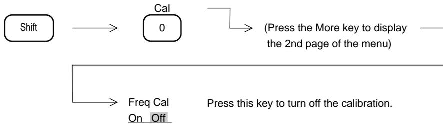
When Freq Cal turned Off, the displayed waveform moves by the error amount.
