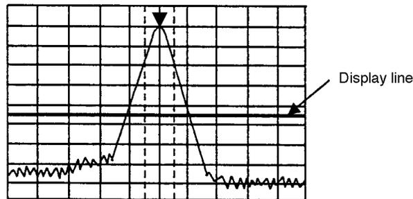
Display-line On and Off are common to all traces (A, B, BG, Time). Also, the display-line level is common except for FM demodulated waveform display.
