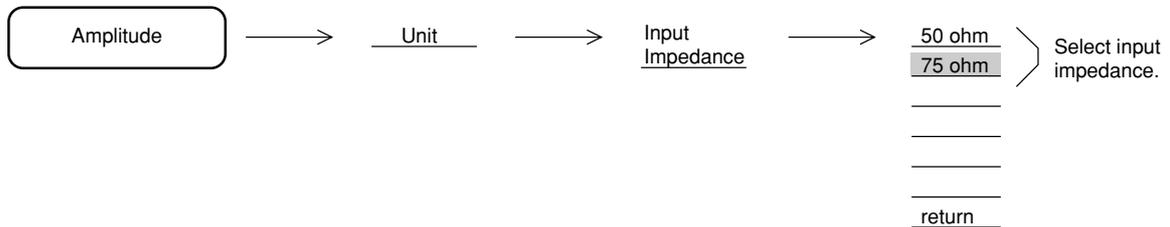
When the input impedance is set to 75 $\Omega$ , "75 ohm" is displayed at the top right of the waveform.
