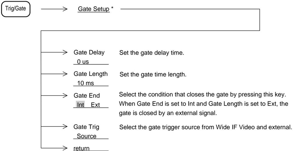
The time domain mode facilitates setting the gate control signal time. The following shows an example of how to use the Time Gate function that uses the time domain mode.
