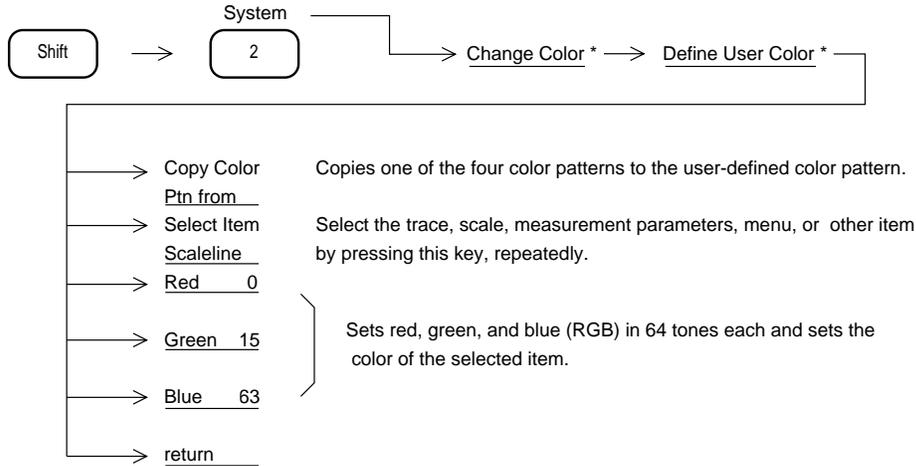
*Note:* *Marker, PTAScreen, Menufield, Menutext, EntryArea, Background, Scalefield, Scaleline, 2ndTrace, 1stTrace, Parameter, Displayline, Trigger, Zone, Temp/Mask, and MultiMarker can be selected.*
