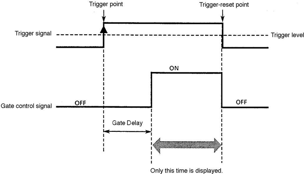
To turn the gate time analysis function On and Off and to create the gate control signal, perform the following key operations.
