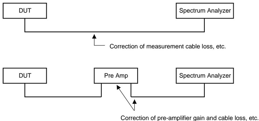
The correction factors for these measurement systems can be stored in the internal memory to add the factor to the measured value and display the spectrum.
