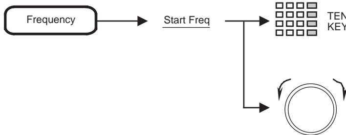
*Note:* Start frequency setting resolution is  $(1 \times N)$  Hz in frequency domain, and in case of zero span mode of MS2665C, is  $(100 \times N)$  Hz, respectively.
