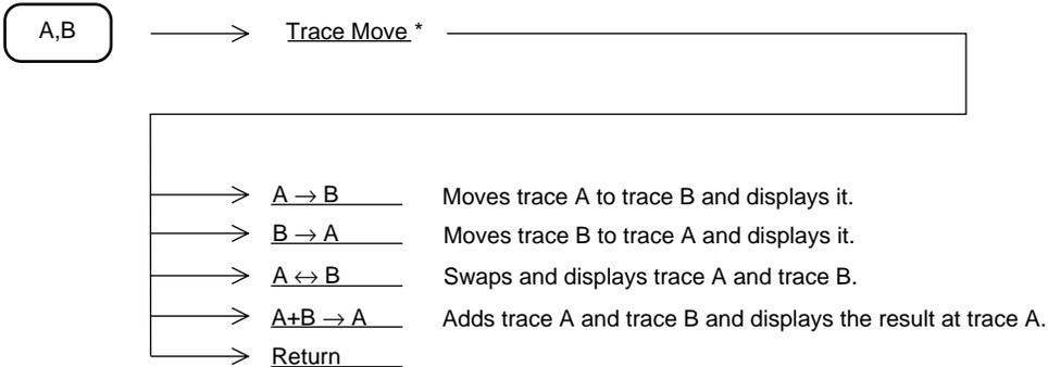
Set the move-destination-trace storage mode to View, and stop the sweeping before moving the trace. If the trace A or trace B threshold is set to any other mode, the trace data will be displayed once, then updated.
