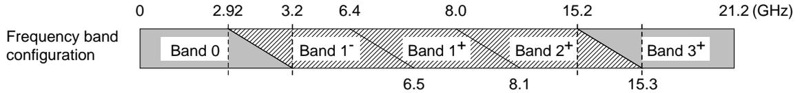
Selection of frequency bands according to range of frequencies to be observed in Auto Band mode
