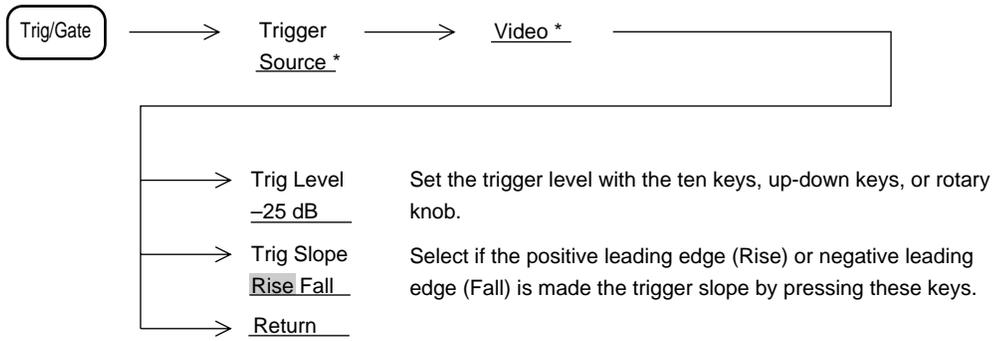
The trigger level is indicated by displaying the trigger level indicator ► at the leftmost vertical line of the screen.
