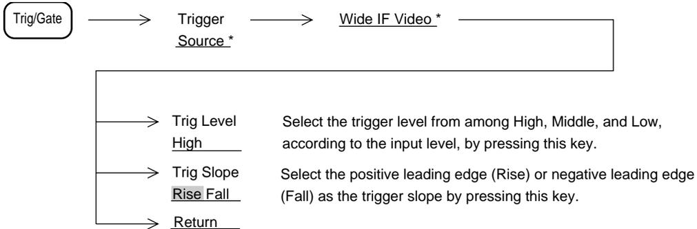
An indicator of appropriate trigger levels for Wide IF Video is listed below.
