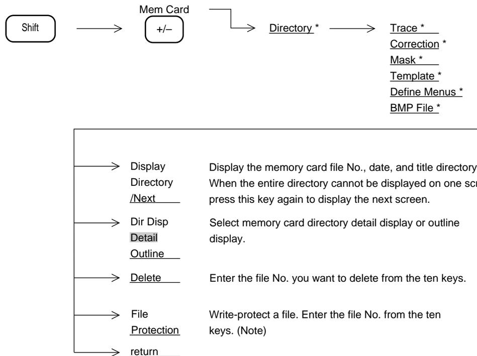
**Note:** The operation above releases write protection of the protected file. Write-protected files are displayed with "protect" in the memory card directory displayed set to "on" and cannot be saved or deleted. Note that the formatting deletes the protected file.
