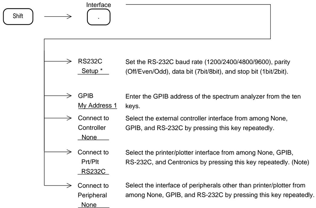
Note: When GPIB is selected as the external controller, for Prt/Plt, select from None and RS-232C.
