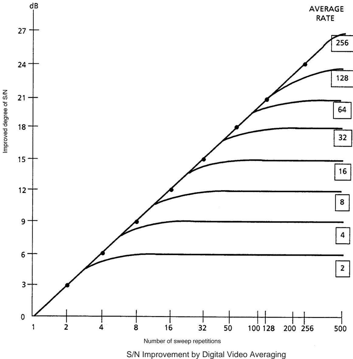
Averaging by video filter has the disadvantage that the sweep time becomes longer when the video bandwidth is narrowed to improve the averaging effect.
