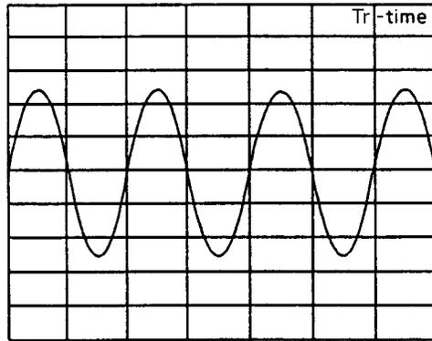
By using the FM demodulated waveform monitor function, frequency deviation can be easily measured.
