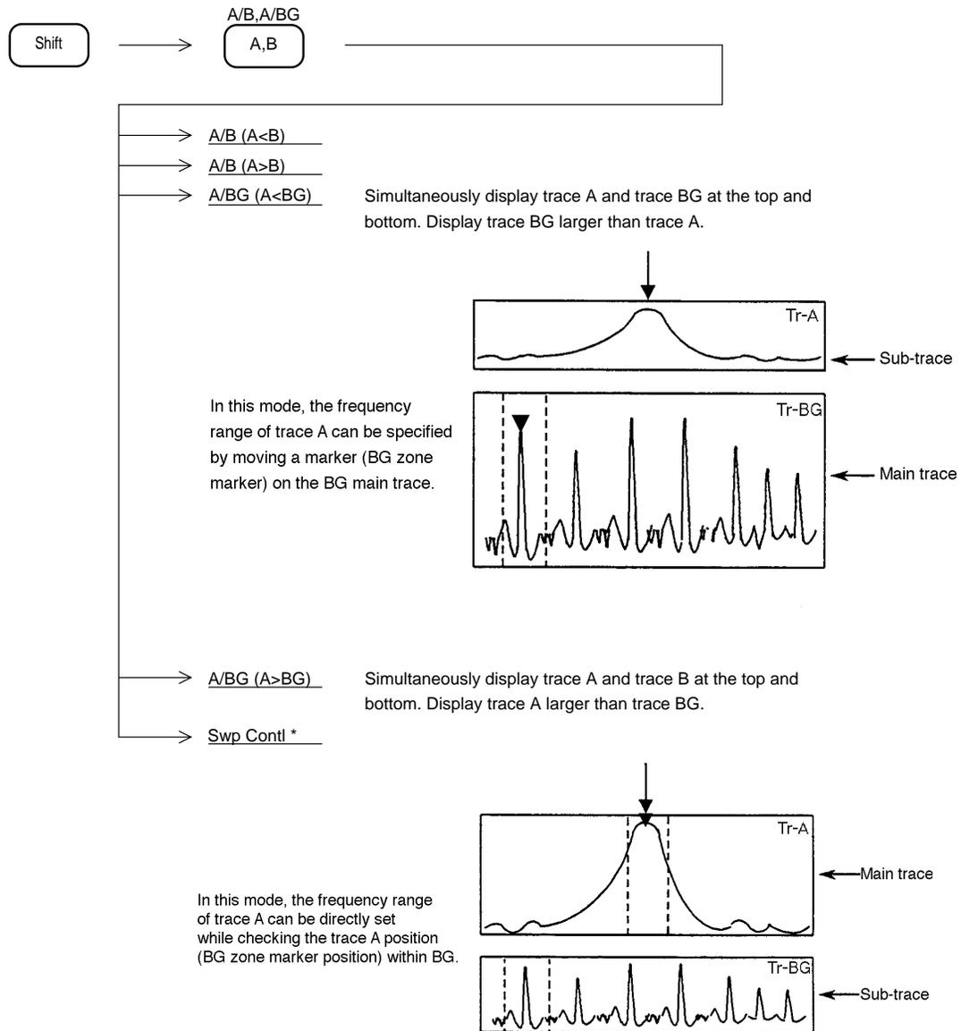
Trace A and trace BG parameters other than reference level, vertical axis scale, and input attenuator settings are used independently. Each parameter can be set in the main trace (larger displayed side).
