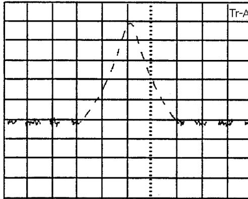
Notes: [1] The detector output is delayed compared to the positive leading edge of the input waveform when the resolution bandwidth (RBW) is narrowed in the frequency domain measurement mode. As a result, spike-like noises may appear on the trace. To prevent this from appearing, set Gate Delay and Gate Length to values that satisfy the following conditions.
