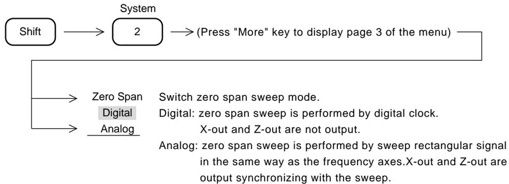
*Note:* When switching the zero span sweep mode to "Analog", a sweep duration is limited to 20ms or more. Even if Option 04 high speed time domain sweep, is mounted, the duration cannot be set at less than 20ms.
