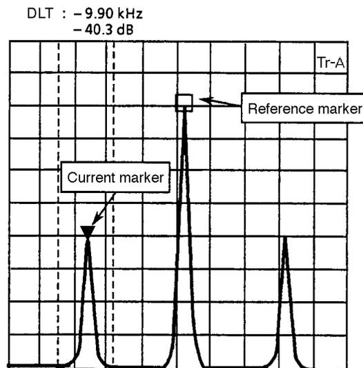
Press the Delta Marker key in the delta maker mode. The reference marker moves to the current marker position and switches to the delta marker mode with that point as the reference point.
