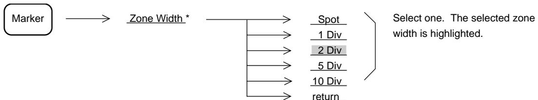
The zone marker width can be arbitrarily set from 1 point to 10 divisions by rotary knob. The zone marker width can be arbitrarily set from 1 point to 10 divisions by the corresponding frequency input from the ten keys.
