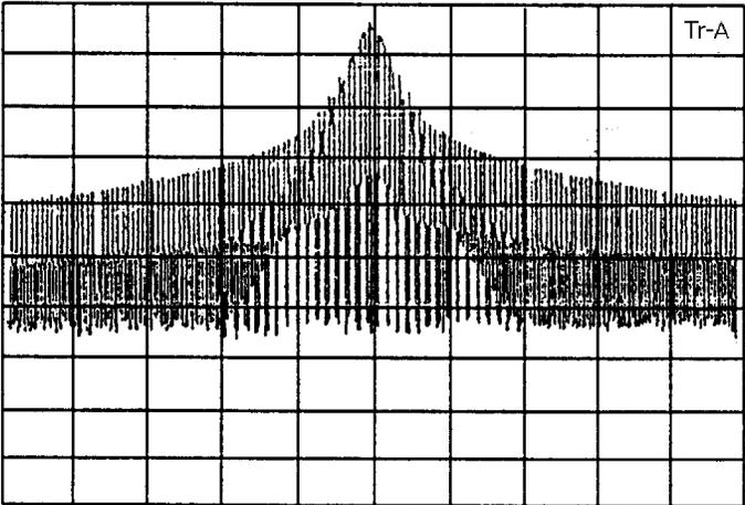
The spectrum spread by the positive leading edge or negative leading edge of the burst wave prevents the spectrum from being observed with the burst set to On.
