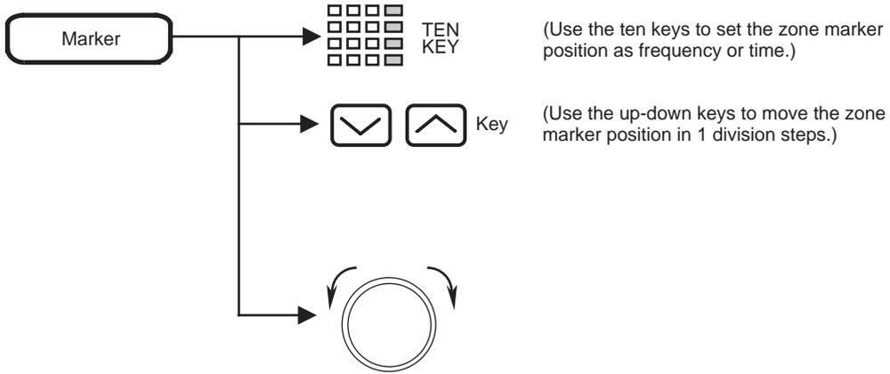
In the delta marker mode, setting the zone marker center frequency (time) with the ten keys results in entry of the delta marker value (difference between reference marker and current marker).
