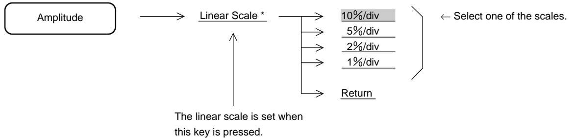
The reference level remains constant, independent of switching between log and linear scales.
