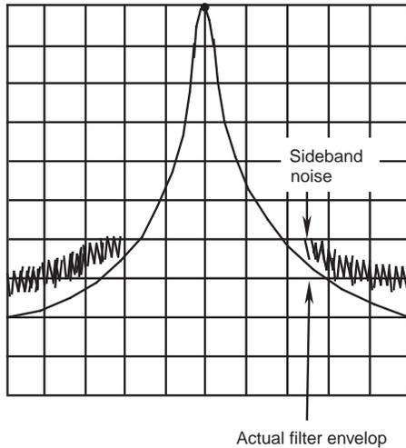
Since the average value is measured for noise level, use a video filter for measurement.
