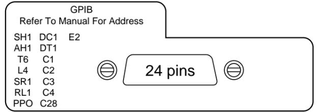
Fig. A-2 MS2665C Rear Panel Layout
