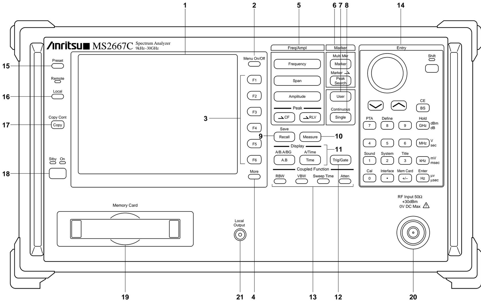
Fig. 3-1 Front Panel
