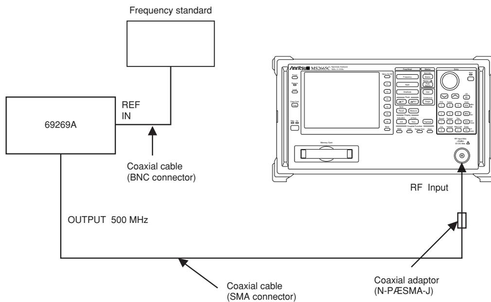
**Frequency Measurement Accuracy Test**
