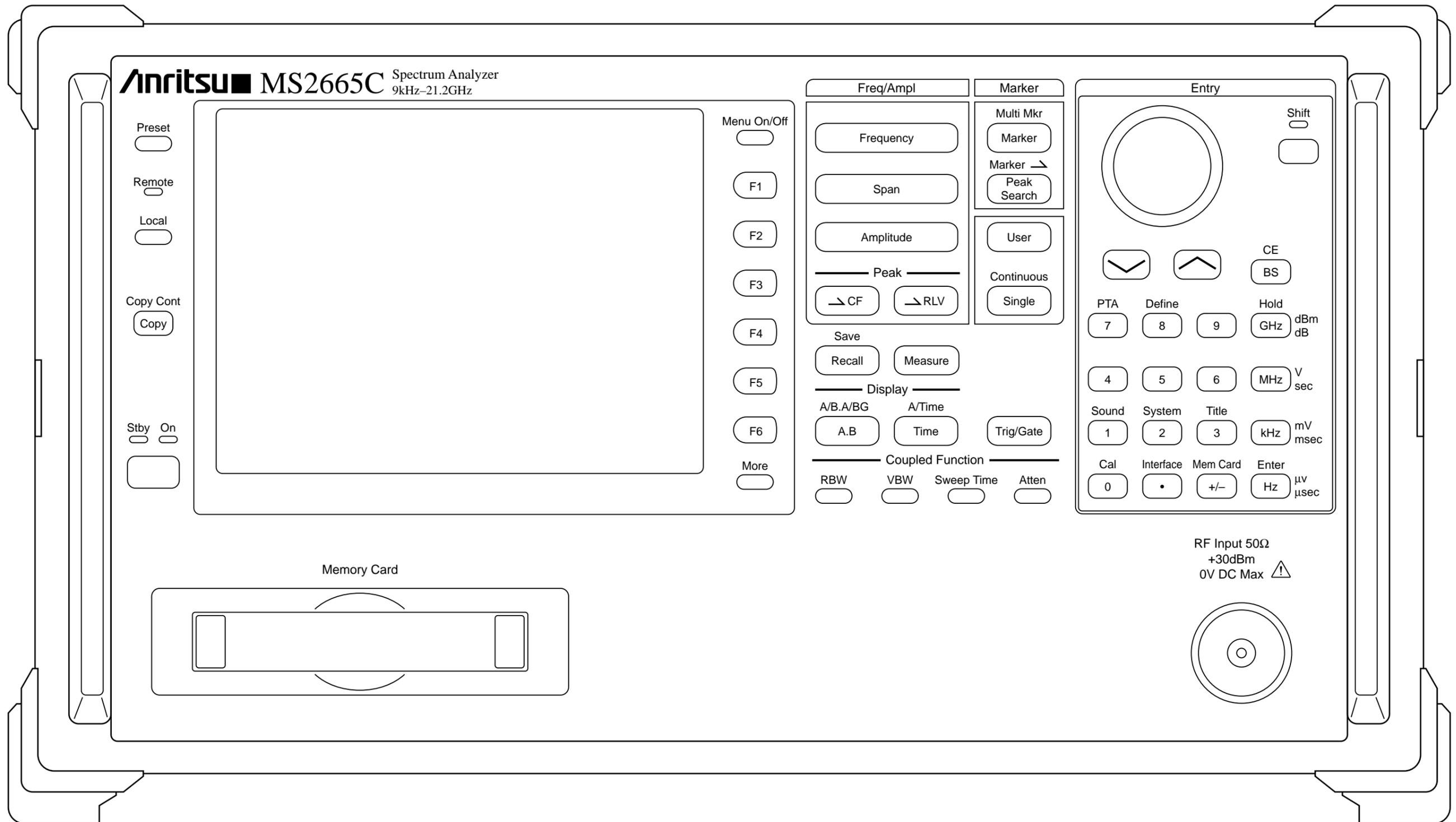
Fig. A-1 MS2665C Front Panel Layout
