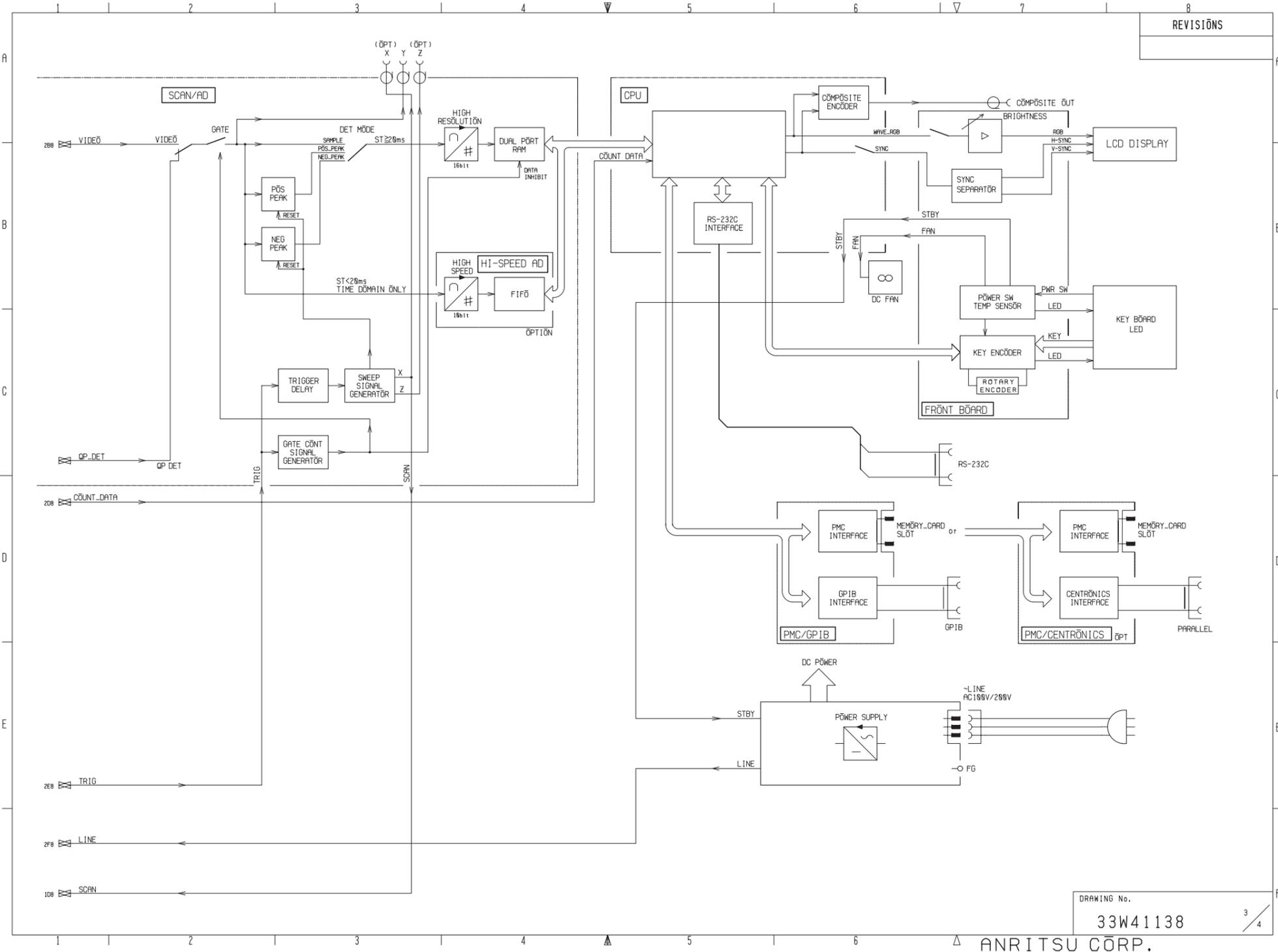
Fig. B-3 MS2665C Block Diagram (3/4)
