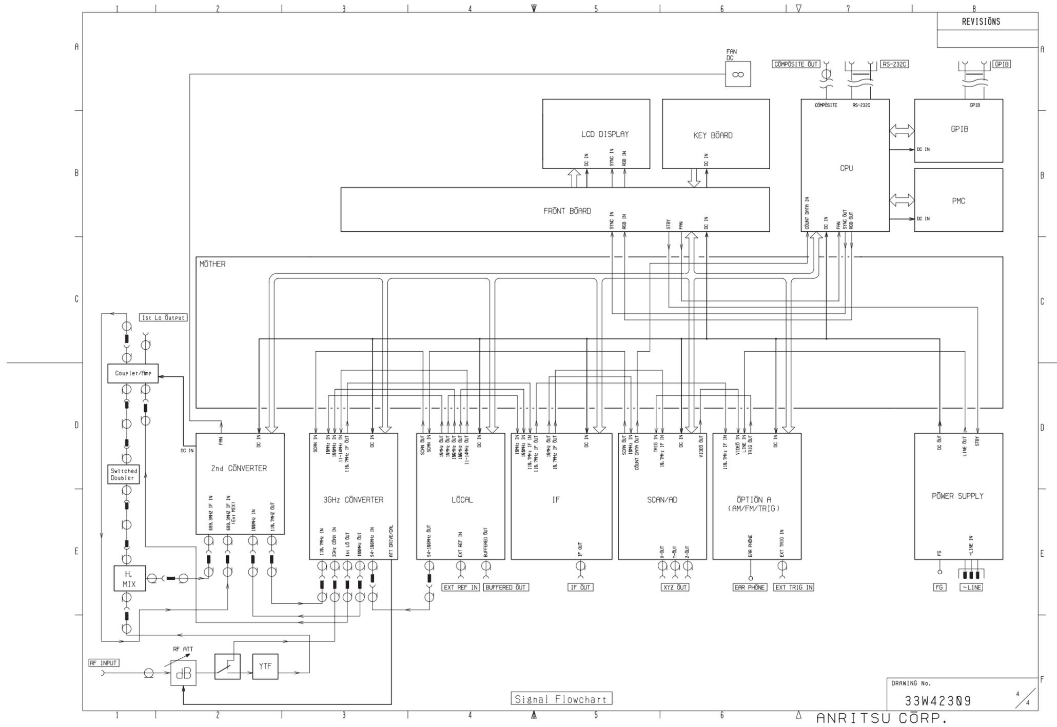
Fig. B-12 MS2668C Block Diagram (4/4)
