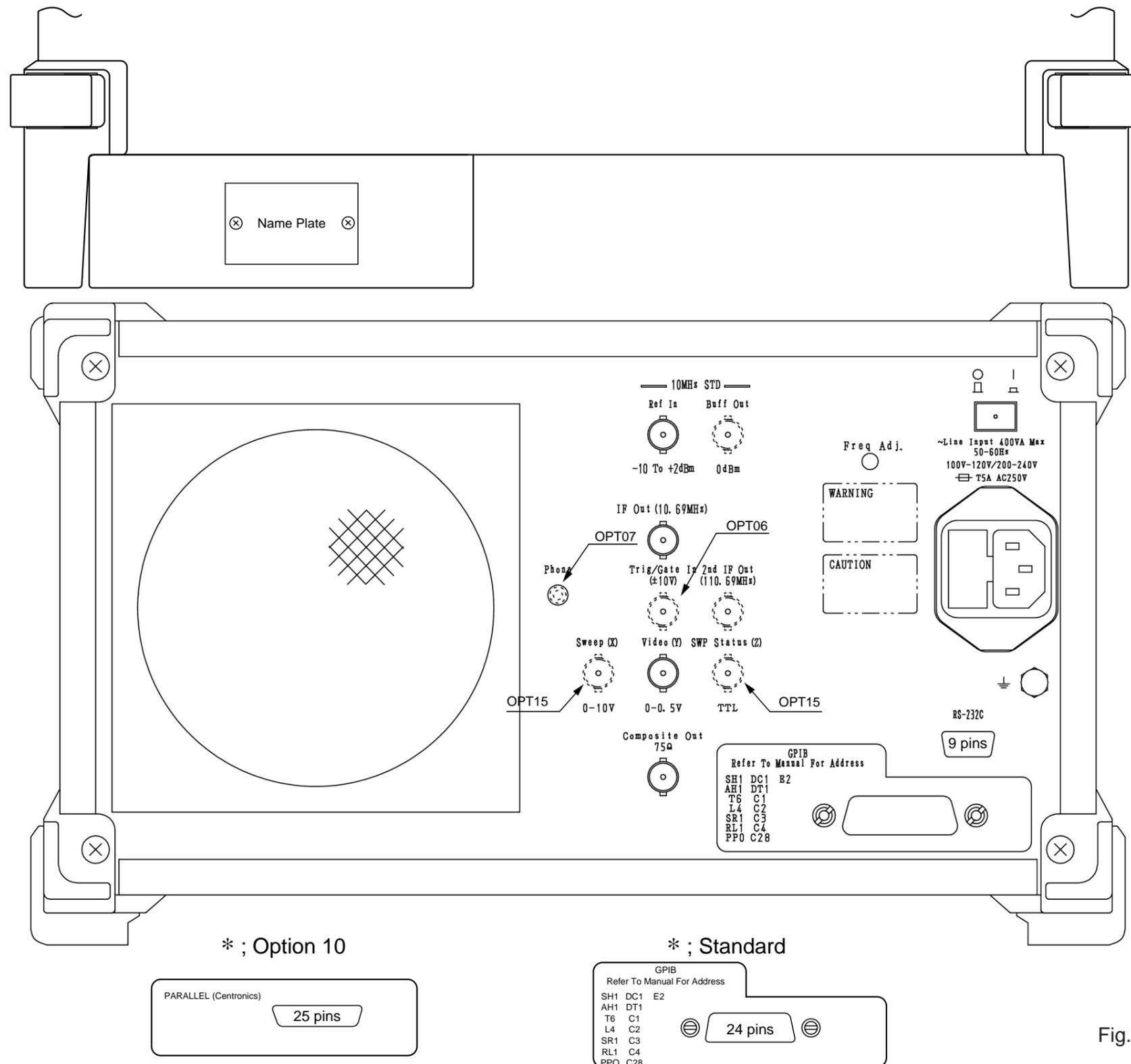
Fig. A-7 MS2668C Rear Panel Layout
