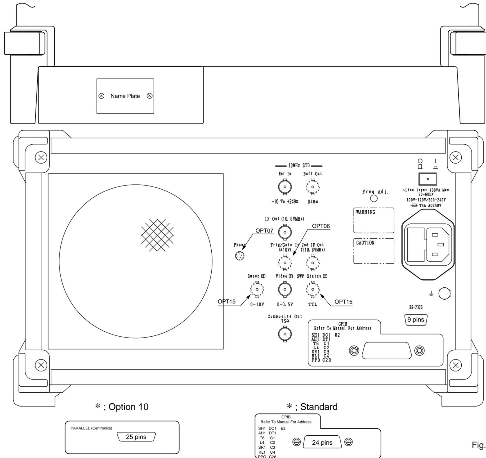
Fig. A-5 MS2667C Rear Panel Layout
