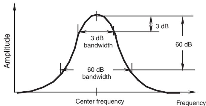
To test the resolution bandwidth and selectivity, first measure the resolution bandwidth (3dB bandwidth), then the 60 dB bandwidth and calculate the 60 dB/3 dB bandwidth ratio.
