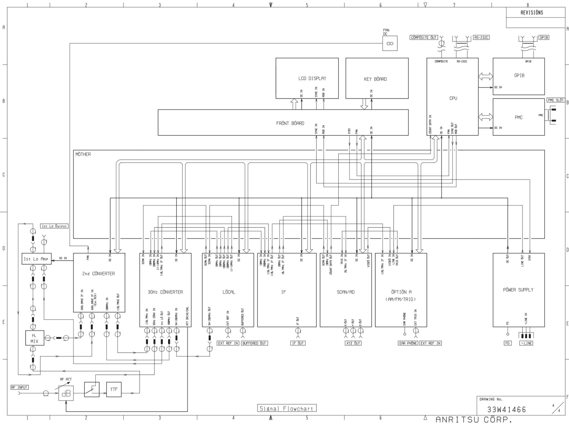
Fig. B-8 MS2667C Block Diagram (4/4)
