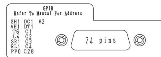
Fig. A-3 MS2665C (with Opt. 14) Rear Panel Layout
