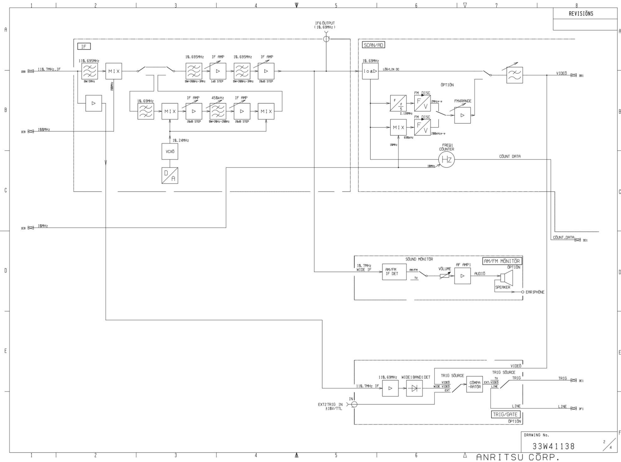
Fig. B-2 MS2665C Block Diagram (2/4)
