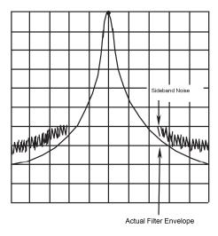
Figure 6.2.3-1 Single sideband noise level
