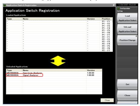
Figure 3.5.1-1 Application Switch Registration screen
