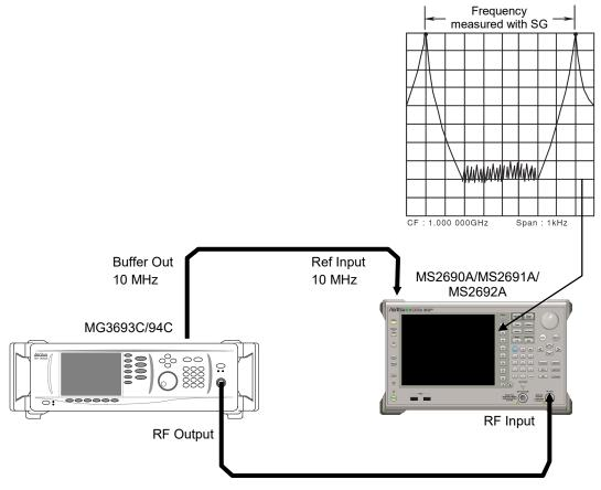
Figure 6.2.2-1 Frequency span display accuracy test
