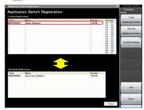
Figure 3.5.2-1 Application Switch Registration screen
