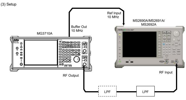
Figure 6.2.6-1 Second harmonic wave distortion test
