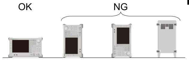
Figure 2.2.1-1 Installation orientation
