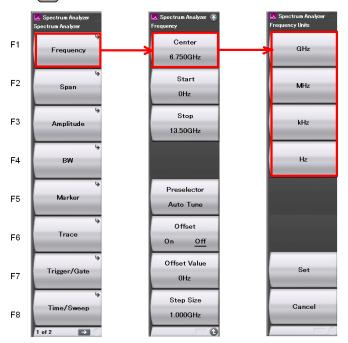
Figure 4.2.1-4 Spectrum analyzer main function menu
