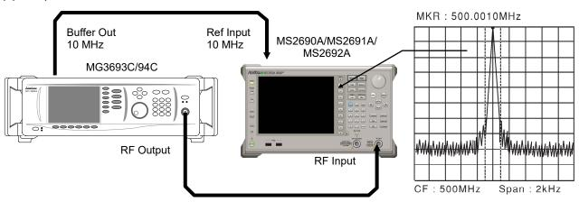
Figure 6.2.1-1 Display frequency accuracy test
