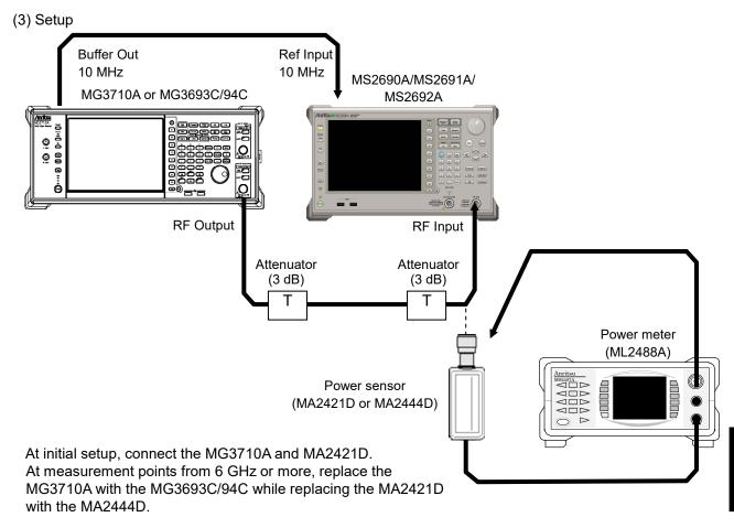
Figure 6.2.4-1 RF frequency characteristics test
